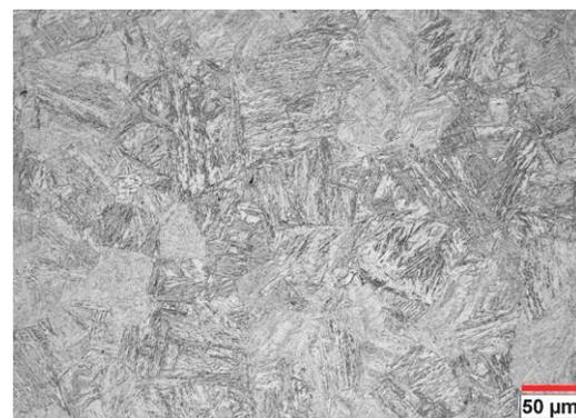
**Figure 5.12: Optical microstructure for L06C06NbMo at different cooling rates**
