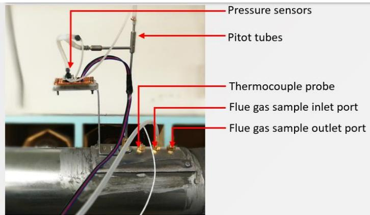
**Figure B-3: Sensors installed in a flue gas duct**
