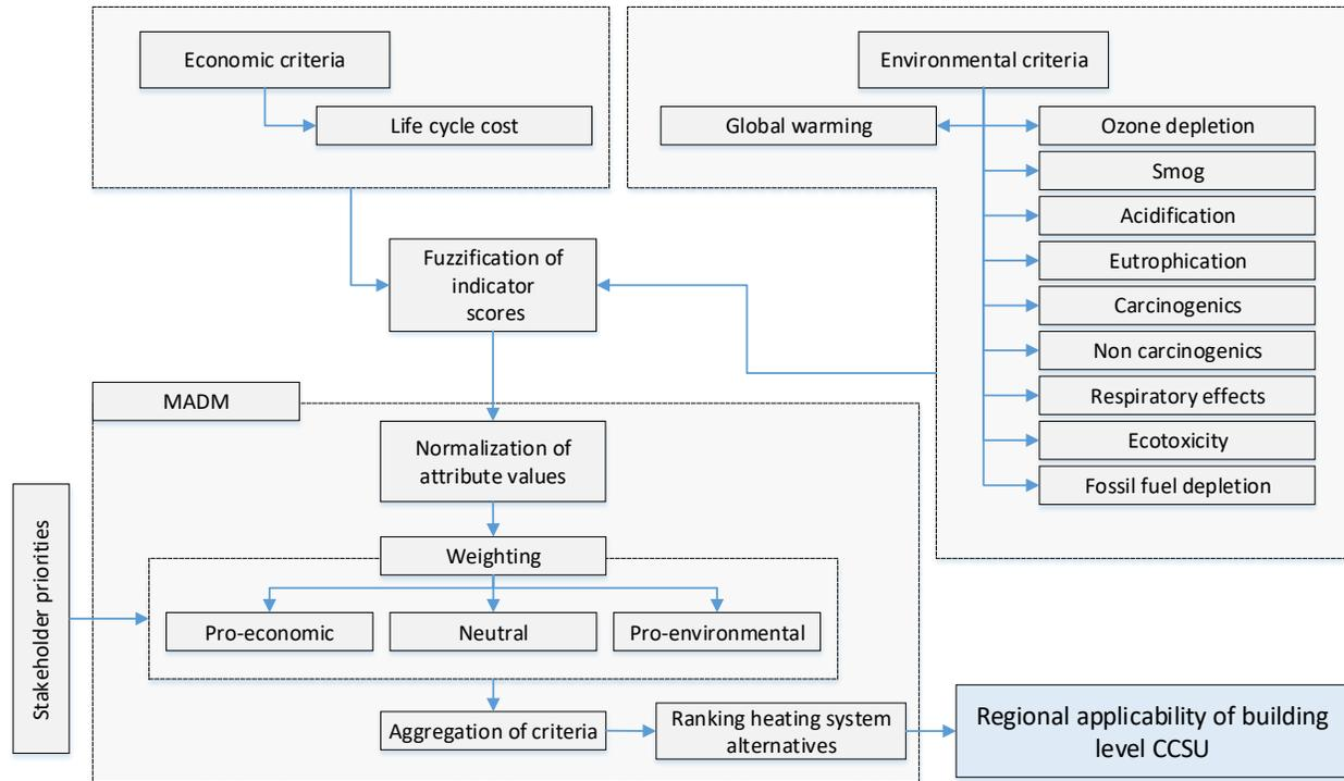
**Figure 6-1: Comparative performance assessment model for building heating systems integrated with carbon capturing**
