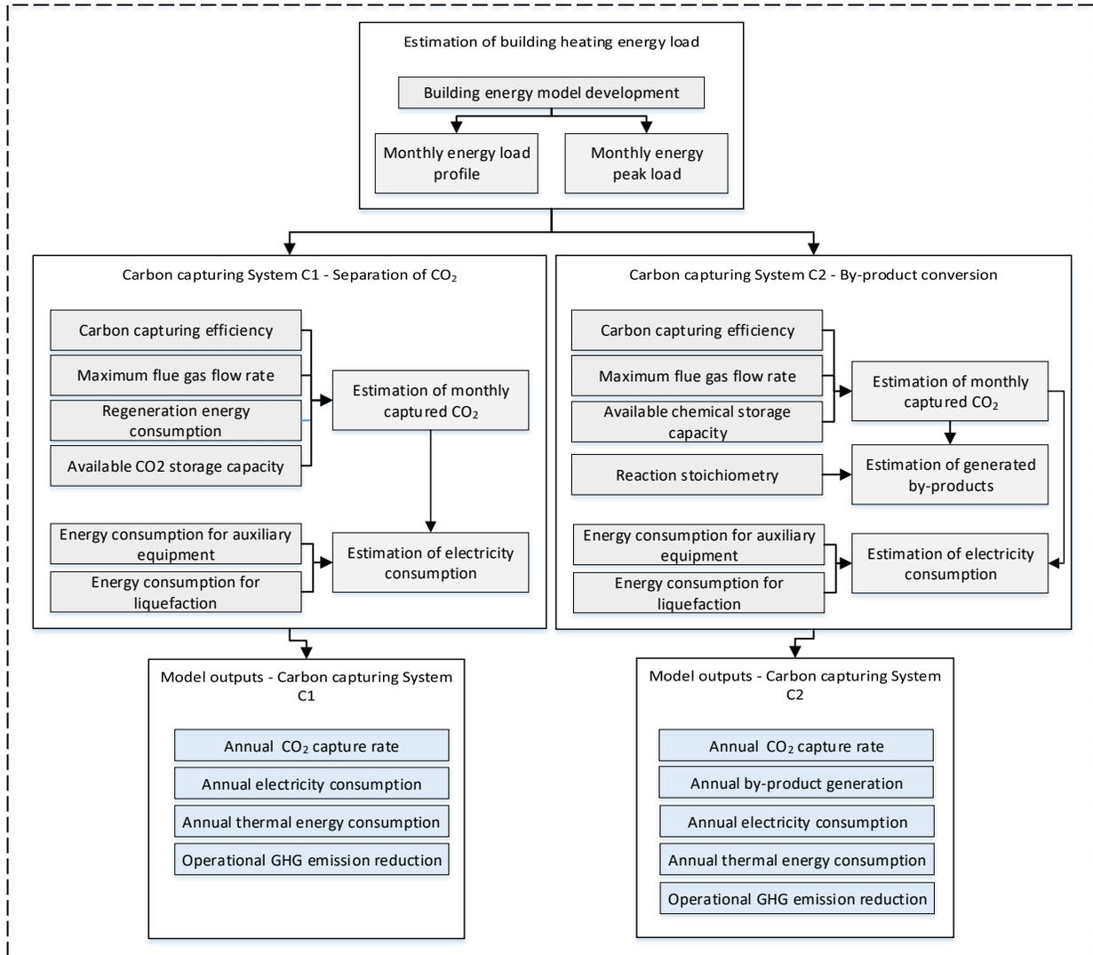
**Figure 4-3: Operational characteristics estimation model**
