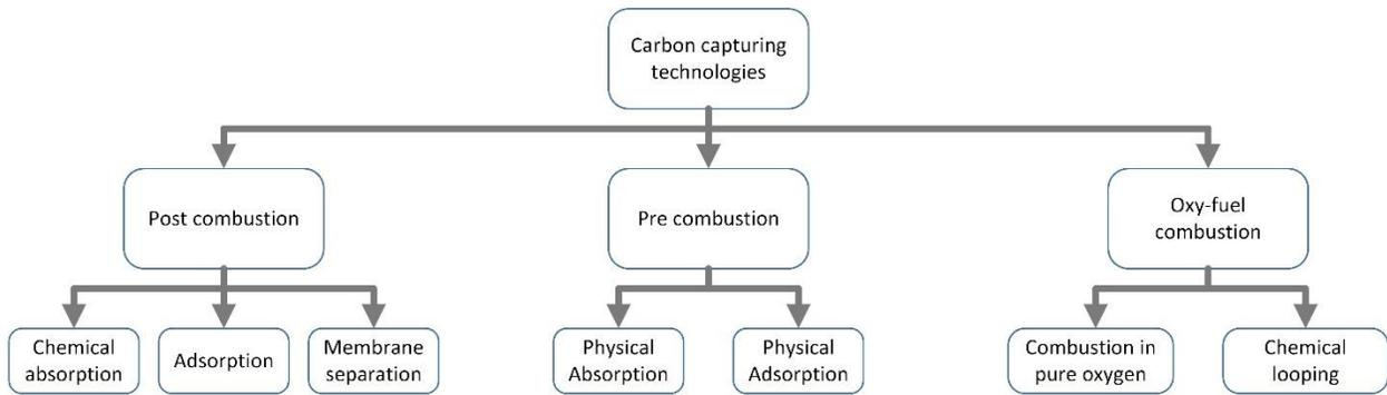
**Figure 3-2: Classification of carbon capturing technologies**
