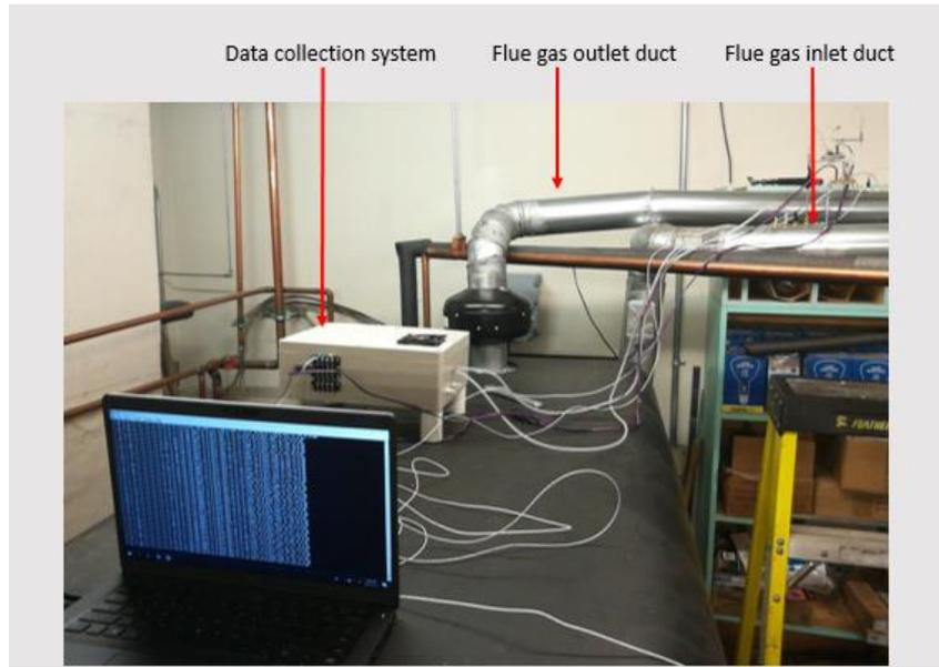
**Figure B-5: Completed instrumentation setup**
