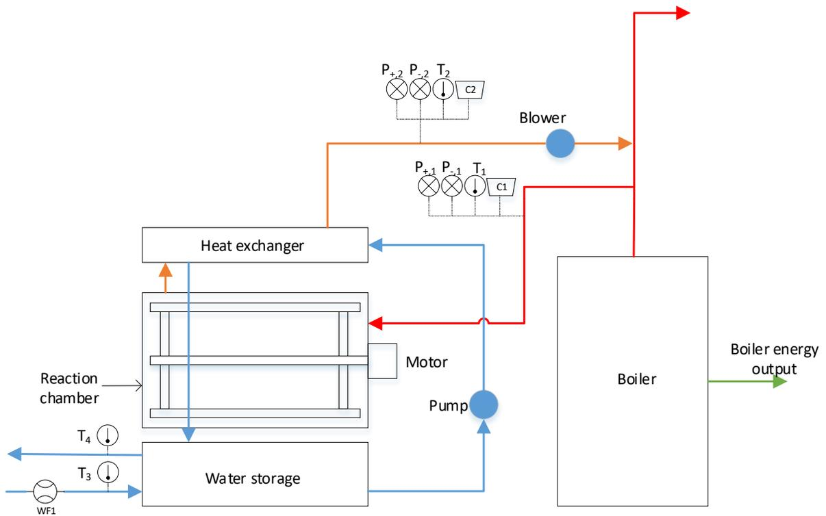
**Figure B-1: Instrumentation diagram**
