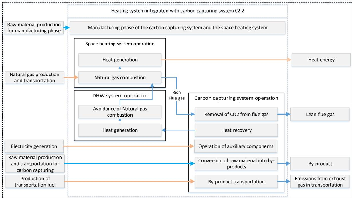
**Figure 5-4: The system boundary used in Scenario C2.2**
