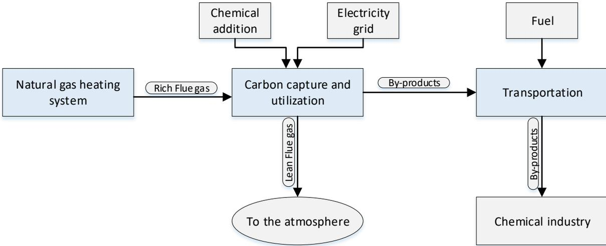
**Figure 4-2: The carbon capturing process that converts CO<sub>2</sub> into a by-product (Type 2)**
