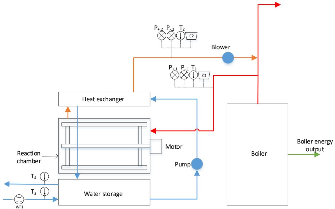
**Figure 4-6: Instrumentation setup of technical performance evaluation**
