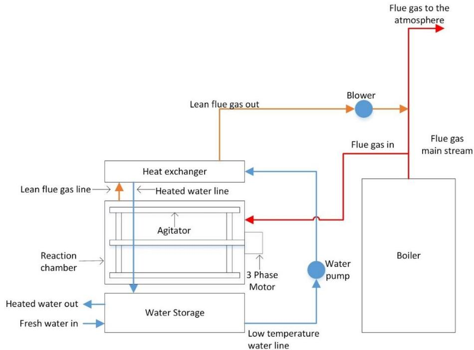
**Figure 4-5: Schematic diagram of KOH-based building-level carbon capturing system**
