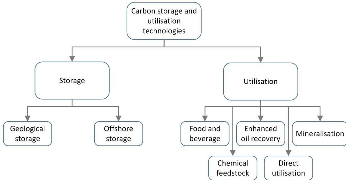
**Figure 3-3: Classification of carbon storage and utilisation methods**
