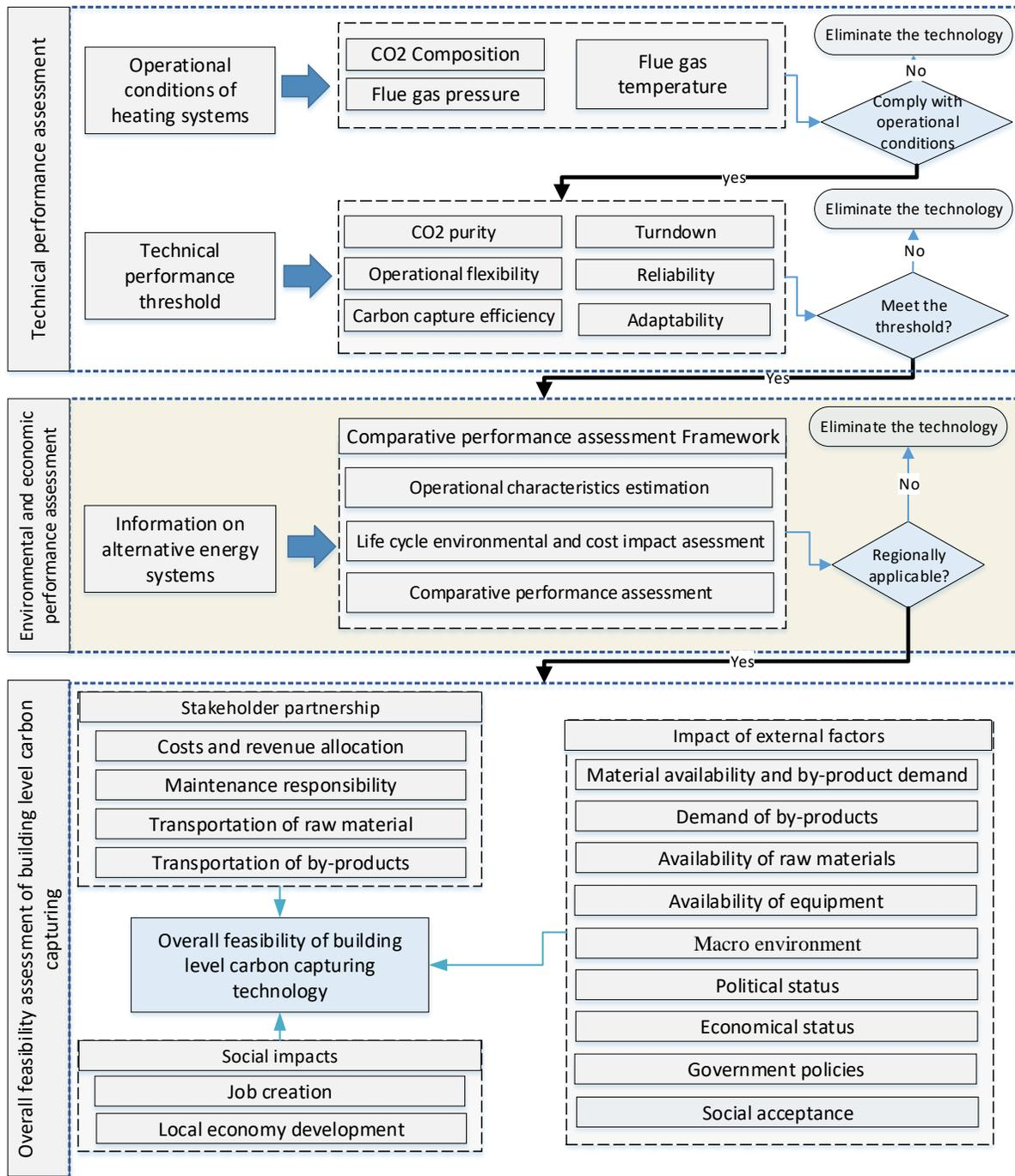
**Figure 7-1: Overall vision of the feasibility assessment of building-level carbon capturing implementation**
