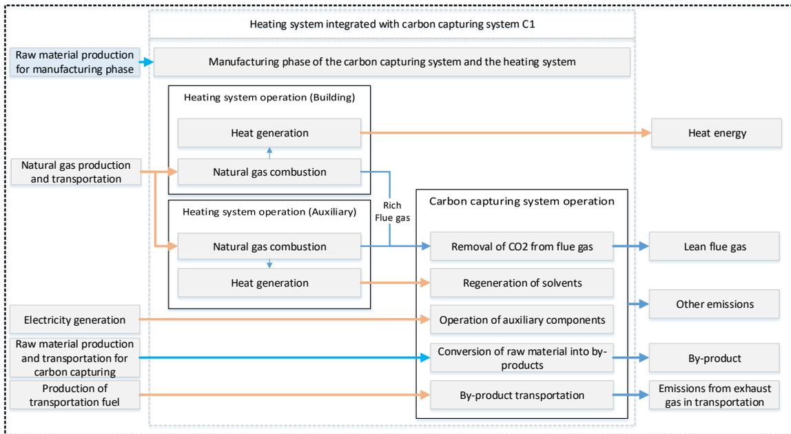
**Figure 5-2: The system boundary used in Scenario C1.1 to Scenario C1.4**
