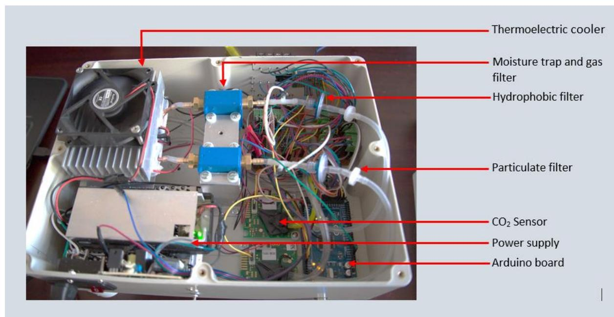
**Figure B-2: Data collection system and components**
