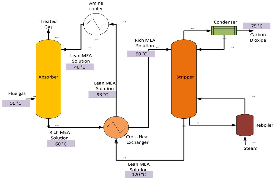
Figure 4-4 Process diagram of the MEA based carbon capturing system
