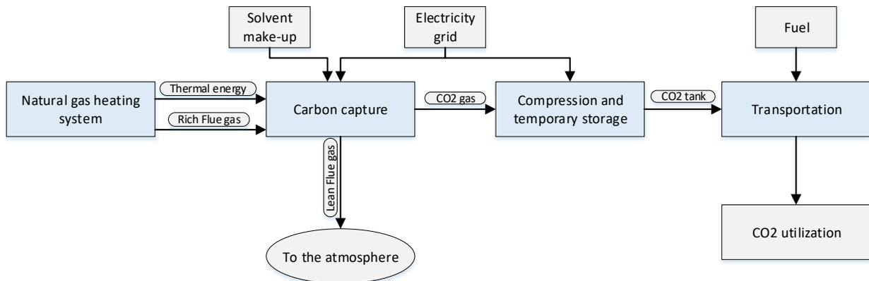
**Figure 4-1: The carbon capturing process that separates CO<sub>2</sub> from flue gas (Type 1)**
