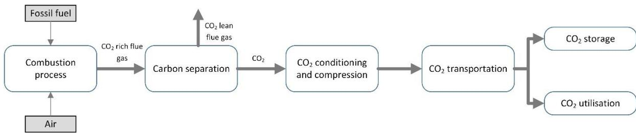
**Figure 3-1: Post-combustion carbon capturing process**
