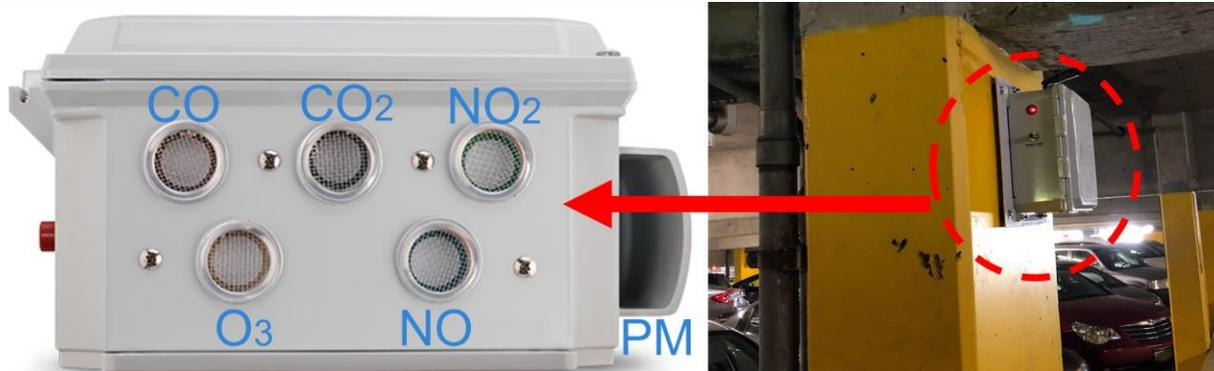
Figure 3.1 RAMP mounted in a parking garage (right) and the bottom of a RAMP monitor showing the location of the sampling units (left).
