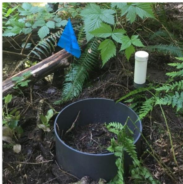
Figure 2.3 Conceptual illustration (left) and photo (right) of static chamber used to measure greenhouse gas exchange in riparian soils.
