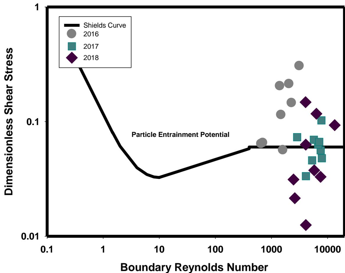
Figure 26. 2016 to 2018 dredged zone calculated dimensionless shear stress and Boundary Reynolds number per cross-section plotted against the critical shear stress for particle entrainment curve at  $2.7 \text{ m}^3\text{s}^{-1}$  discharge.
