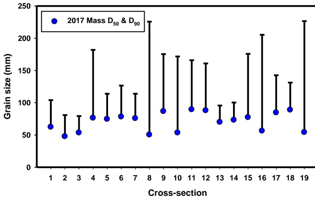
Figure 8. Frequency (a) and mass (b). The 2017  $D_{50}$  and  $D_{90}$  per cross-section using the frequency and mass processing methods. The  $D_{50}$  is represented by the blue marker and the  $D_{90}$  with the upper marker.
