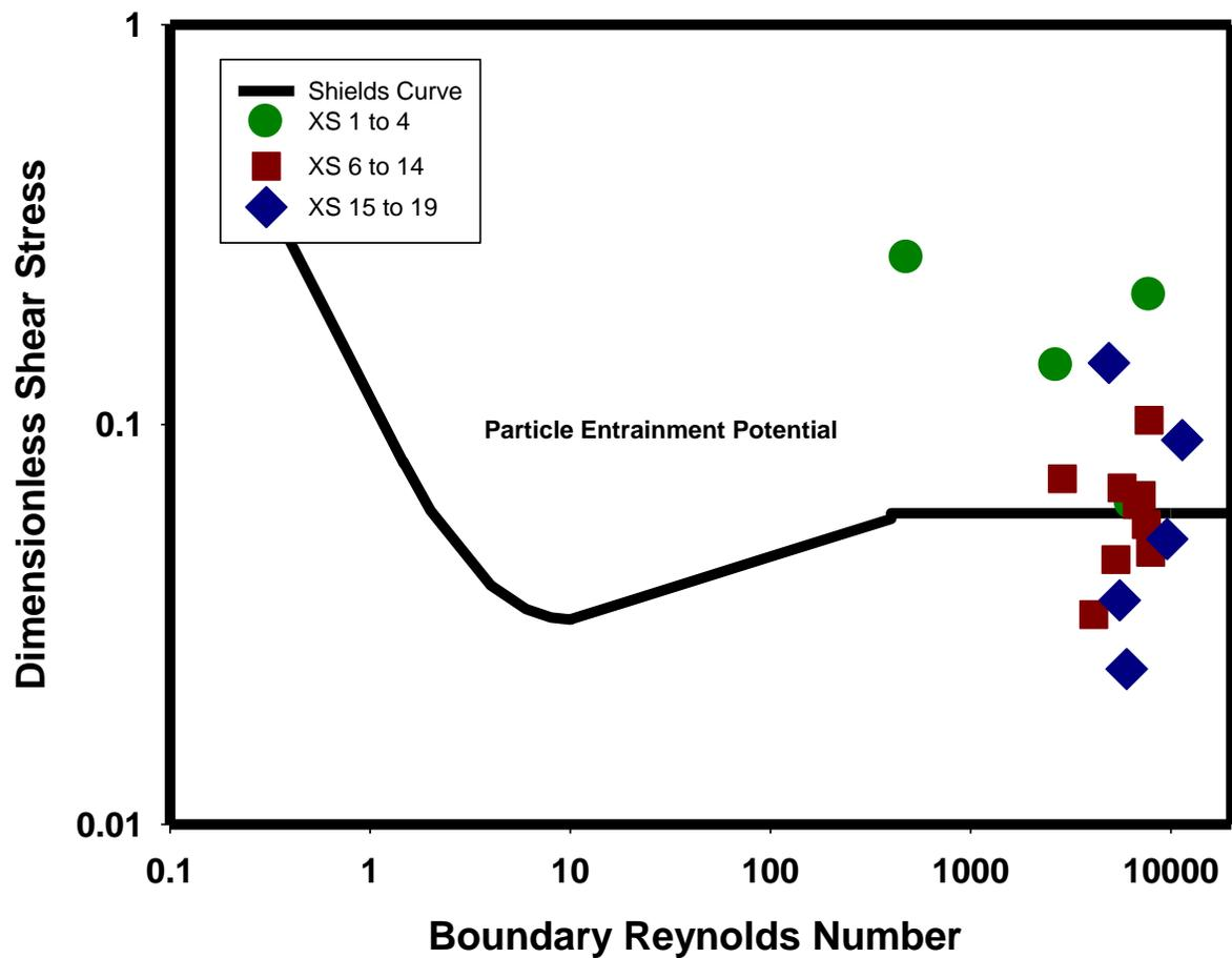
Figure 24. 2017 calculated dimensionless shear stress and Boundary Reynolds number per cross-section plotted against the critical shear stress for particle entrainment curve at  $2.7 \text{ m}^3\text{s}^{-1}$  discharge.
