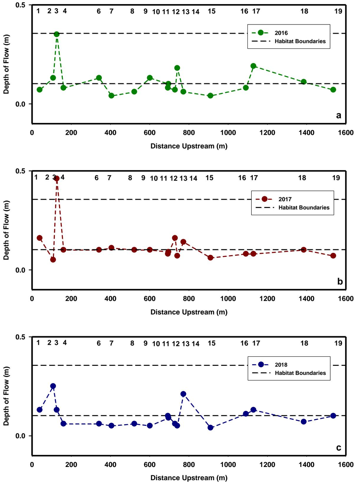
Figure 31. 2016 (a), 2017 (b), and 2018 (c) HEC-RAS  $0.100 \text{ m}^3\text{s}^{-1}$  simulated average depth of flow at each cross-section. The ideal habitat parameters for spawning Coho, 0.10 - 0.36 m (DFG, 2002b; Sandercock, 1991).
