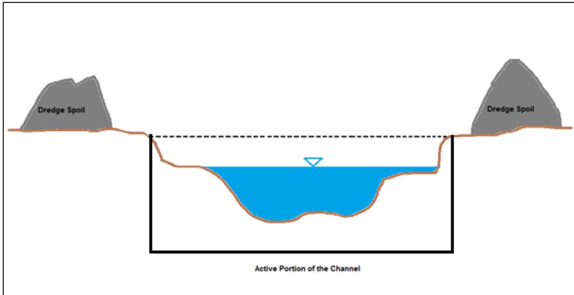
**Figure 7. Typical stream levels (solid blue) and peak flood stage (dashed black line) define of the bankfull width for each cross-section, which is used within WINXSPRO to define the limits of the area calculations. Areas beyond the bankfull stage, such as dredge spoil and levee-top roads were excluded.**
