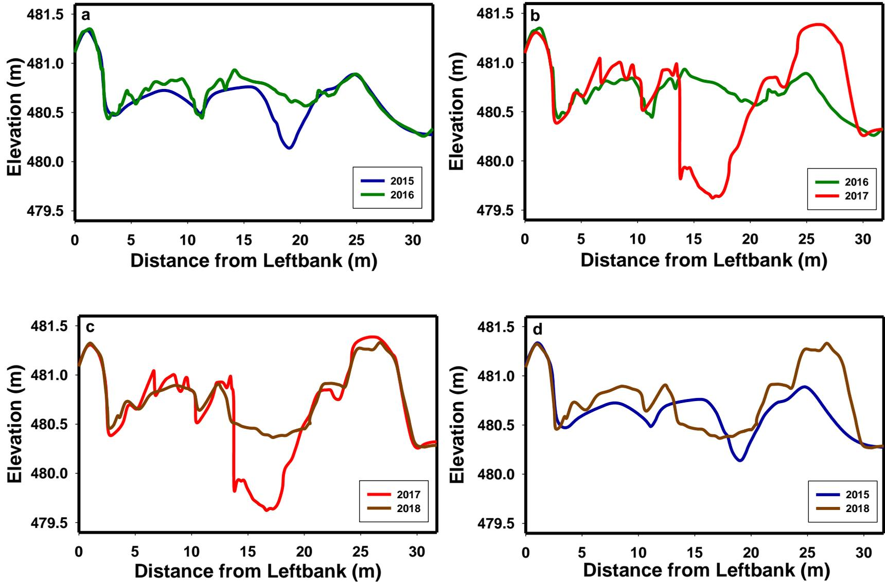
Figure 11. Channel geometry changes at cross-section 8 from 2015 to 2016 (a), 2016 to 2017 (b), 2017 to 2018 (c), and 2015 to 2018 (d).
