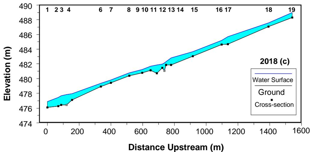
Figure 16. HEC-RAS modelled surface water elevation and minimum channel elevation per cross-section simulated at  $2.7\text{m}^3\text{s}^{-1}$  discharge for 2016 (a), 2017 (b), and 2018 (c).
