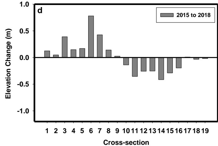
Figure 18. Thalweg elevation change per cross-section 2015 to 2016 (a), 2016 to 2017 (b), 2017 to 2018 (c), and 2015 to 2018 (d).
