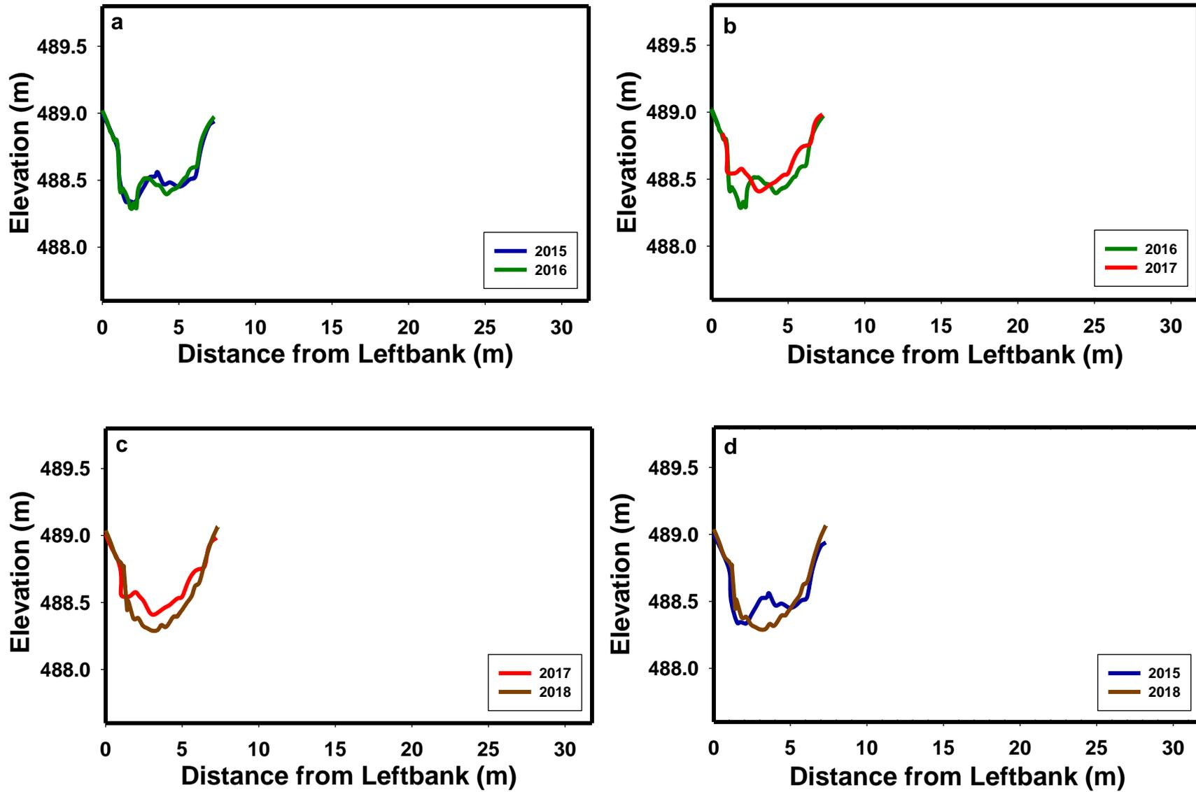
Figure 13. Channel geometry changes at cross-section 19 from 2015 to 2016 (a), 2016 to 2017 (b), 2017 to 2018 (b), and 2015 to 2018 (d).
