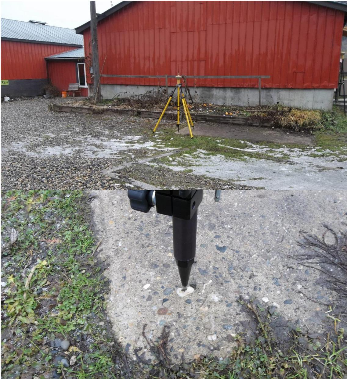
**Photograph 2. The Topcon RTK-DGPS base station set up and the quartz pebble benchmark December 12, 2015 (Photograph: B. Bauer).**
