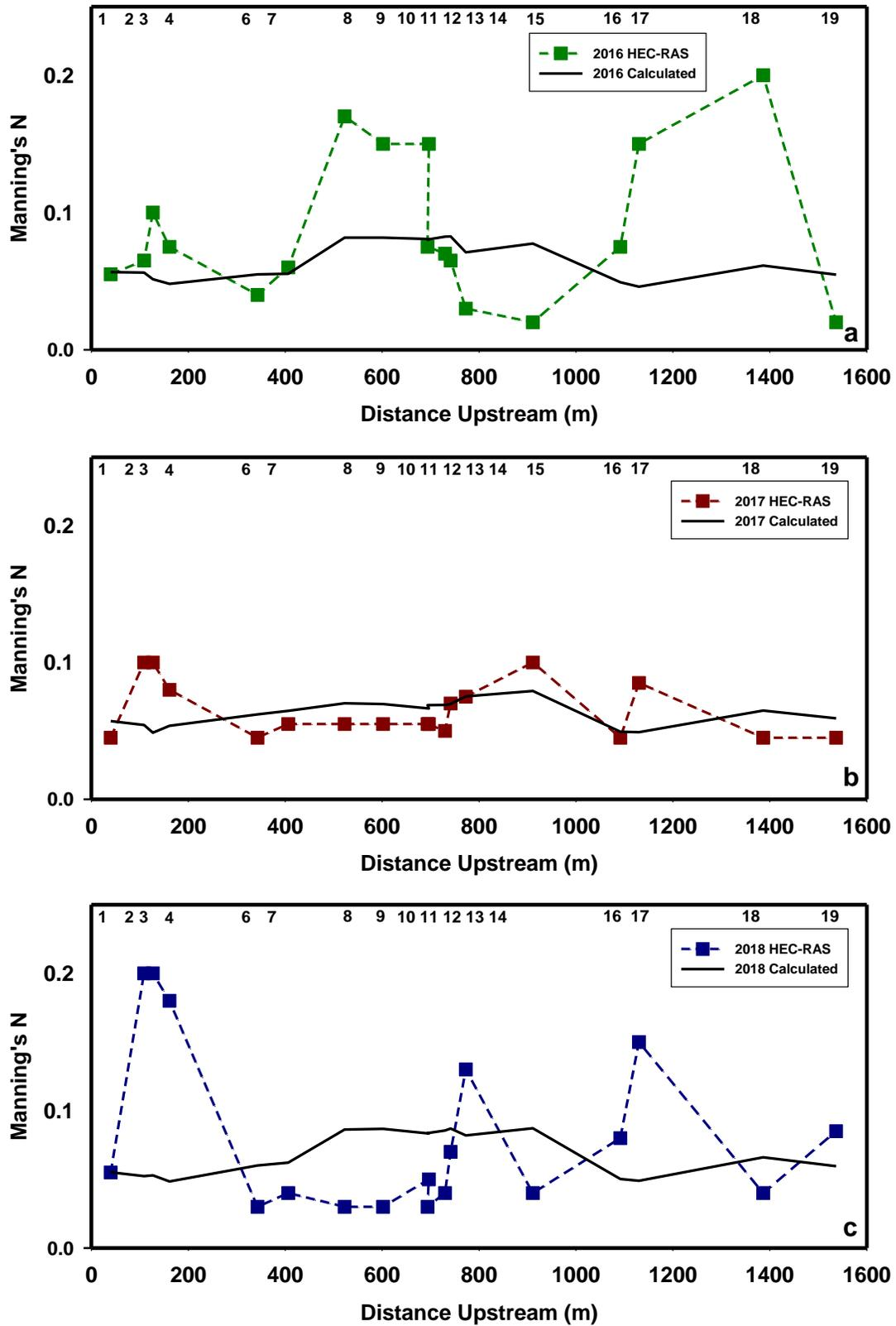
Figure 29. 2016 (a), 2017 (b), and 2018 (c) comparison of the calculated and HEC-RAS modelled Manning's N roughness coefficient per cross-section.
