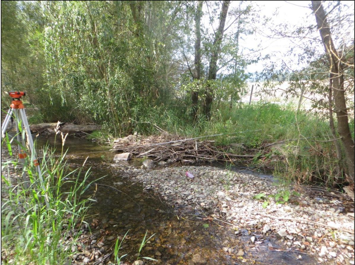
**Photograph 3. Surveying August 30, 2016 using an engineer's level and stadia rod at cross-section 9 (Photograph: L. Hettrich).**
