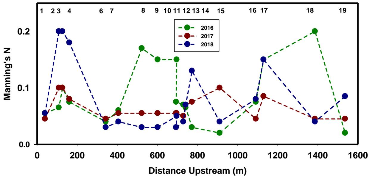
Figure 28. The 2016 to 2018 Manning's N per cross-section used to calibrate the HEC-RAS models.
