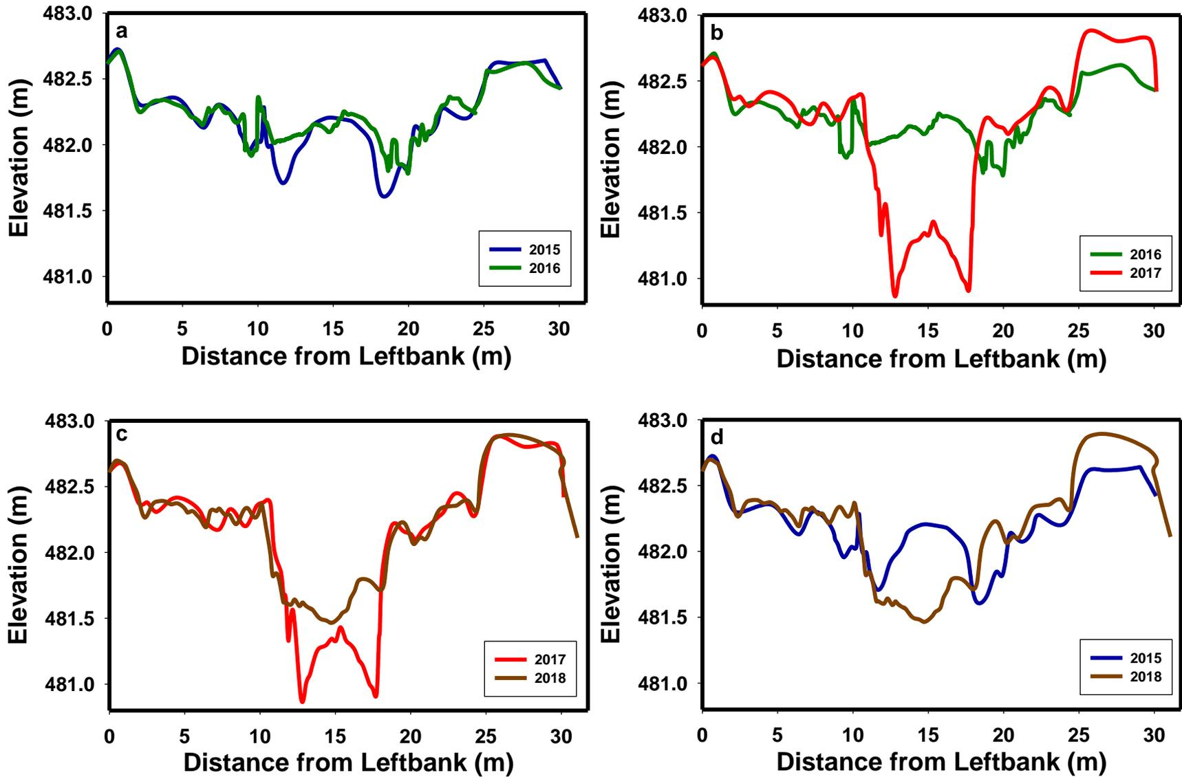
Figure 12. Channel geometry changes at cross-section 12 from 2015 to 2016 (a), 2016 to 2017 (b), 2017 to 2018 (c), and 2015 to 2018 (d).
