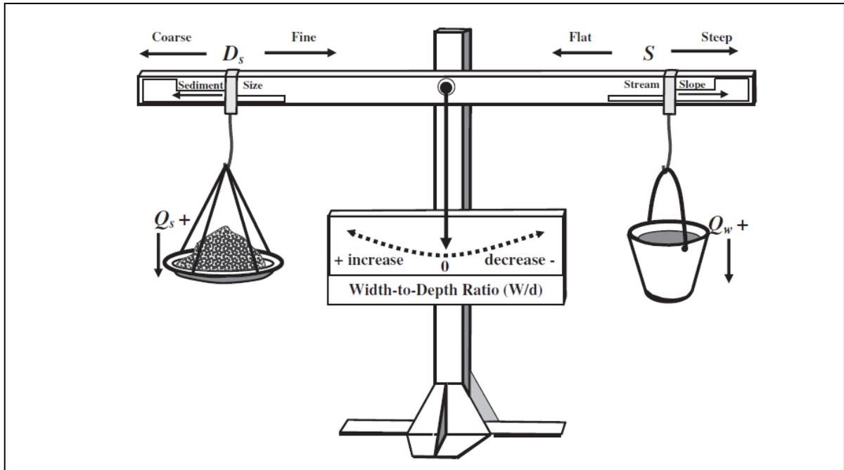
**Figure 5. Depiction of Lane's Balance (1955) representing the balance between sediment size, load, channel slope and discharge adapted from Dust & Wohl (2012).**
