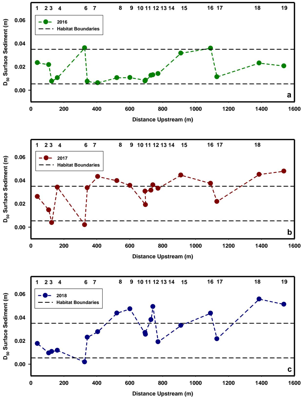
Figure 30. 2016 (a), 2017 (b), and 2018 (c) changes in  $D_{50}$  distribution at each cross-section including habitat parameters. The ideal  $D_{50}$  for spawning Coho is 0.0054 to 0.0350 m (Chambers et al. 1954, Koski 1966, Kondolf & Wolman 1993).
