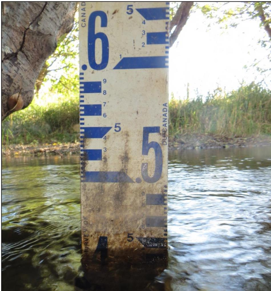
**Photograph 4.** FLNRORD staff gauge located at Creighton Creek, identified as CRE2 (Photograph: L. Hettrich).
