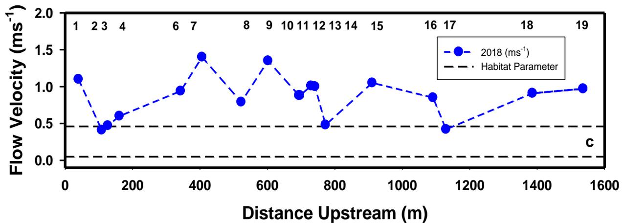
Figure 22. 2016 (a), 2017 (b), and 2018 (c) HEC-RAS 2.7 m<sup>3</sup>s<sup>-1</sup> simulated average flow velocity (ms<sup>-1</sup>) at each cross-section. The dotted lines represent the critical velocity habitat requirements (0.05 - 0.46 ms<sup>-1</sup>) (Bjornn & Reiser, 1991; Moyle, 2002) for juvenile Coho Salmon.
