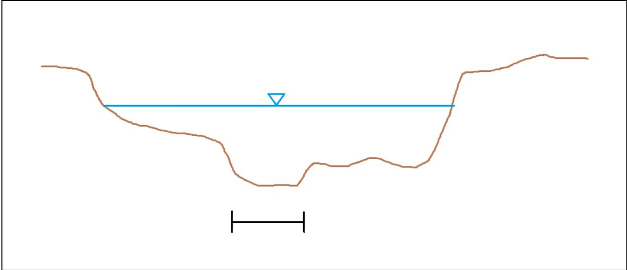
**Figure 6. Illustrates the area within a cross-section where the average of the geo-referenced thalweg survey points were taken to represent the elevation of the cross-section.**
