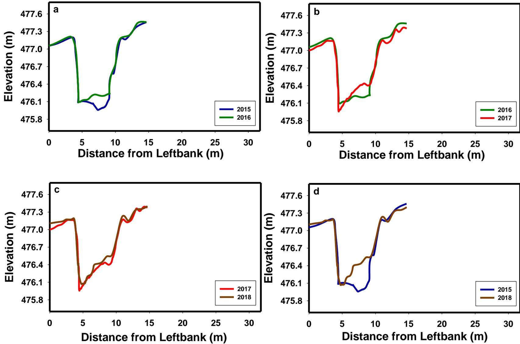
Figure 10. Channel geometry changes at cross-section 1 from 2015 to 2016 (a), 2016 to 2017 (b), 2017 to 2018 (c), and 2015 to 2018 (d).
