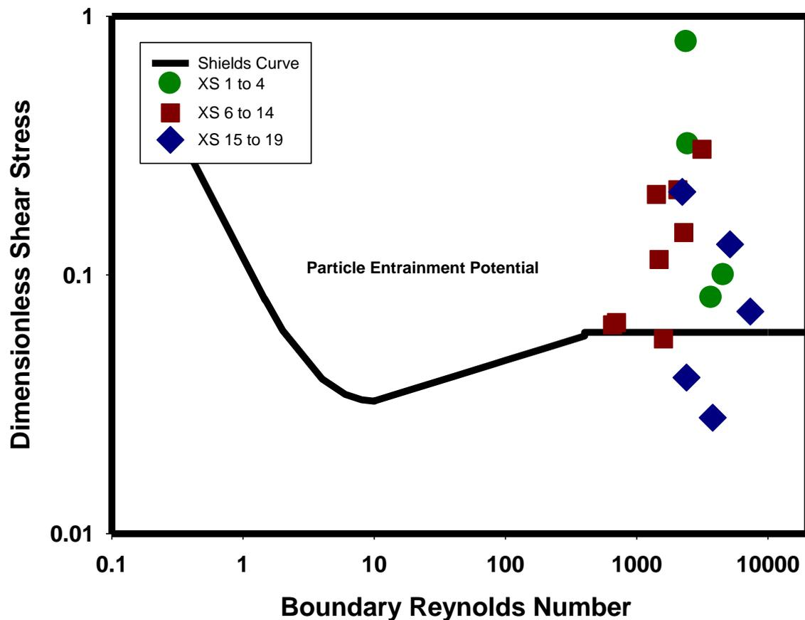
Figure 23. 2016 calculated dimensionless shear stress and Boundary Reynolds number per cross-section plotted against the critical shear stress for particle entrainment curve at  $2.7 \text{ m}^3\text{s}^{-1}$  discharge.
