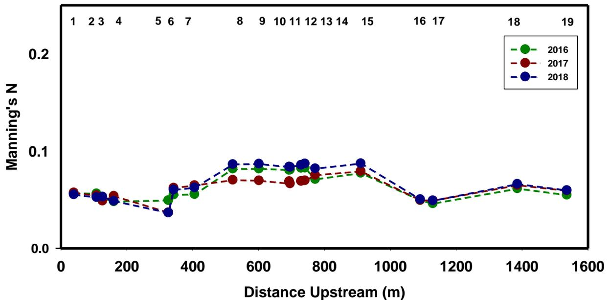
Figure 27. The 2016 to 2018 Stickler equation Manning's N (Stricker 1923) described by Chow 1959, Limerinos 1970 and Arcement & Schneider, 1989.
