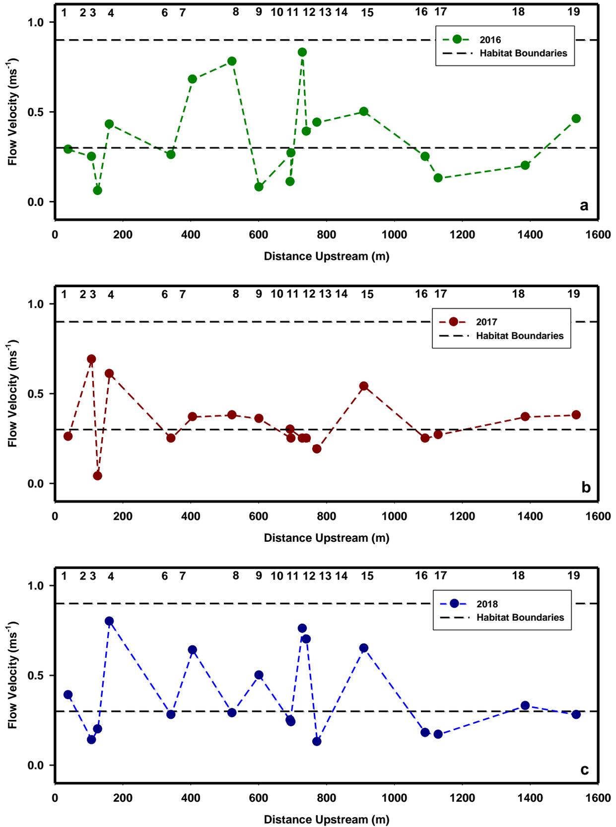
Figure 32. 2016 (a), 2017 (b), and 2018 (c) HEC-RAS  $0.100 \text{ m}^3\text{s}^{-1}$  simulated average flow velocity  $\text{ms}^{-1}$  at each cross-section. The dotted lines represent the critical velocity habitat requirements  $0.3 - 0.9 \text{ ms}^{-1}$  for spawning Coho salmonids (Bjornn & Reiser, 1991).
