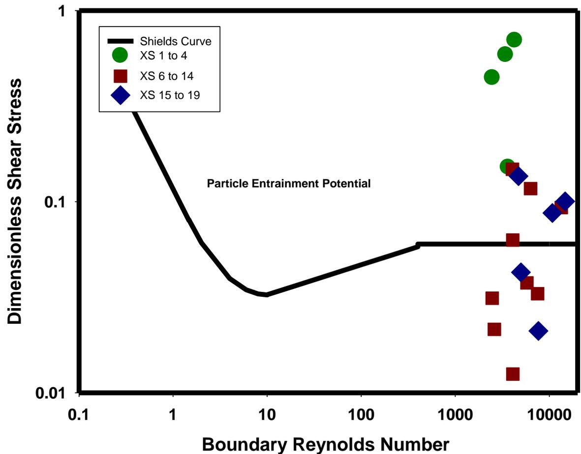
Figure 25. 2018 calculated dimensionless shear stress and Boundary Reynolds number per cross-section plotted against the critical shear stress for particle entrainment curve at  $2.7 \text{ m}^3\text{s}^{-1}$  discharge.
