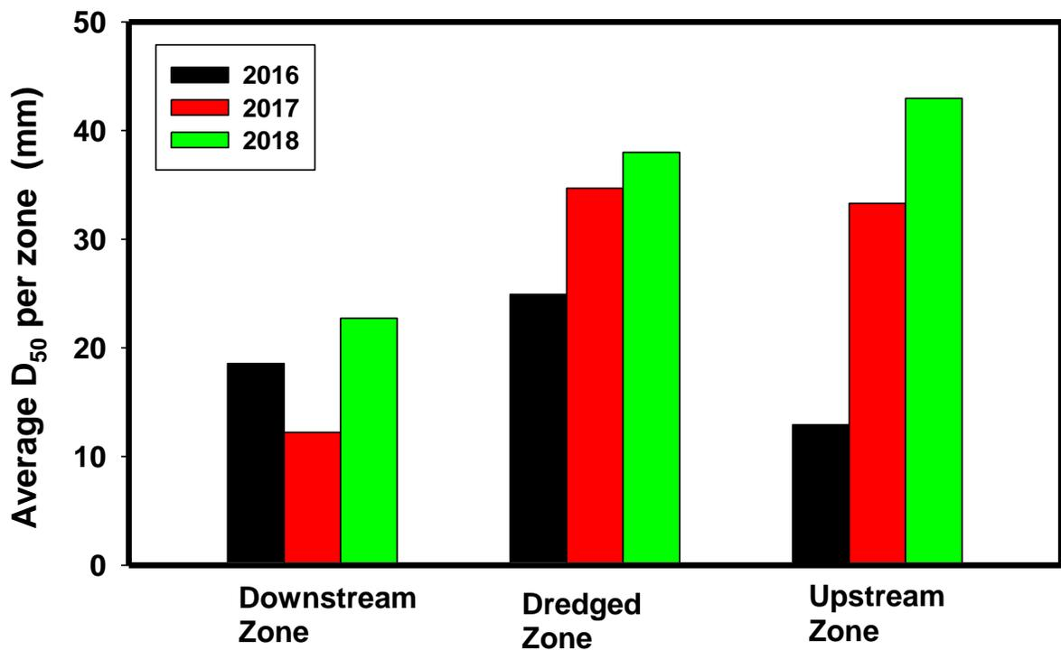
**Figure 21.** Compares the average D<sub>50</sub> (mm) in the downstream zone (cross-sections 1, 2, 4) to the dredged zone (cross-section 6-15) and the upstream zone (cross-sections 16-19).
