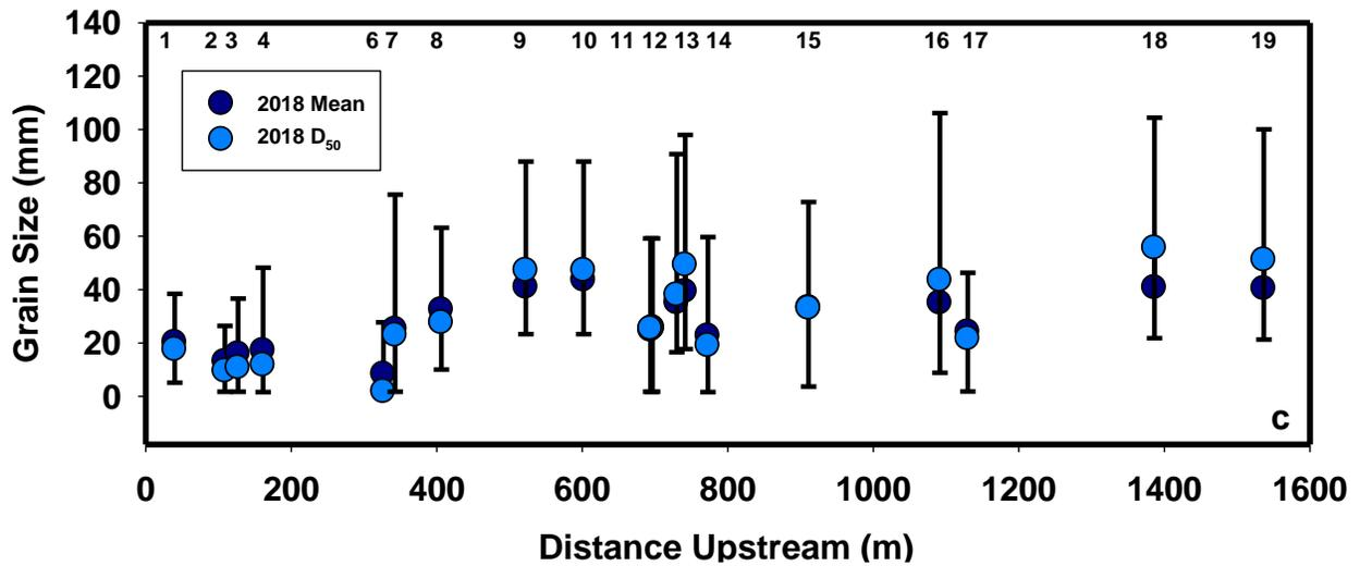
Figure 15. 2016 (a), 2017 (b), and 2018 (c)  $D_{50}$  and mean per cross-section. The upper whisker presents the  $D_{90}$  and the lower represents the  $D_{10}$  per cross-section.
