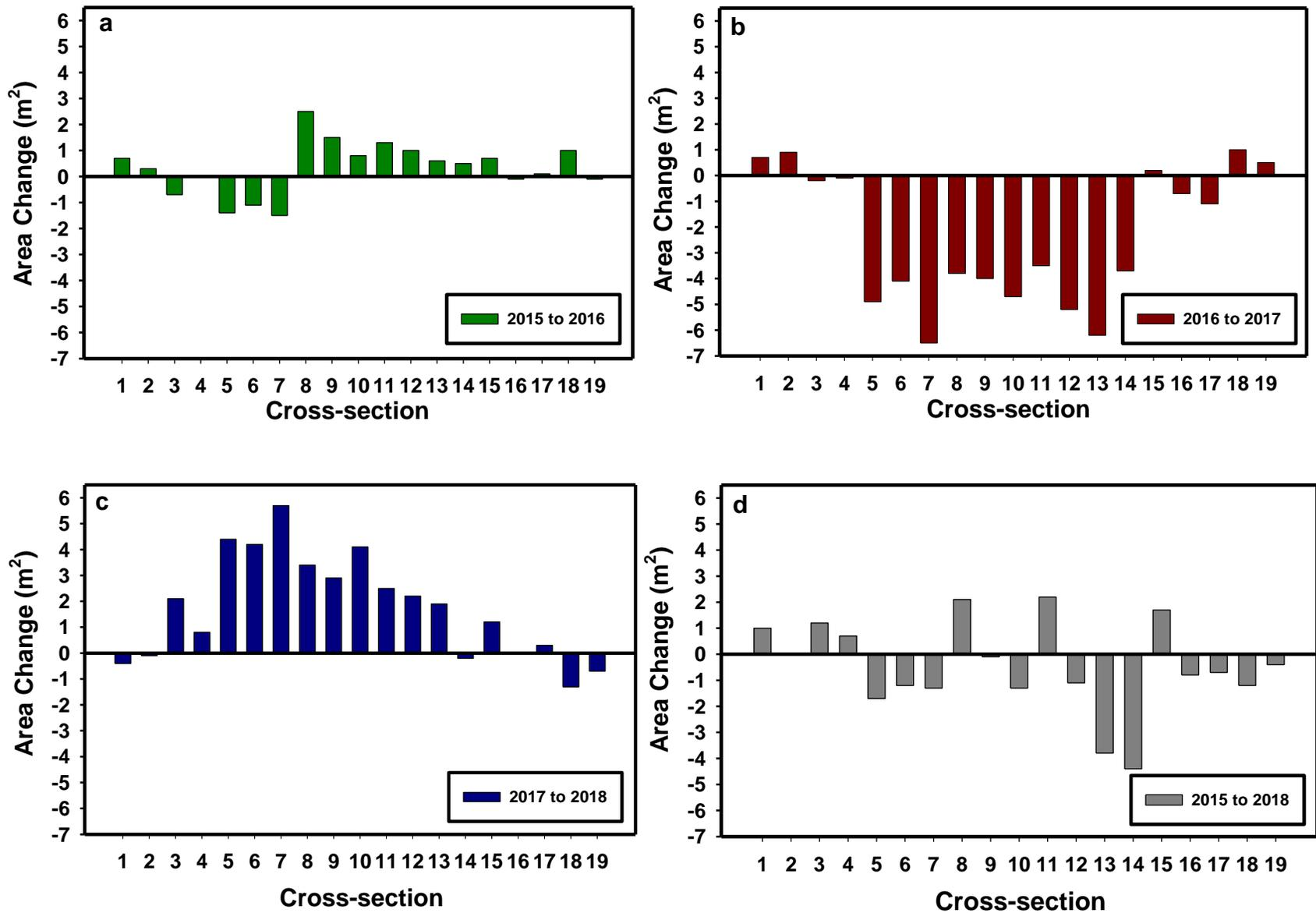
Figure 14. Change in cross-section area (m<sup>2</sup>), calculated using WINXSPRO, within the bankfull width per cross-section 2015 to 2016 (a), 2016 to 2017 (b), 2017-2018 (c), and 2015 to 2018 (d).
