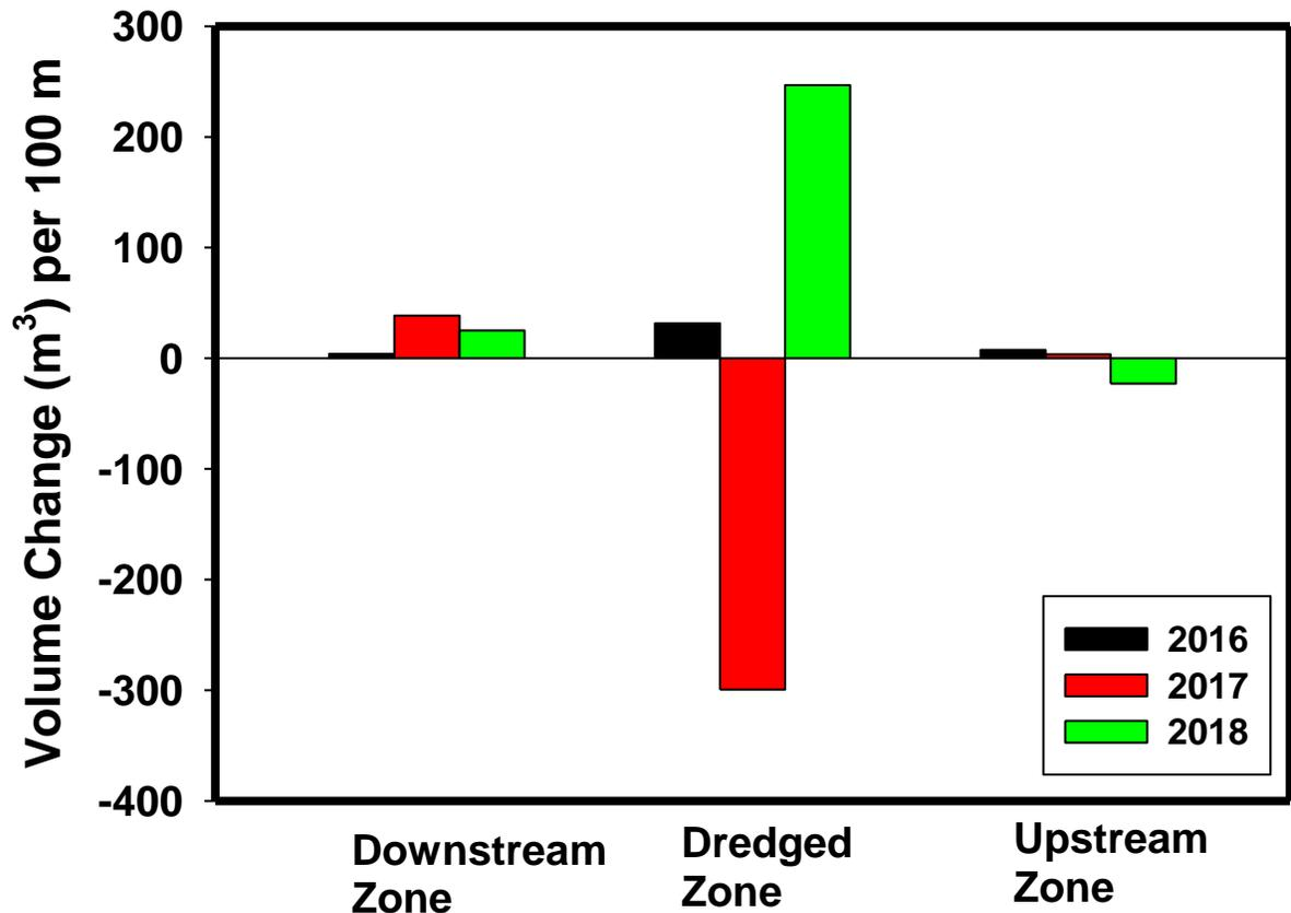
Figure 20. Compares the rate of volume change ( $\text{m}^3$ ) of the active portions of the channel per 100 m reach length in each zone. The downstream zone represents cross-sections 1 to 4. The dredged zone represents cross-sections 5 to 15 and the upstream zone cross-sections 16 to 19.
