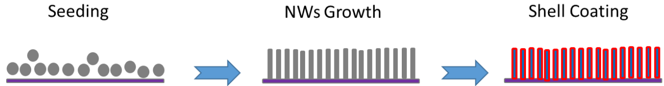
Figure 6-1: Schematic illustration of the core-shell nanowires synthesis process
