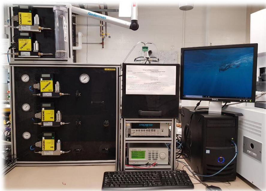
Figure A1-1: Experimental platform, composed of a delivery section to control the gas flow and concentrations through a set of MFCs, a sensing chamber to expose the sensor to the photons and gas (in the black box), and the electrical section which powers the LED and sensor, also monitors the sensor resistance by using a digital Multimeter.
