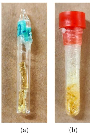
Figure 7.12: Sample PG1 (a) as originally packed in a sealed NMR tube and (b) after being opened and manually cut and compressed to introduce mechanical stress.
