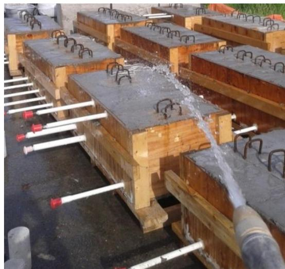
B-Beam specimen curing
