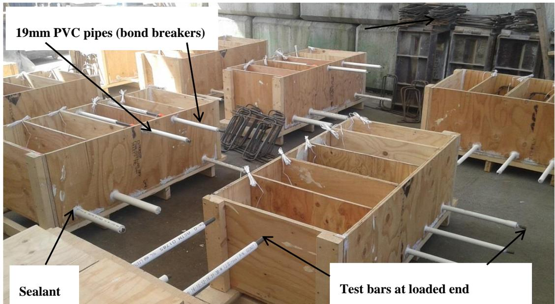
Figure 3.9 Completed formwork with test bars and embedded in PVC and sealed
