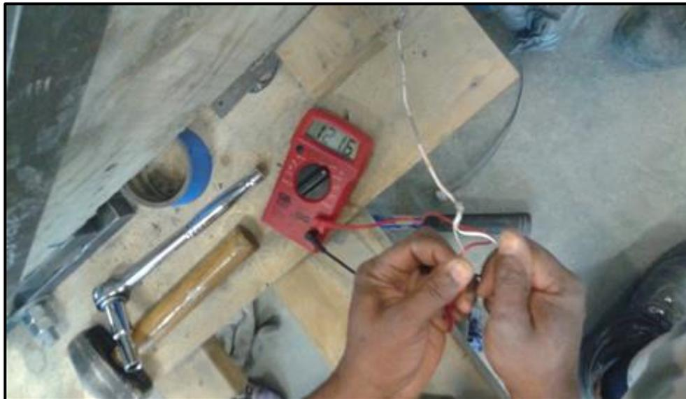
Figure 3.16 Strain gage pretesting from specimen lead wires
