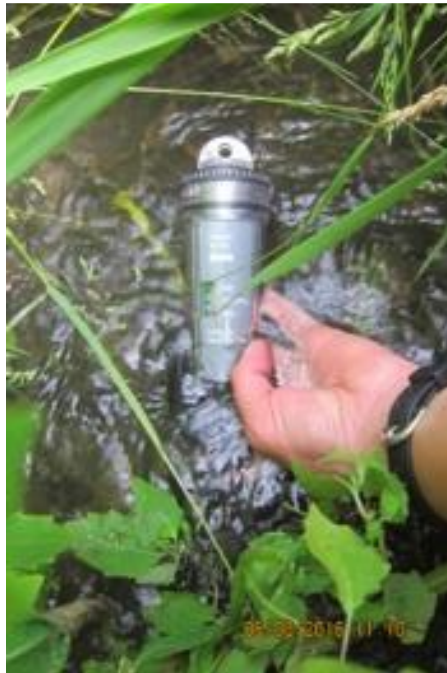
Figure 3.4. HOBOWare shuttle attached to the temperature pendants in the creek to download data stored on the pendants.
