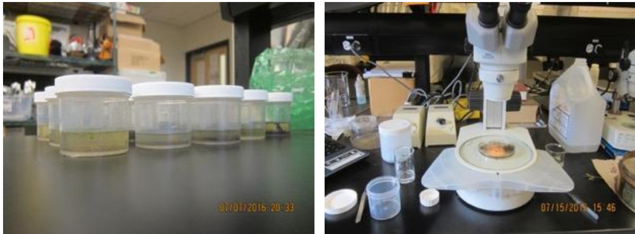
Figure 3.13 Left: macroinvertebrates samples preserved in 95% ethanol. Each jar represents various locations and dates of collection. Right: sample in a petri dish under a stereo zoom microscope to count Ephemeroptera, Plecoptera, and Trichoptera occurrences.
