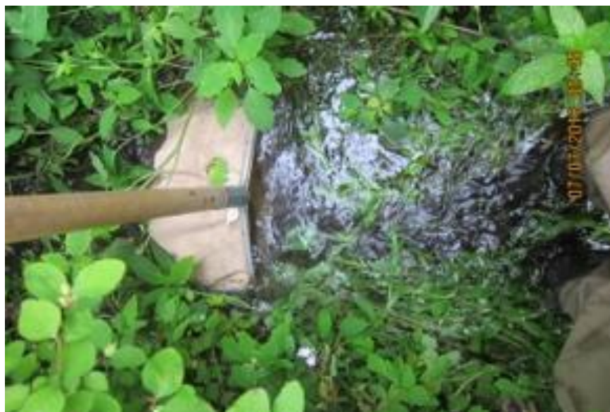
Figure 3.11. Kick net method to collect macroinvertebrate samples in Alderson Creek.
