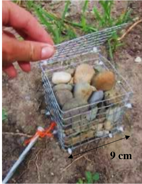
Figure 3.8. Artificial substrate basket consisting of river stone. Wire baskets were secured into the creek bed with a nail and left to collect macroinvertebrates.
