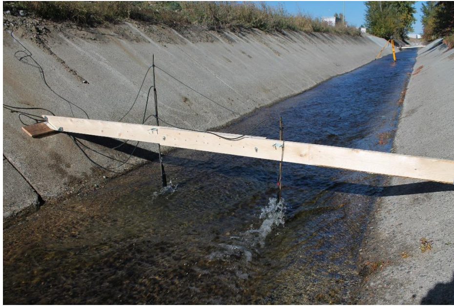
Figure 16. Conductivity and turbidity sensors in the concrete channel.
