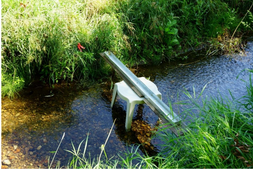
Figure 14. The trough utilized for the injection of sodium chloride and sediment in the semi-natural channel at the injection site.
