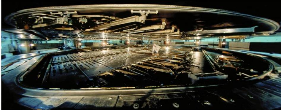
Figure 2.3: Internal view of the 520 MeV main cyclotron vault at TRIUMF. Notice the size of the vault compared to the man at the center. Adapted from Ref. [94].
