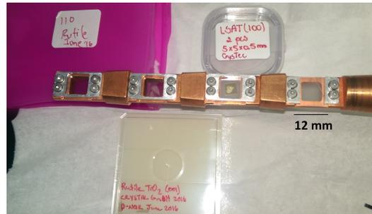
Figure 2.9: The  $\beta$ -NQR sample holder (made of copper) with four samples mounted. In contrast to the  $\beta$ -NMR one, it has four sample stations, which reduces significantly the number of sample changes needed during an experimental run period.
