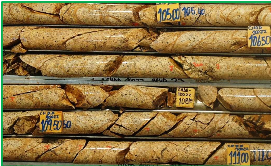
Figure 3.9. Photograph of drill core with defects. Infill of defects and joints coating correspond to the same mineralogy of iron oxides and gypsum. Orientation of defects and open joints is in various cases similar.
