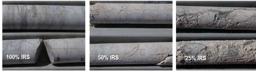
Figure 2.6. Influence of defects intensity in the intact rock strength estimation. Is not uncommon that, as in the case in the central and right photographs, defects are difficult to assign to any type of geological feature. IRS: Intact Rock Strength (From Jakubec, 2013).
