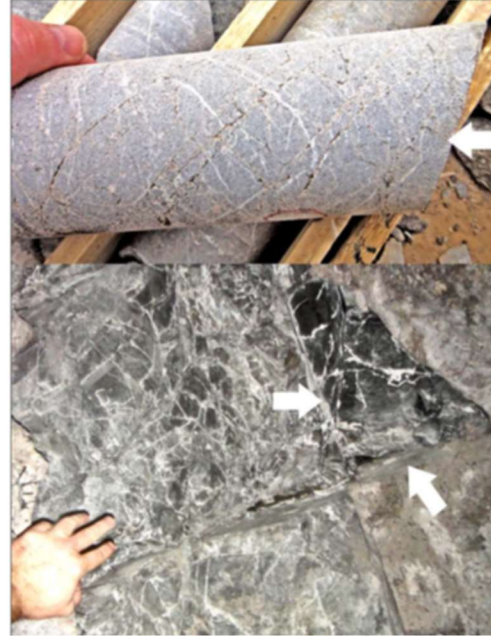
Figure 2.8. a) Adjustment factor to determine rock block strength based on Laubscher and Jakubec (2000) procedure (from Bewick et al., 2019) b) White arrows indicate joints bounding the “intra block structure” included in Day’s Compound GSI (modified from Day et al., 2012).
