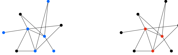
Figure 1.9: Example of a vertex cover and a minimum vertex cover
