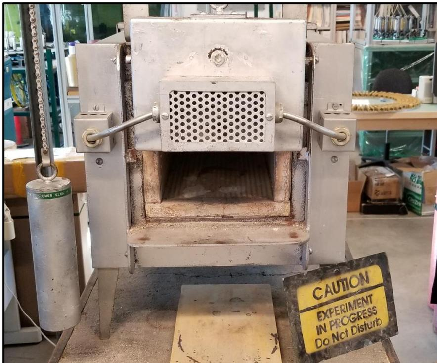
Figure 3.10 Muffle furnace
