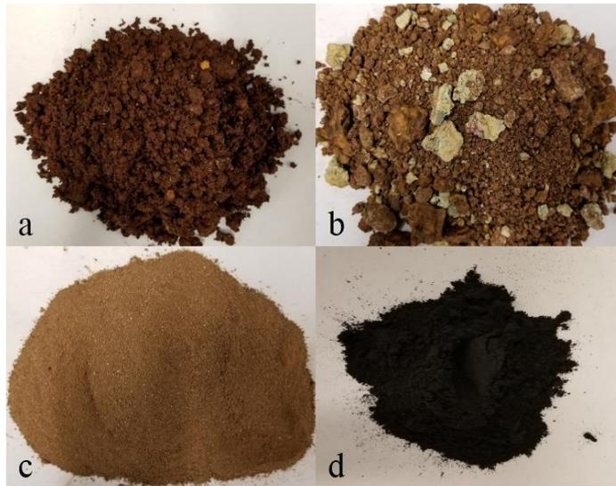
Figure 3.3 (a) As-received ore (b) Dried ore (c) Ground ore (d) Ground coal
