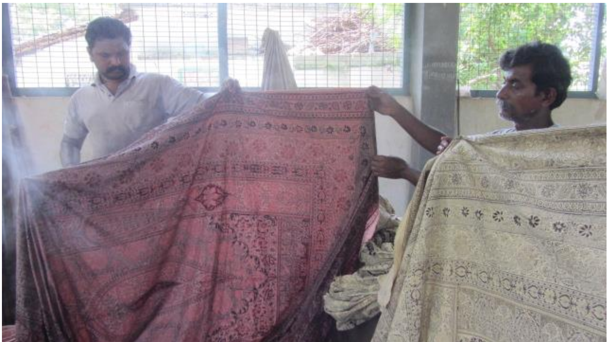
Figure 2.12: Difference of color, before (right) and after (left) of the dyeing, Polavaram, 2015.
