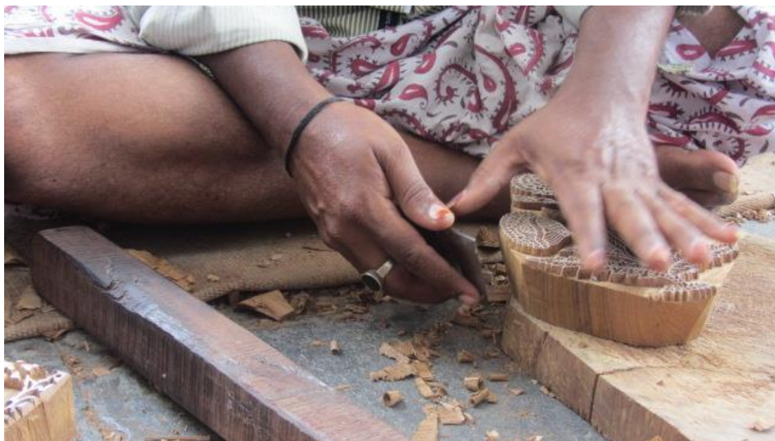
Figure 3.15: Beveling and trimming of blocks, Kondra brothers workshop, Pedana, 2015.
