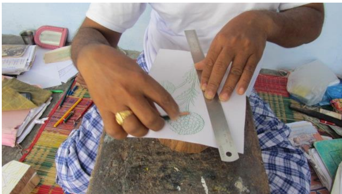
Figure 3.16: Taking a rubbing print of a newly prepared block, Kondra brothers' workshop, Pedana, 2015.
