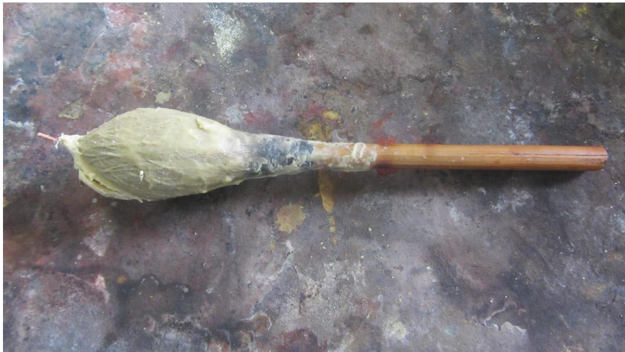
Figure 4.17: Kalam for wax resist drawing, Weavers' Service Centre, Hyderabad 2017.
