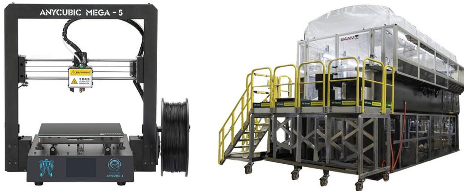
Figure 1.6: Printer comparison. Left: desktop FDM printer (scale: 1:10) [34]; Right: BAAM printer (scale: 1:150) [33].
