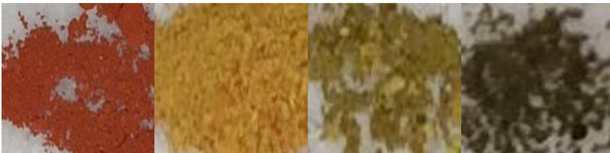
Figure 5.13 – Photographic images of jar-mixed \text{Fe}_2\text{O}_3 ( <5\ \mu\text{m} ) and \text{Na}_2\text{CO}_3 ( 38\text{--}63\ \mu\text{m} ) at 298 K (red), and after heating to 1023 K (yellow), 1123 K (green) and 1223 K (dark-brown).
