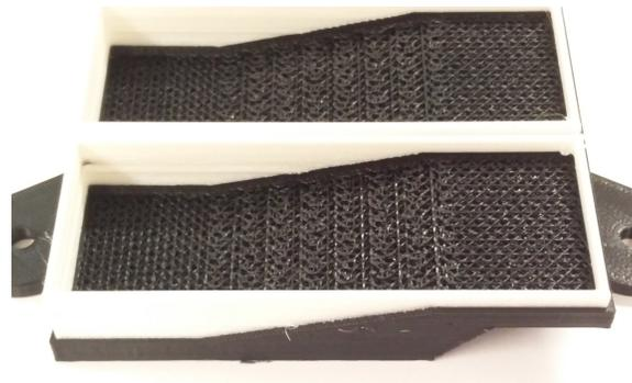
**Figure 2.12:** Close-up of the phantom tray before silicone casting, showing lattice base and removable (disposable) mold walls.
