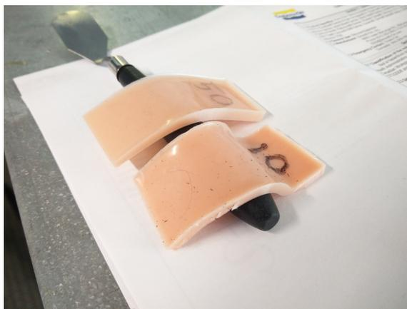
**Figure 2.10:** Two silicone phantoms cast outside the tray, demonstrating different levels of softness with variant resting configurations.
