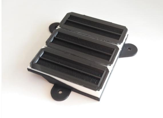
**Figure 2.13:** Phantom tray during silicone casting, with mold caps installed.
