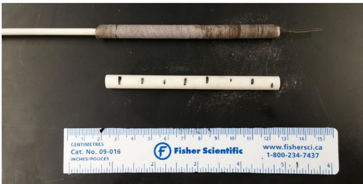
Fig. S1. Photograph of the calibration heater and a tubular alumina crucible. The calibration heater and its leads are formed from a continuous length of Kanthal A1 resistance wire. Each of the two leads has a resistance of approximately 2.7\Omega while the leads and coil combined have a resistance of approximately 33\Omega . Thus only 83.6% of the nominal power dissipated in the heater is dissipated in the coil. The measurement of the power dissipated in the calibration heater could be made more accurate through the use of 4-wire power measurement and/or heater current supply leads to having lower resistance. (Reproduced from MacLeod et al. , Review of Scientific Instruments 88 , 084101 (2017), with the permission of AIP Publishing)
