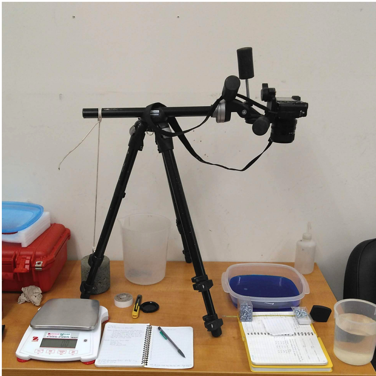
Figure 2.4: The method of photographing an evaporation pan with blue dyed water for the determination of the pan water surface area.
