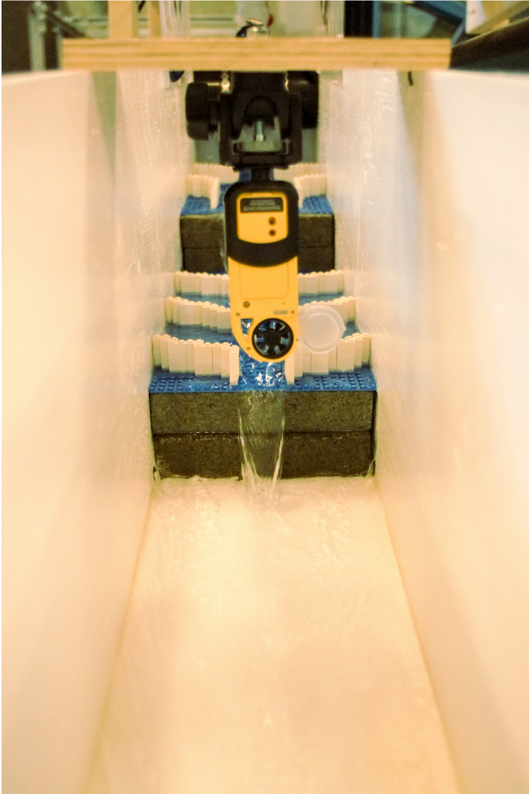
Figure 3.3: Photograph showing the Kestrel weather meter measuring the wind speed over the surface of the flow in the flume. The impeller is approximately 20 cm above the surface of the flow.
