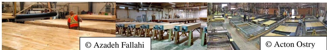
Figure 7-6 CLT panels, GLT columns, and envelop panel at off-site manufacturing facility (Image source: Fallahi (2017) & Acton Ostry Architects)
