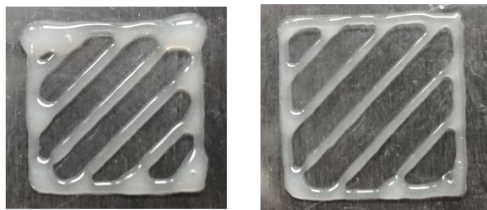
Figure 4.16: Evaluation of the effect of the PWM-based synchronized dispensing: on the left is constant dispensing, and on the right is when synchronized dispensing is used.
