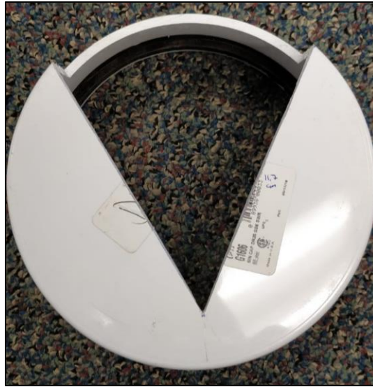
Figure 4.5: PVC weir cap with 53.13^\circ V-notch
