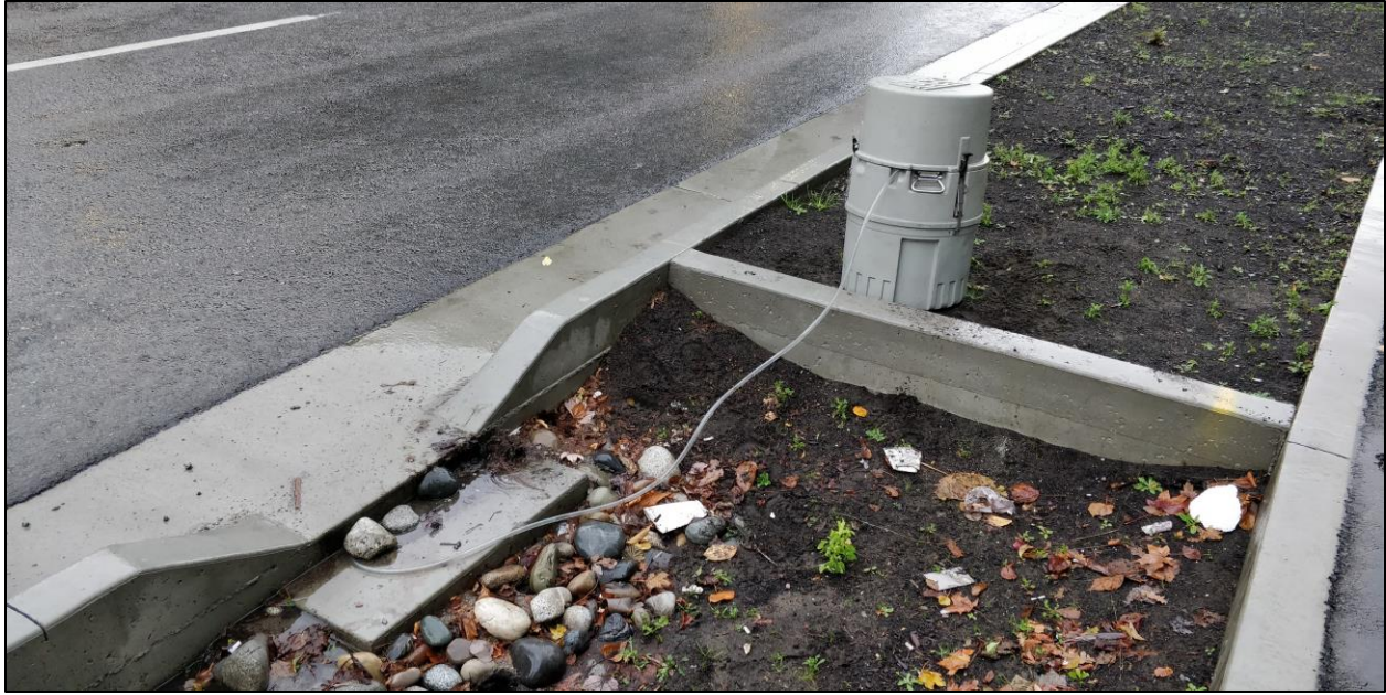
Figure 4.33: ISCO® 3700 sampler deployed at Bioswale 1 for inflow sampling
