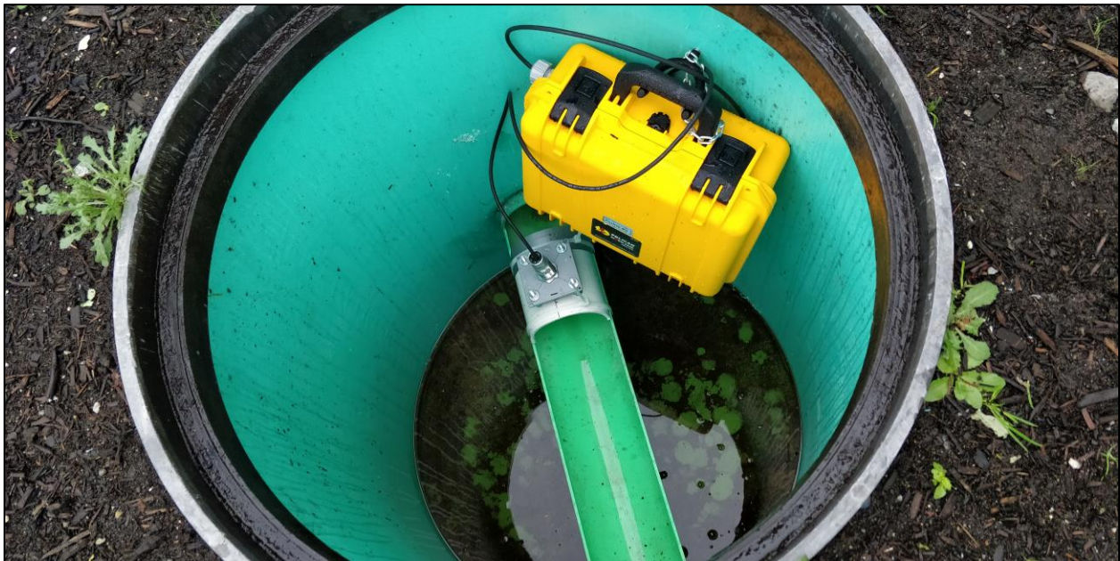
Figure 4.21: Flow sensor system installed in through pipe and data logger deployed in the field
