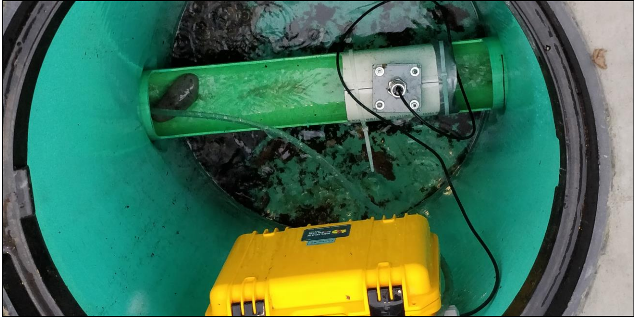
Figure 4.35: PVC tubing sapling from the through channel in the monitoring basin
