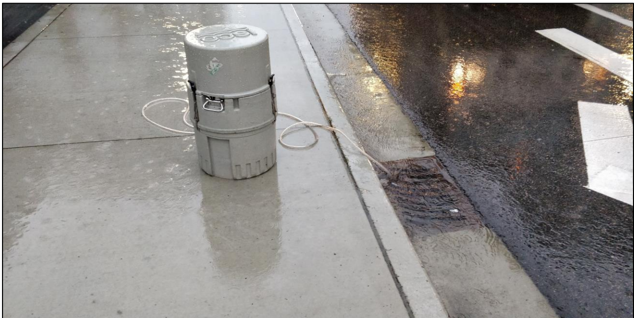
Figure 4.32: ISCO® 3700 sampler deployed at structural soil STT for inflow sampling
