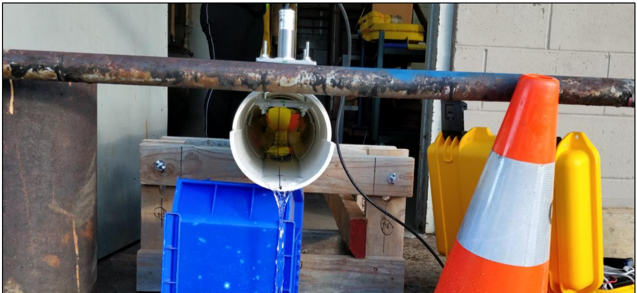
Figure 4.23: Flow experiment capture which shows flow width changes due to coupling transitions
