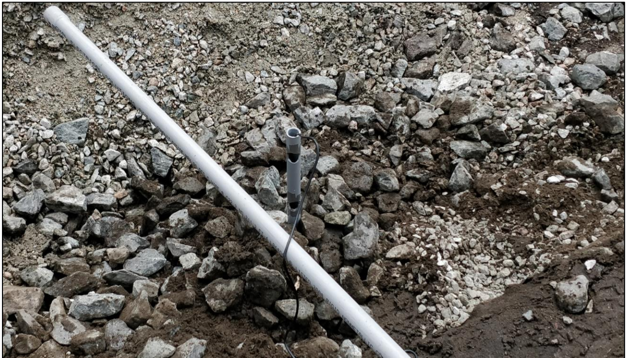
Figure 4.29: Installation of second soil sensor at a 40cm depth. The cables of the soil sensors were slipped into the holes in the PVC pipe for protection. 1" PVC pipe left by CoV crews
