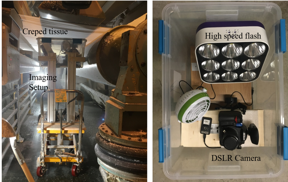
Figure 3.3: Online crepe count quantification setup in a real tissue machine (left). Components of the high speed imaging setup (right).
