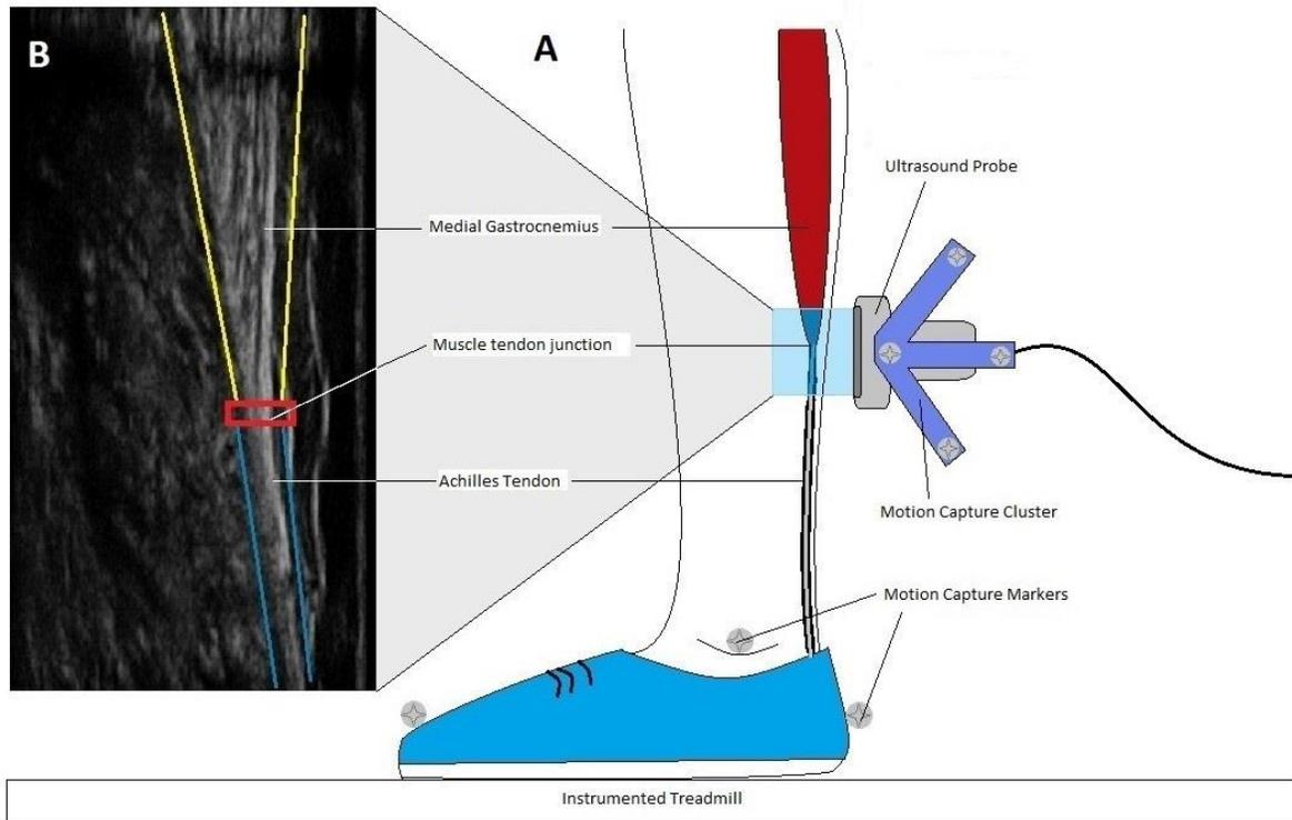
**Figure 5. (A) Methodological set-up of ultrasound and motion capture markers. (B) Ultrasound visualization of the GM, MTJ and AT to quantify AT displacement during data collection.**
