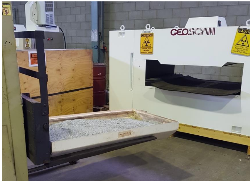
Figure 3.9 Sample being loaded into Geoscan-M with conveyor belt cut-off (Balzan, 2016)
