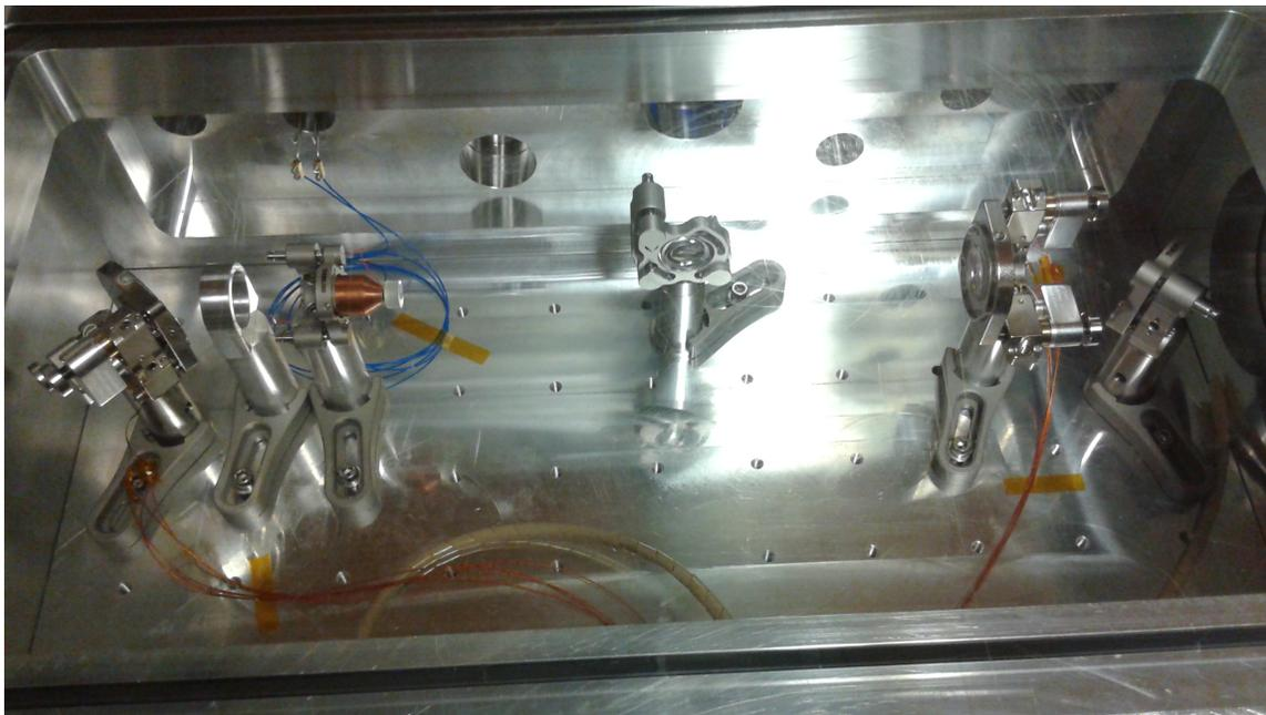
**Figure 4.11:** Photo inside the vacuum box, showing turning mirror from brewster window UV input; holder for QWP and lens; input coupler and PZT mounted to hollow copper block; LIF collection lens; HR mirror; turning mirror to UV cavity monitor.
