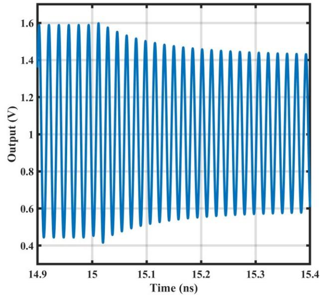
Figure 19. Simulated output signal after applying a pulse at the gate of the switch.
