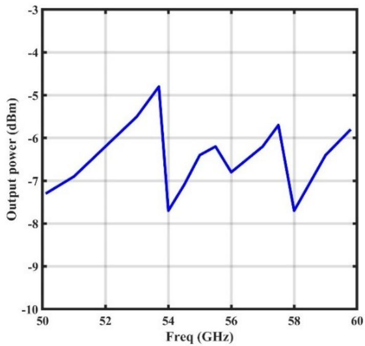
Figure 41. The measured output power over the whole frequency tuning range.
