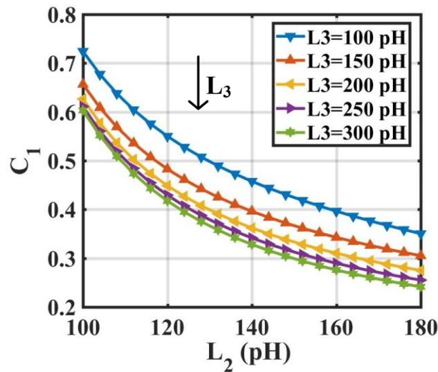
Figure 7. Simulated  $C_1$  versus different values of  $L_2$  and  $L_3$ .
