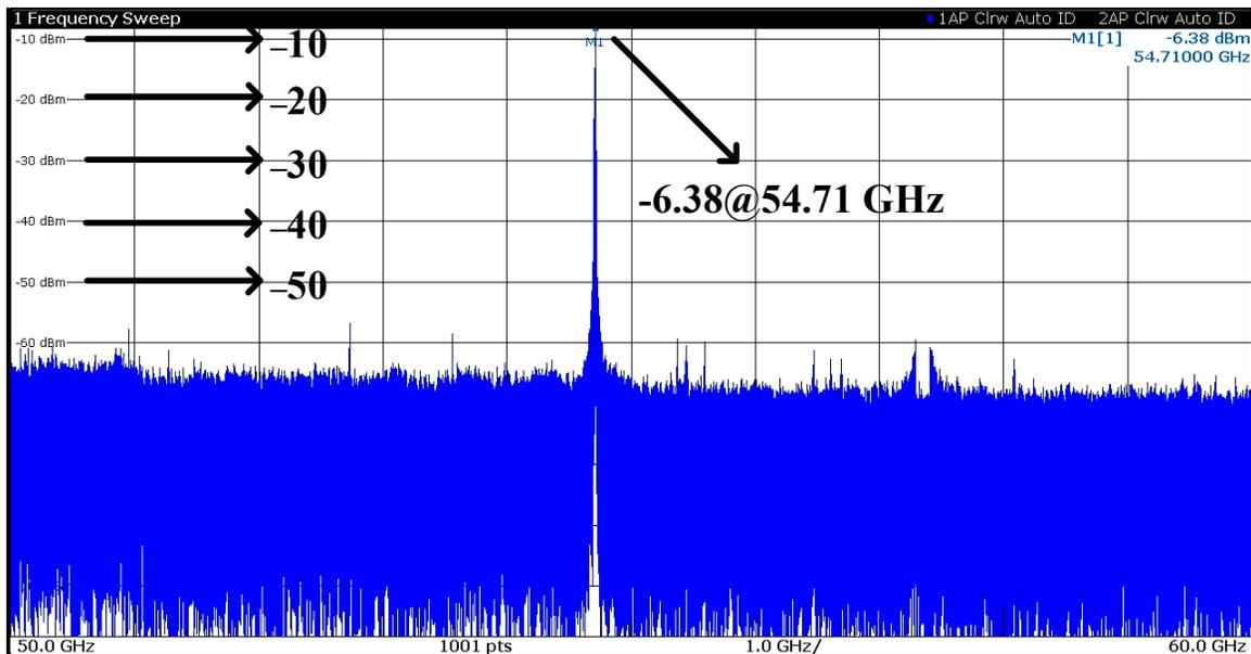
Figure 38. Output spectrum of the fabricated VCO.
