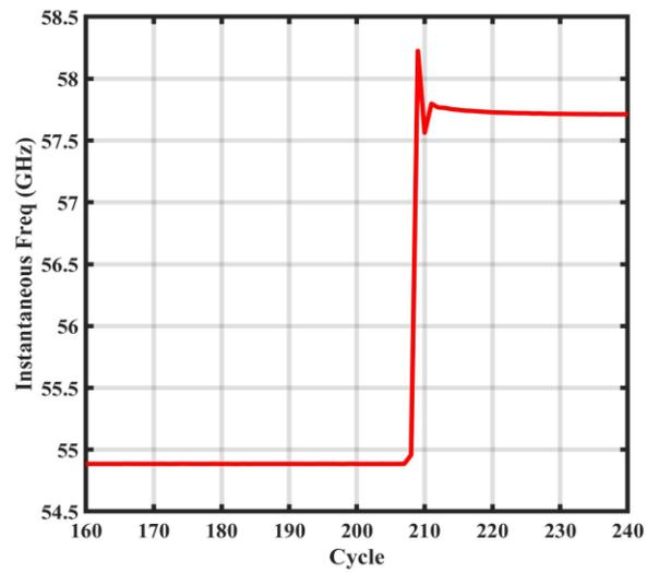
Figure 20. Transient response of the oscillation frequency after applying a pulse at the gate of the switch.
