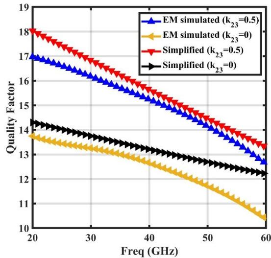
Figure 18. Q factor comparison between that of the proposed model and transformer.
