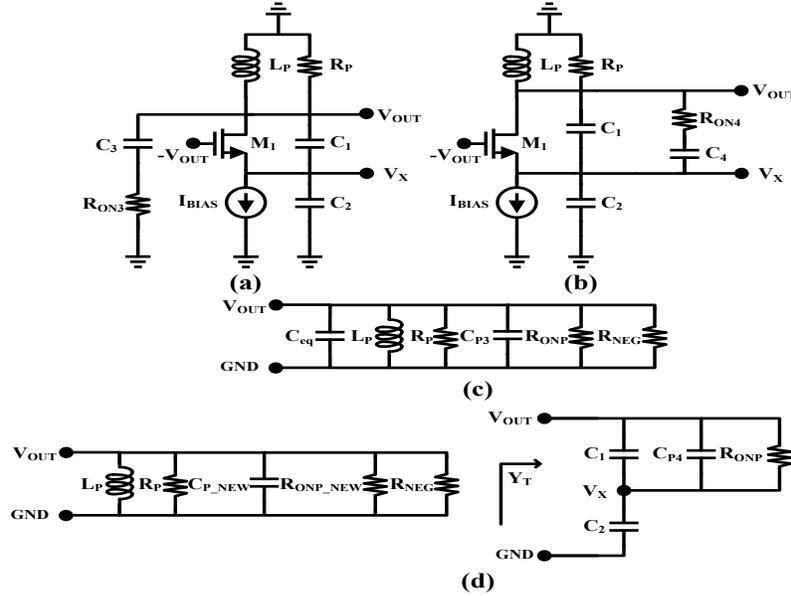
Figure 22. Half-circuit and small-signal models of : (a, c) conventional switching network (b, d) proposed switching network.
