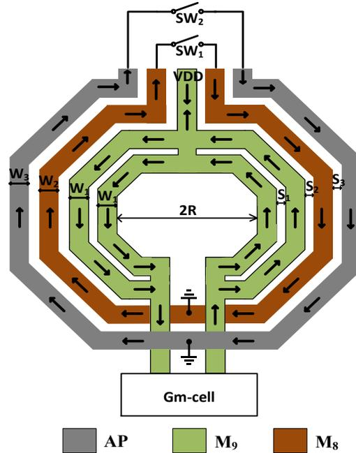
Figure 14. Top view of the proposed switchable transformer.
