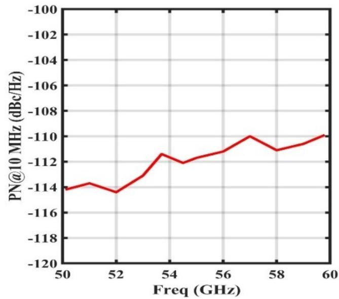
Figure 40. The measured PN at 10-MHz offset over the whole frequency tuning range.
