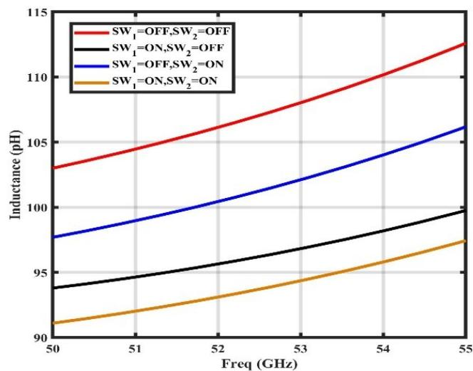
Figure 11. Simulated effective inductance over the whole frequency tuning range.
