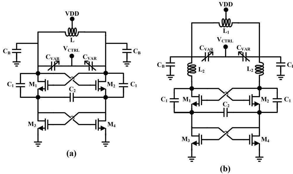
Figure 25. Schematic of the (a) conventional Colpitts VCO; (b) proposed gm-boosted Colpitts VCO.
