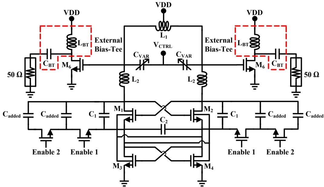
Figure 35. Schematic of the fabricated VCO.
