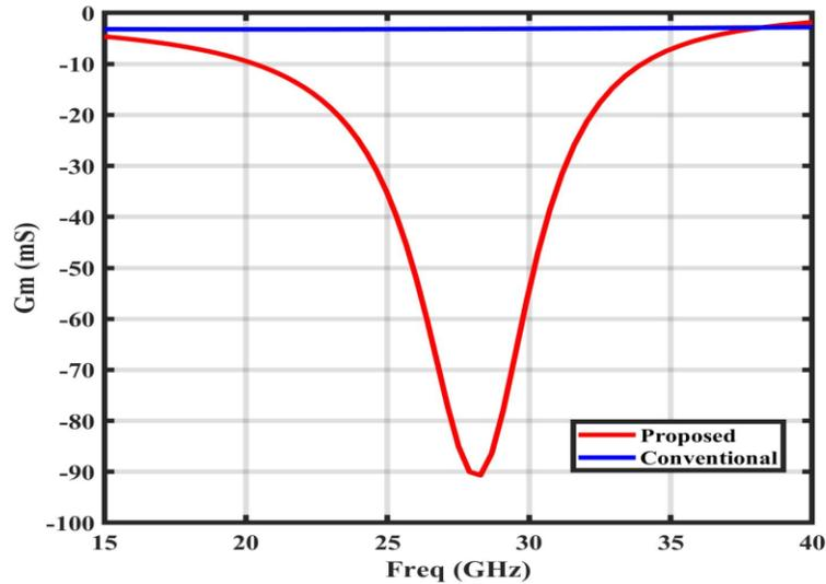
Figure 27. Comparison of the simulated small-signal negative transconductance in conventional and proposed topology.
