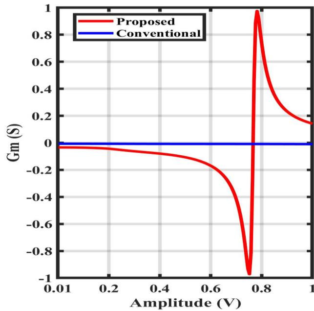
Figure 29. Comparison of simulated equivalent parallel transconductance in Conventional and proposed technique.
