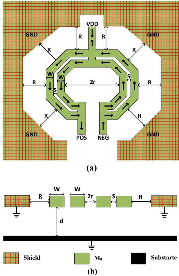
Figure 36. Different views of the proposed tank; (a) top; b) cross sectional.
