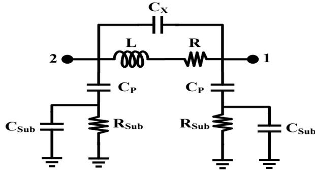
Figure 17. A high frequency circuit model of an inductor.
