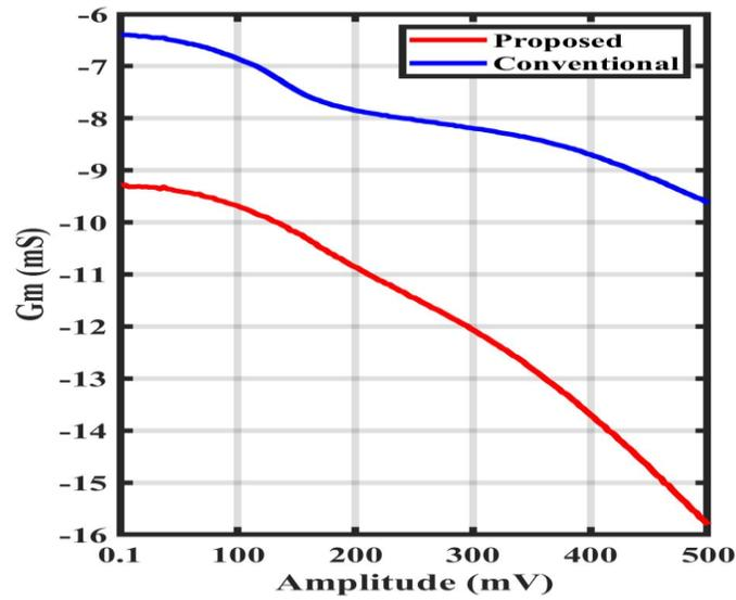
Figure 32. Comparison of the simulated negative transconductance in conventional and proposed body bias technique.
