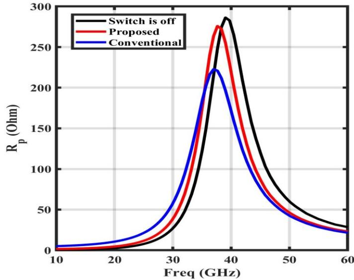
Figure 24. The simulated loss of the tank in conventional and proposed structures.
