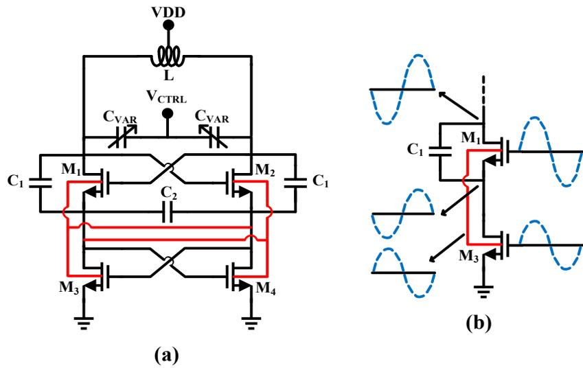
Figure 31. The proposed body bias technique; (a) schematic (b) corresponding signals.
