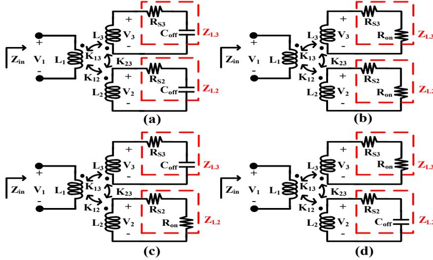
Figure 1. The simplified model for the proposed inductive tuning technique; (a) SW1 and SW2 are off; (b) SW1 and SW2 are on; (c) SW1 is on and SW2 is off; (d) SW1 is off and SW2 is on.
