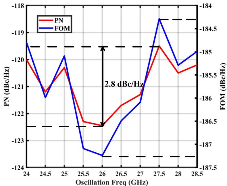
Figure 47. Measured PN and FOM at 10-MHz offset from the carrier over the entire tuning range.
