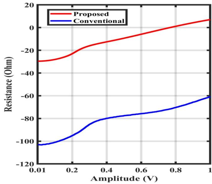
Figure 28. Comparison of simulated equivalent parallel resistance in Conventional and proposed technique.
