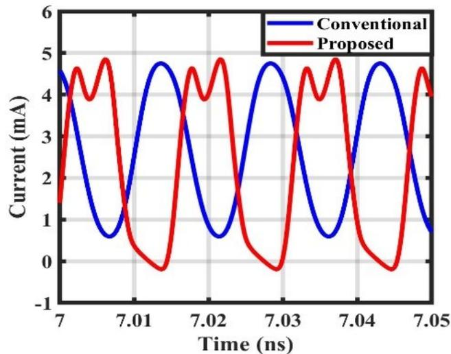
Figure 34. The simulated transient drain current of  $M_1$ .
