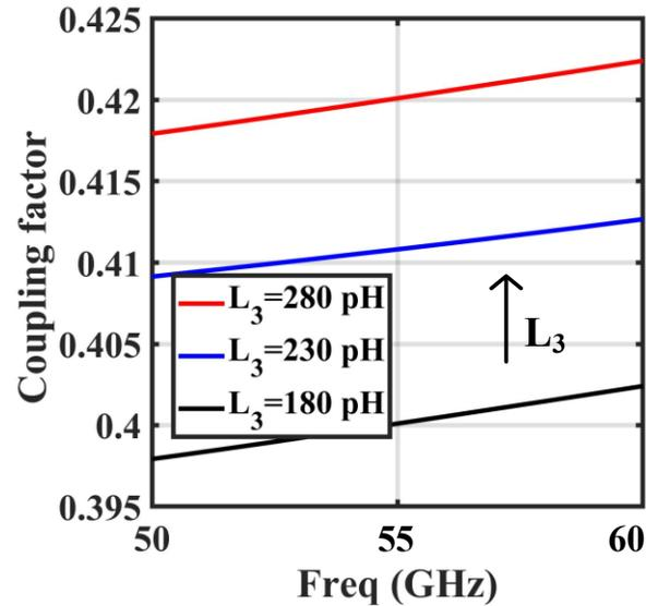
Figure 9. Dependency of the coupling factor on  $L_3$ .
