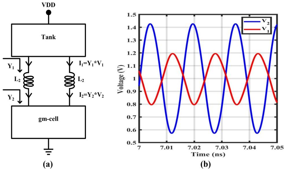
Figure 30. System-level model of the proposed gm-boosting technique. (b) Simulated transient signals at  $V_1$  and  $V_2$ .
