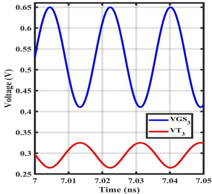
Figure 33. Simulated transient response of the proposed body bias technique.
