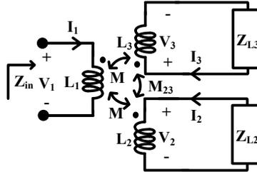
Figure 5. Simplified model of the transformer where both switches are on (or off).
