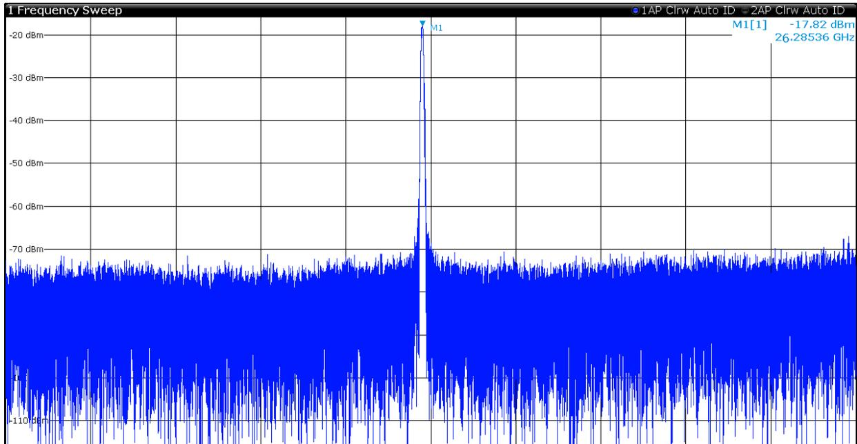
Figure 44. Measured output spectrum of the fabricated VCO.
