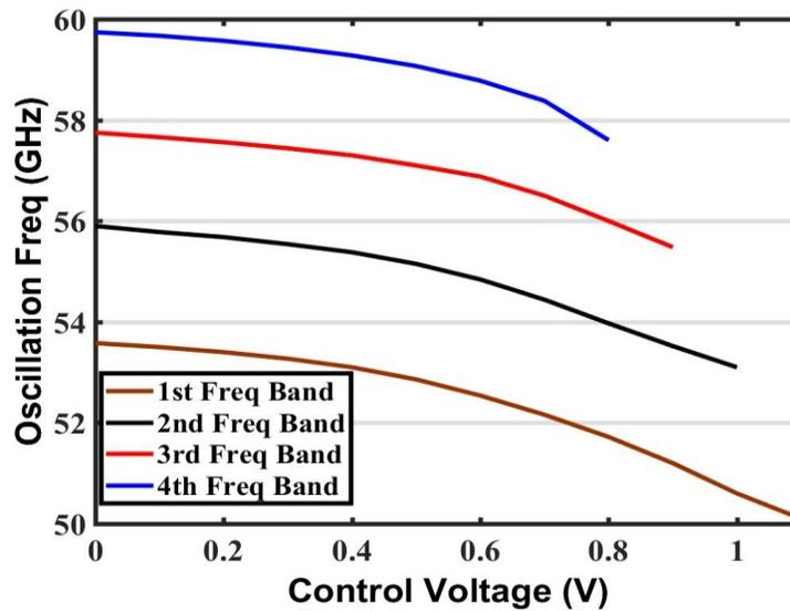
Figure 42. Measured frequency tuning range over different control voltages.
