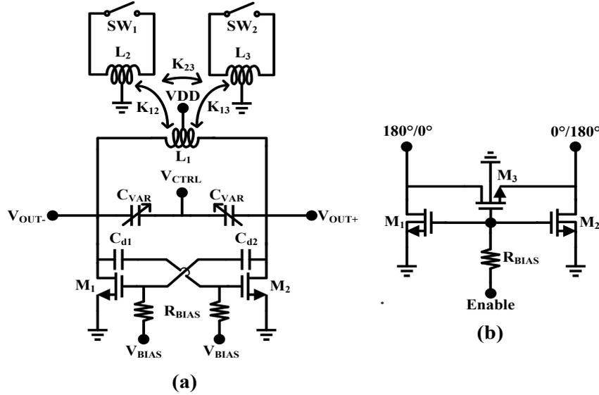
Figure 12. Schematic of the proposed (a) VCO. (b) The proposed switch architecture.
