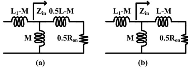
Figure 4. Simplified  $\pi$ -model of the transformer when; (a)  $K_{23}=0$ . (b)  $K_{23}=1$ .
