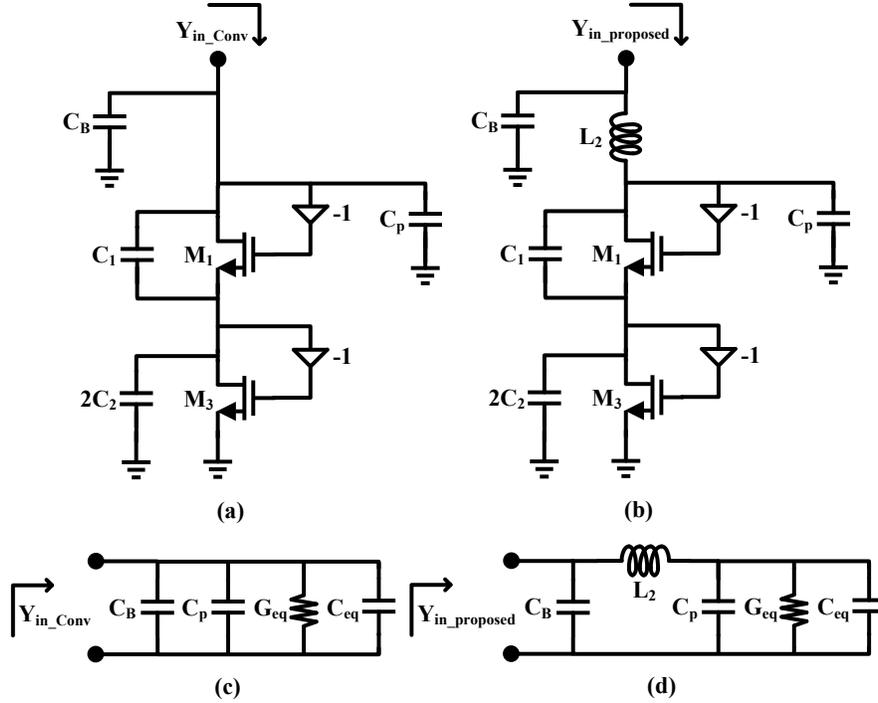
Figure 26. The simplified and small signal model of the (a, c) conventional Colpitts VCO; (b, d) proposed Colpitts VCO.
