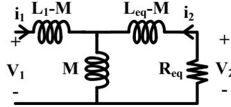
Figure 6. Simplified pi-model for one of transformers.
