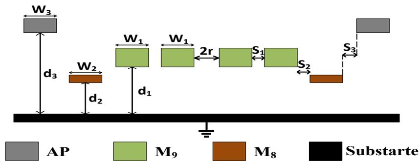
Figure 13. Cross section view of the proposed switchable transformer.
