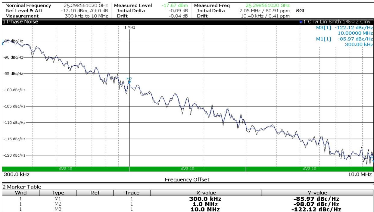
Figure 45. Measured phase noise of the fabricated VCO at the center frequency of oscillation.
