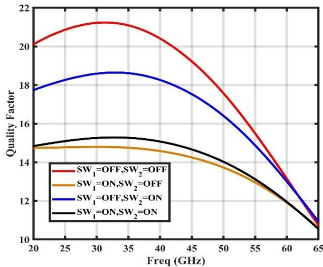
Figure 10. The simulated Q-factor over all switch states.
