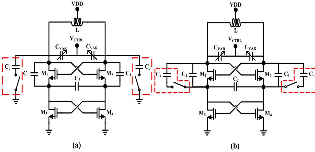
Figure 23. Schematic of the conventional differential Colpitts VCO with a one-branch capacitor bank (a) conventional; (b) proposed.
