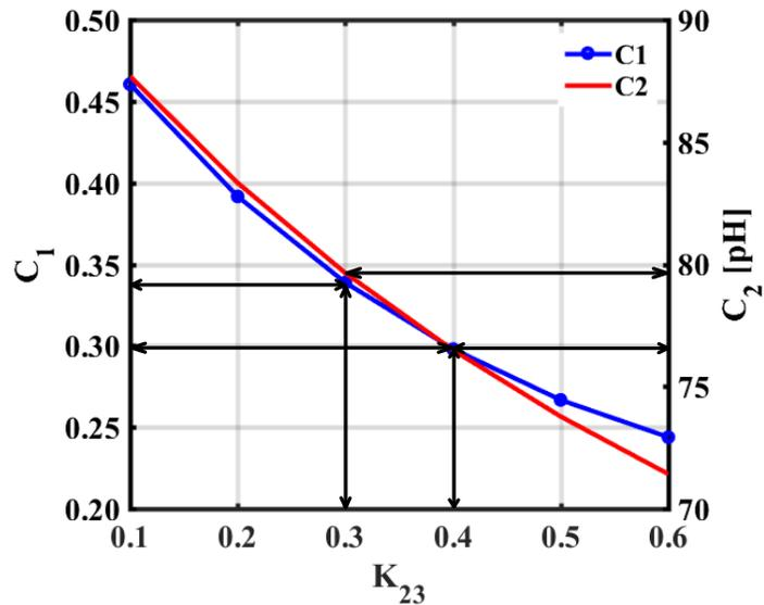
Figure 3. Plotted  $C_1$  and  $C_2$  versus  $k_{23}$  with  $L_2=210$  pF,  $L_3=250$  pF, and  $M=115$  pF.
