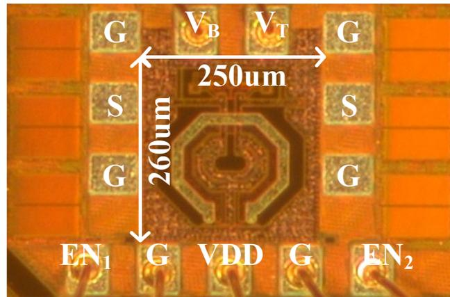
Figure 37. Micrograph of the fabricated 60-GHz VCO.
