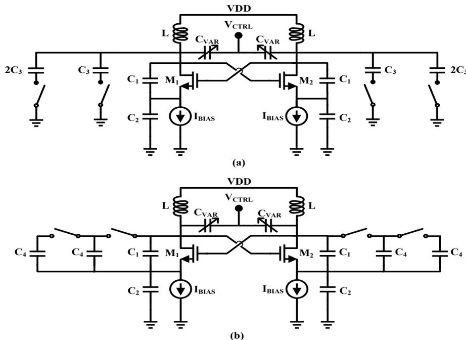
Figure 21. Schematic of the Colpitts VCO with (a) Conventional (b) Proposed capacitor bank. To have a fair comparison of the phase noise between these two VCOs, we consider the same frequency of oscillation and switch size for both cases. In the conventional structure, because of
