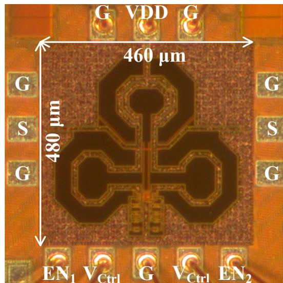
Figure 43. Micrograph of the fabricated 28-GHz VCO.
