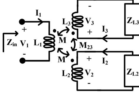
Figure 2. Simplified schematic of the proposed transformer.
