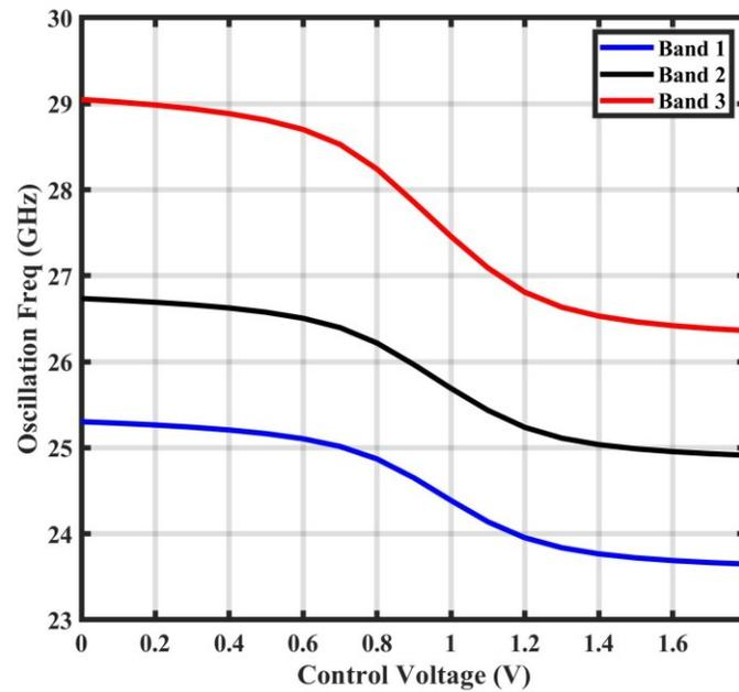
Figure 46. Measured tuning range of the fabricated VCO.
