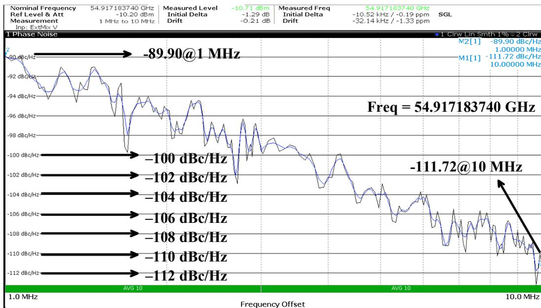
Figure 39. Measured phase noise at the center frequency of oscillation.
