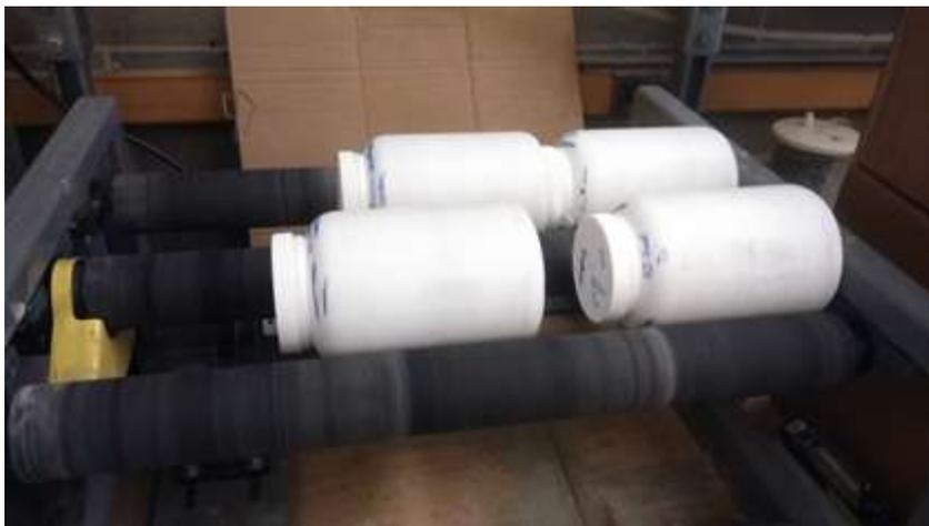
**Figure 6. Laboratory scale bottle roller and plastic bottles used for bottle roll leaching experiments.**
