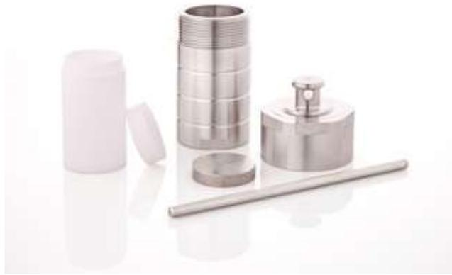
**Figure 4. Pressure autoclave used for hydrothermal precipitation of copper sulfides.**
