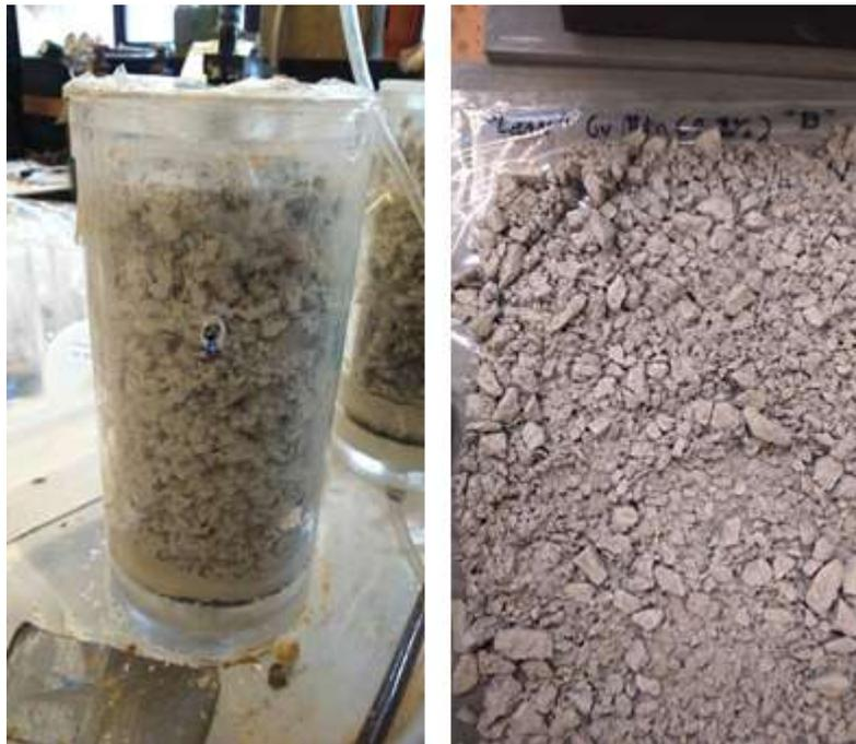
**Figure 5. Small-scale leaching column and low-grade copper sulfide ore sample.**
