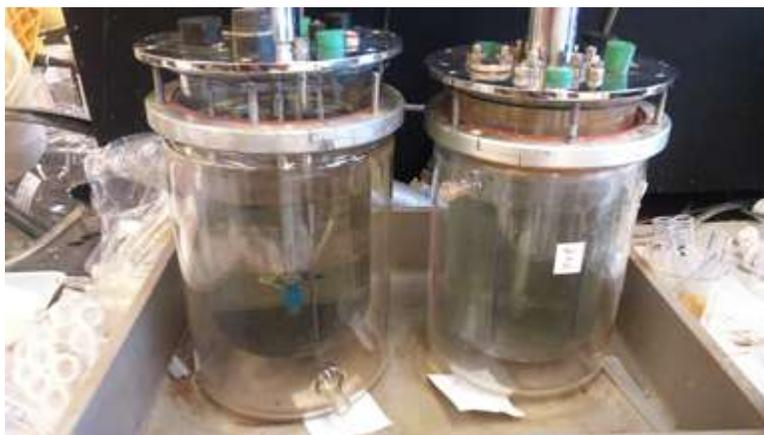
**Figure 3. Agitated glass-jacketed reactors for stirred tank leaching experiments.**
