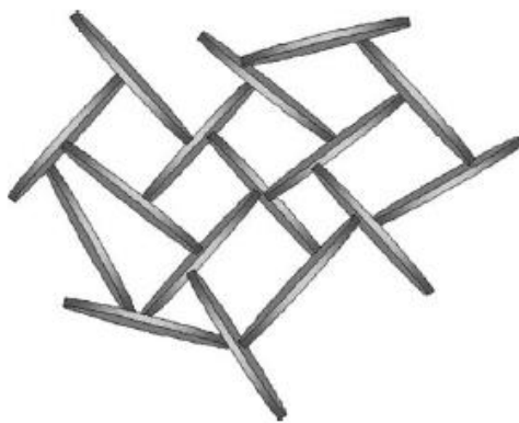
Figure 7.5 House of card structure observed in kaolinite suspension (from [265]).
