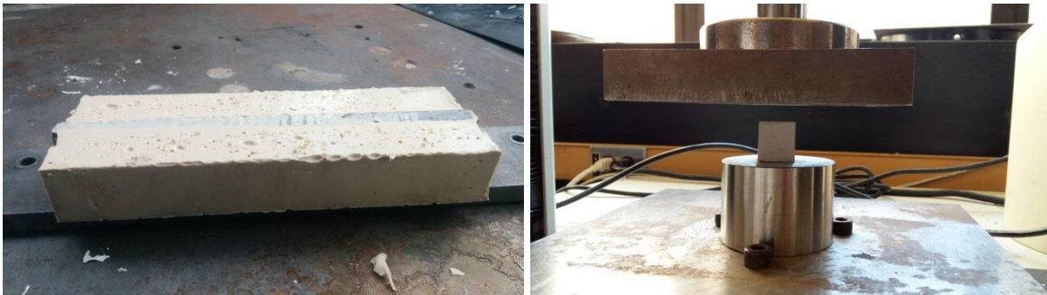
Figure 4.9 Left: Geopolymer bar during demolding operation. Right: GP cube and head of the Instron machine during UCS test.
