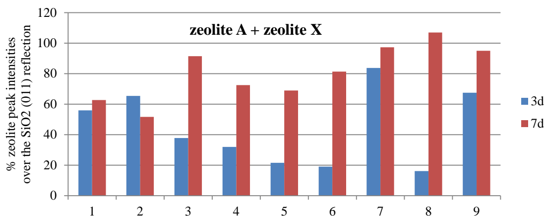
Figure 6.16 Zeolite content expressed in term of sums of XRD integrated intensities of 200) reflection of zeolite A and the (111) reflection of zeolite X over the (011) reflection of SiO 2 at 3 days and at 7 days.
