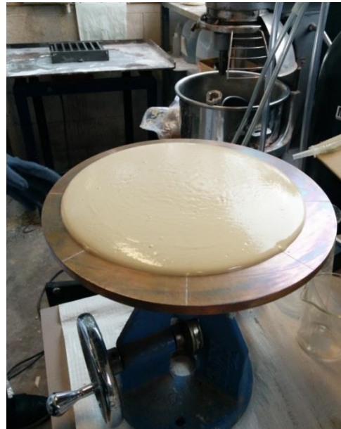
Figure 5.4 Flow table apparatus and flow of the GP with Si/Al=1.35.
