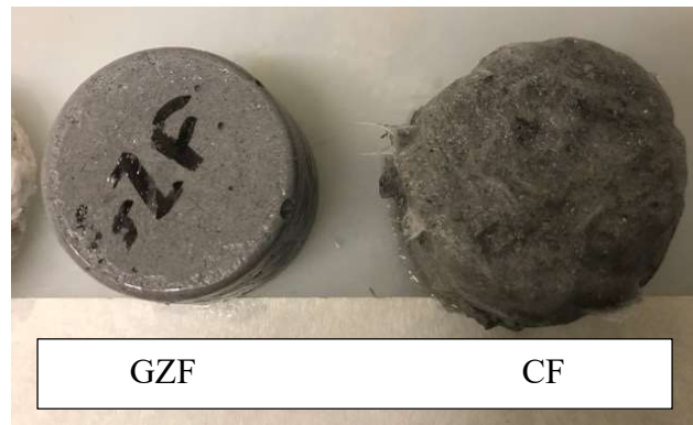
Figure 4-47: Deteriorated samples in acidic environment after 16 weeks of immersion
