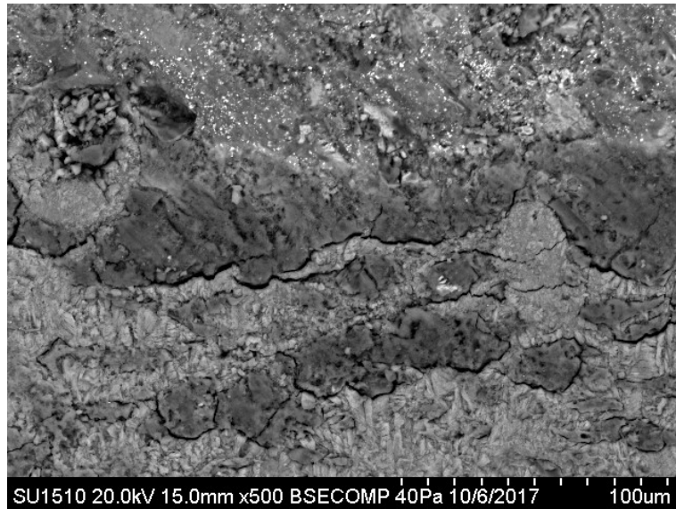
Figure 5-14: SEM image of interface between corroded and non-corroded parts in HMZ coating, Top: non-corroded part, Bottom: corroded part
