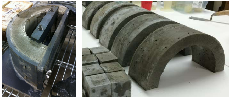
Figure 2-16: Preparation of arch-shaped test specimens
