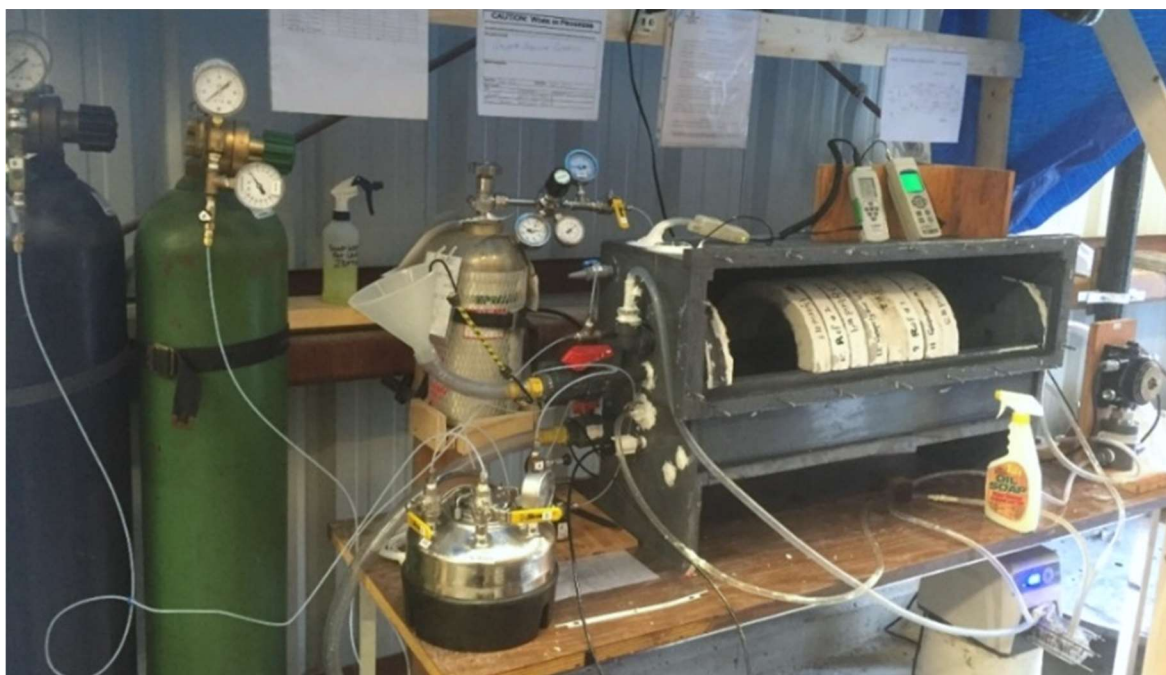
Figure 2-10: Developed chamber for simulating bio-corrosion in the laboratory
