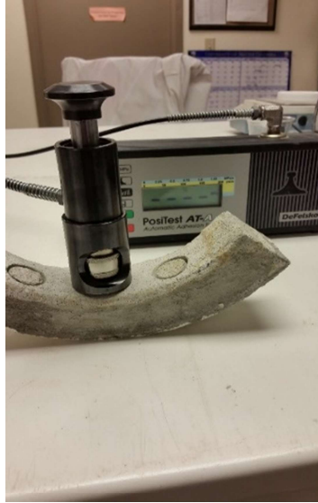
Figure 5-18: Pull-off test set-up
