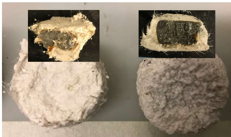
Figure 4-48: CZF samples deteriorated in acidic environment
