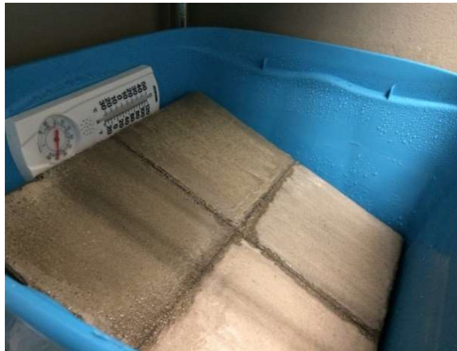
Figure 4-30: Curing of coated samples for the adhesion test
