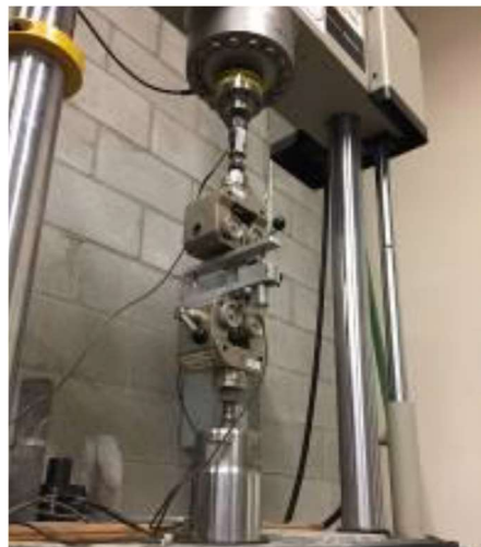
Figure 4-10: Uniaxial tensile test set up
