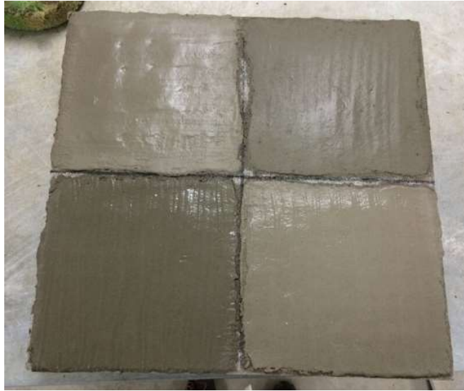
Figure 4-29: Application of the mixes for the adhesion test
