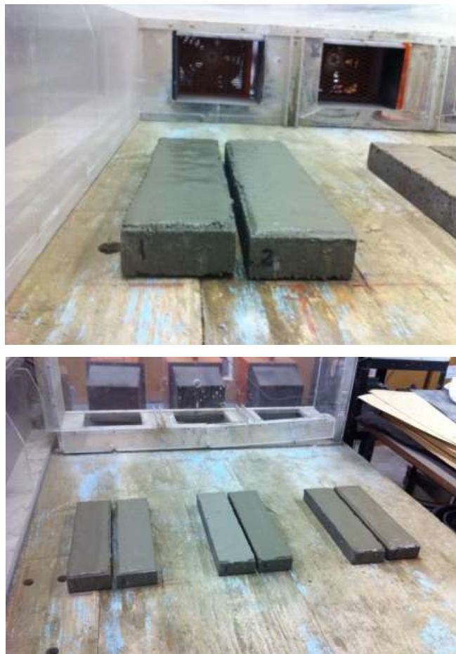
Figure 4-34: Application of coating on shrinkage samples for this experiment
