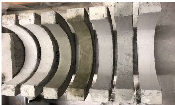
Figure 5-3: Application of different coatings on the surface of arch-shaped samples
