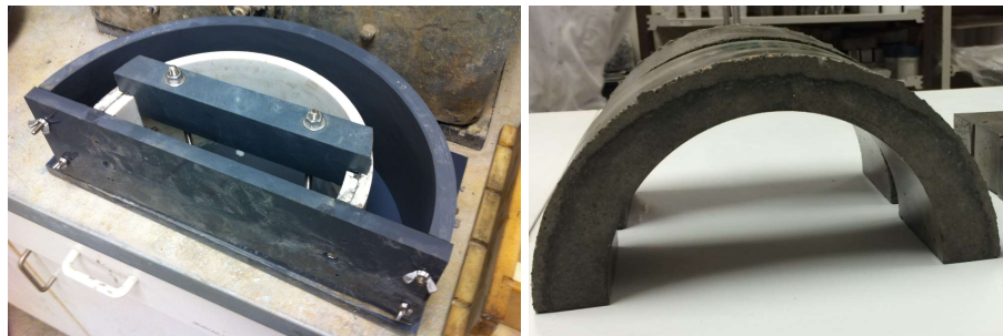
Figure 5-1: Casting arch-shaped mortar base for coatings
