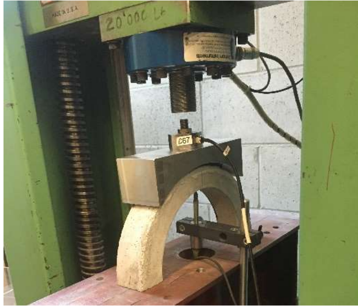
Figure 3-25: Test set-up for measuring flexural strength of the samples after and before corrosion
