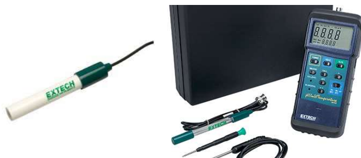
Figure 3-4: Flat surface pH electrode (Extech 601100) used to measure surface pH of the samples
