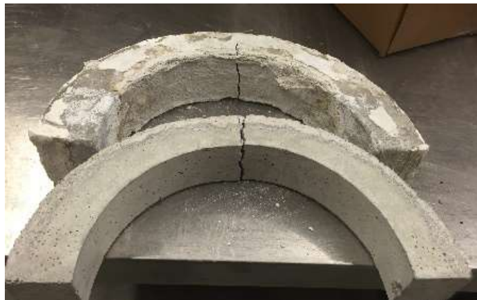
Figure 3-26: Measurements of the effect of corrosion on the ultimate load bearing capacity of the samples
