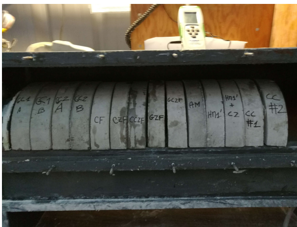
Figure 2-17: Allocating arch-shaped samples (age 28 days) in the accelerated test chamber
