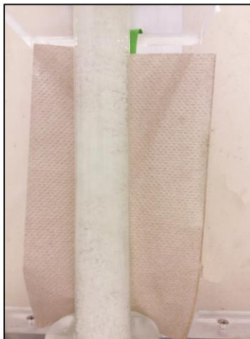
Figure 3.8 Struvite crystal forming in the active zone
