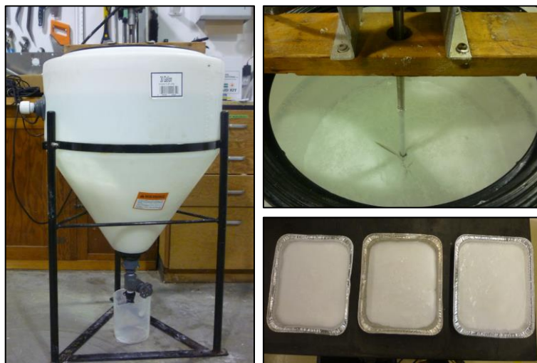
Figure 3.4 Synthetic newberyite preparation tank (left), Settling of synthetic newberyite (top right), Filtered newberyite before drying (bottom right)
