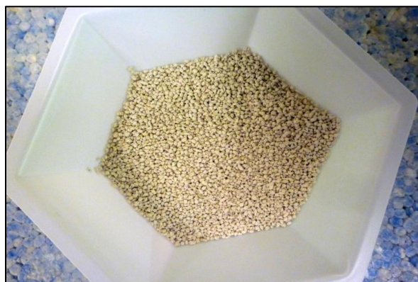
Figure 3.2 Newberyite pellets made by thermally decomposing struvite.
