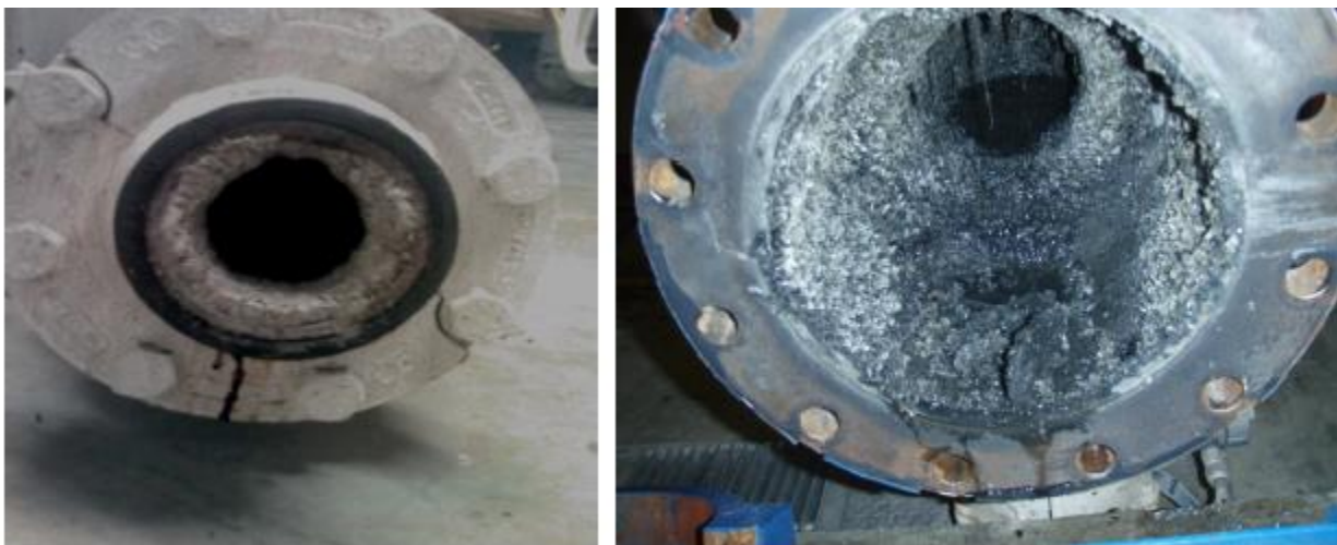
Figure 2.1 Struvite encrustation in a pipe at Lulu Island WWTP (Fattah, 2004)
