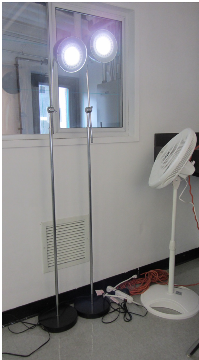
Figure 2.4: Partial view of the south wall inside the test chamber, showing two of the three LED lights, the room fan, and the exhaust vent above the base of the light stand.
