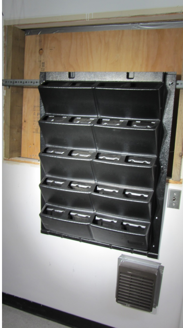
Figure 2.5: Partial view of the north wall inside the test chamber, along with an empty Modulogreen panel. The ventilation fan is located near the base of the wall.
