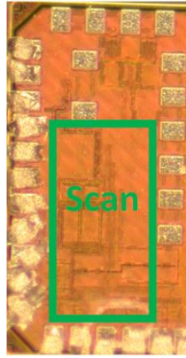
Figure 4.5 Die photo of the standalone scan chain and custom-made pads to reduce area and parasitics.
