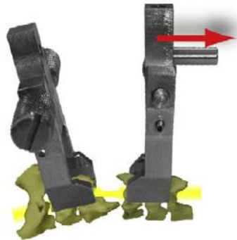
Figure 1-38 - A distraction injury produced by the UBC multi-mechanism injury device, where the rostral vertebral clamp was rigidly secured at 15 degrees flexion, and the caudal vertebral clamp was distracted caudally. (reprinted with copyright permission) (Choo et al., 2009)
