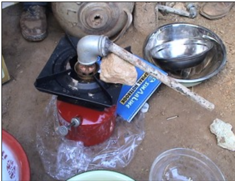
Figure 2.4 Examples of Retorts (Veiga, 2003) 10
