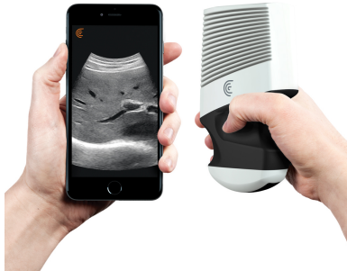
(c) Clarius: a Hand-held Ultrasound Machine Device. (Image Source: www.clarius.me )
