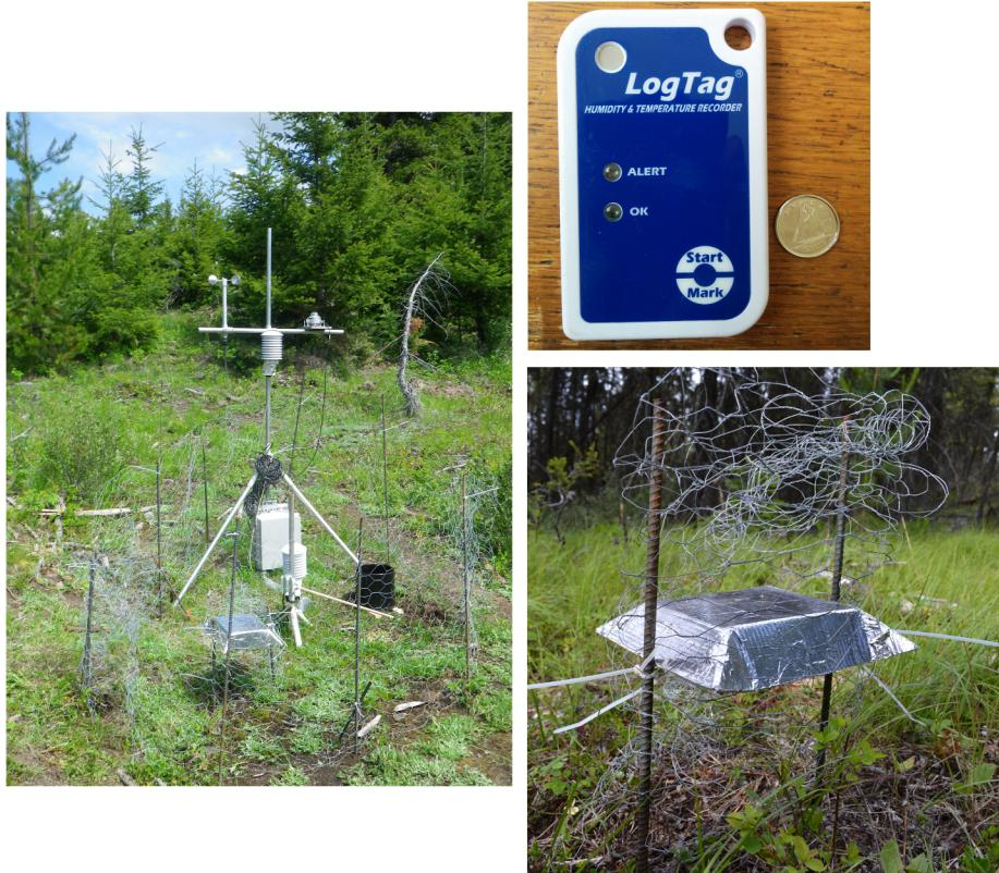
**Figure 2.3:** Field instrumentation. *Left:* Base Station; *Top Right:* LogTag Haxo-8 humidity and temperature sensor; *Bottom Right:* Radiation screen installed at Site 6. Instrumentation was surrounded by chicken wire to protect against grazing cattle.
