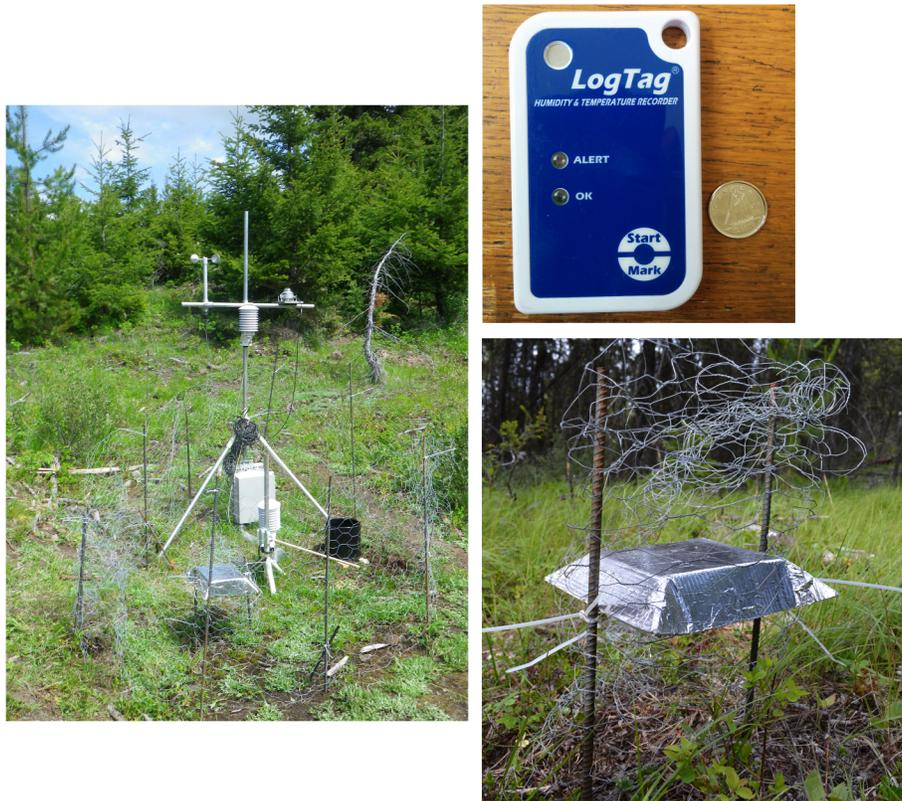
**Figure 2.3:** Field instrumentation. *Left:* Base Station; *Top Right:* LogTag Haxo-8 humidity and temperature sensor; *Bottom Right:* Radiation screen installed at Site 6. Instrumentation was surrounded by chicken wire to protect against grazing cattle.
