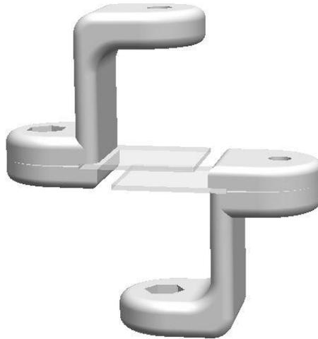
**Figure 2-4 – 3D Printed Electrode Holders** – 3D CAD drawings of holders designed using SolidWorks. Omitted from these drawings include hardware, specifically wingnuts and bolts for clamping the electrodes and connecting to the tensiometer.
