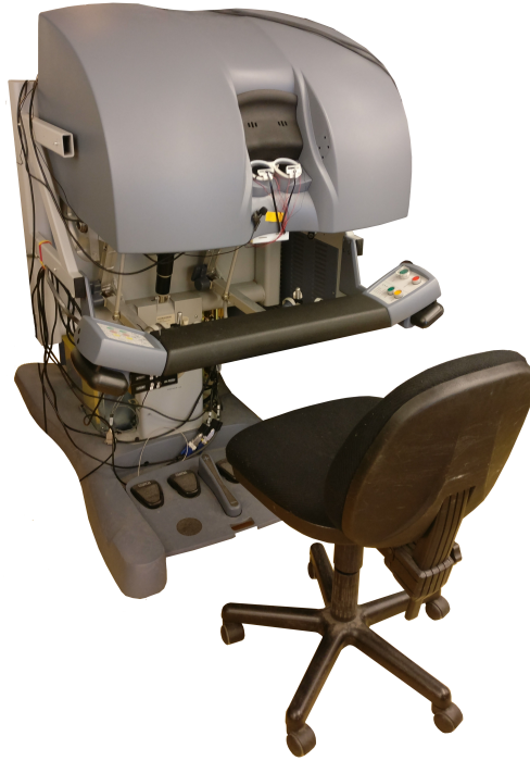
Figure 4.1: Surgeon console with retro-fit eye gaze tracker
