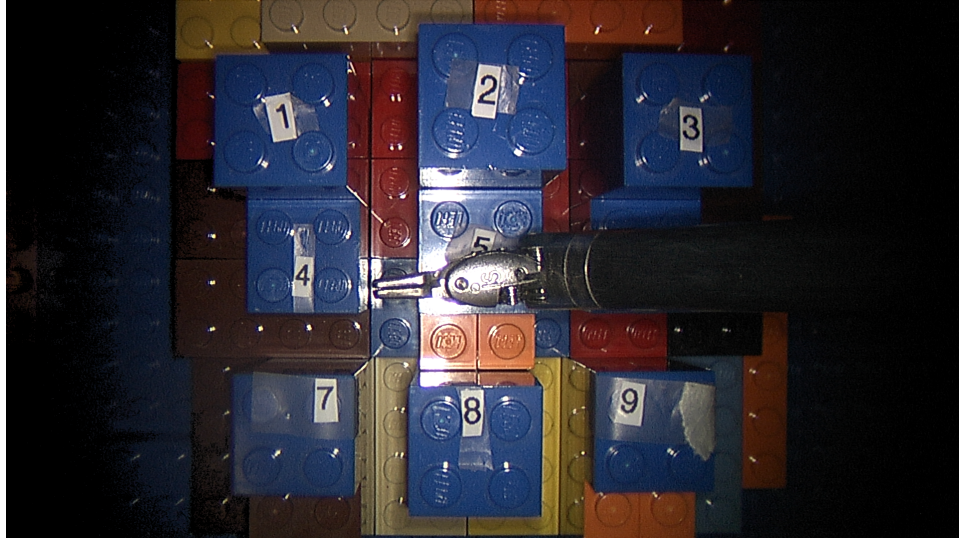
Figure 4.8: 3D accuracy evaluation view within da Vinci surgeon console.
