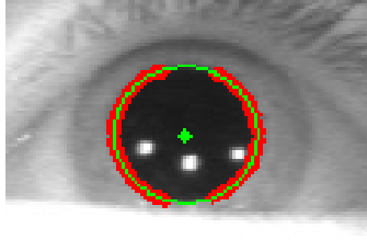
Figure 3.21: Outcome of RANSAC algorithm, with pupil center shown as green point and detected contour shown as green circle.
