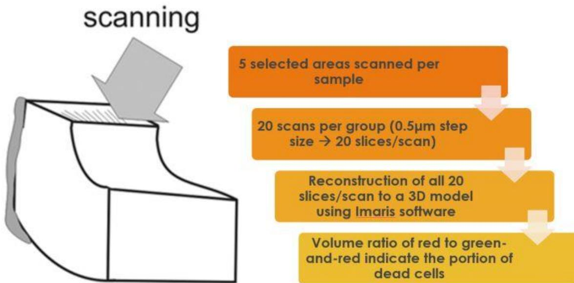
**Figure 9 Description of the CLSM procedure (83)**
