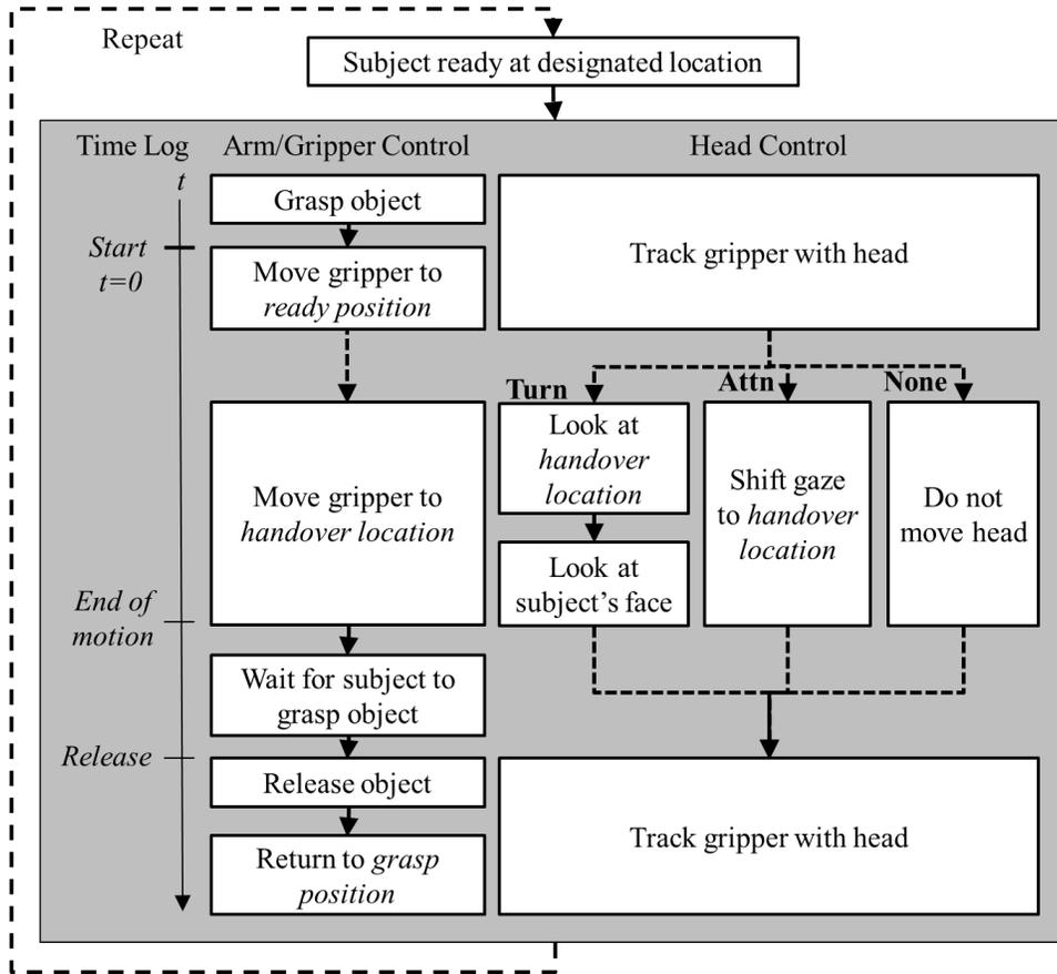
**Figure 3.5:** Experiment system flow diagram. (©2014 IEEE/ACM)
