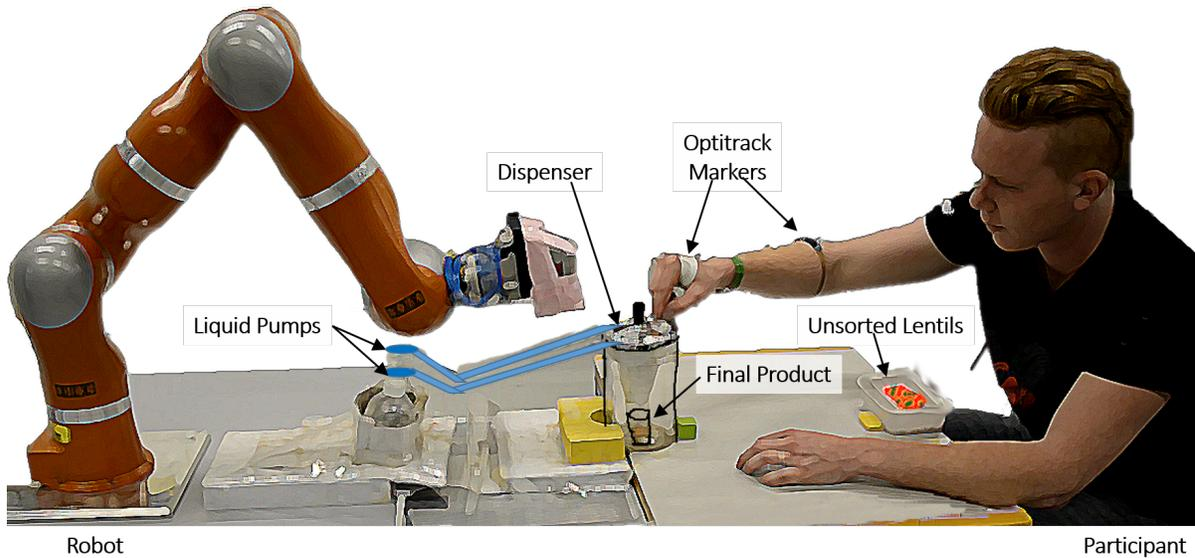
**Figure 5.1:** Experiment set-up of Study 5. The robot and a participant sat facing each other with a dispenser mechanism located on the table between them. The shared use of the dispenser allowed spontaneous HR resource conflicts to occur throughout the experiment.
