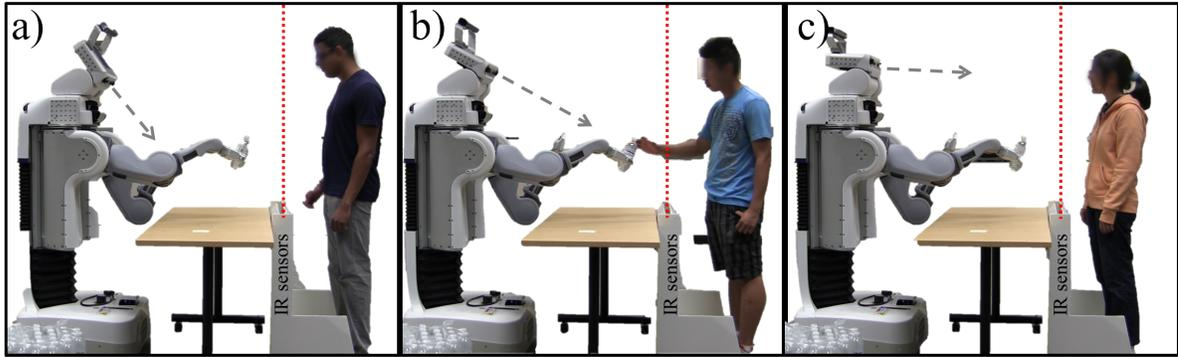
**Figure 3.3:** Demonstration of the experimental set-up and the three conditions at the *handover location*: a) No Gaze; b) Shared Attention; and c) Turn-Taking. An array of infrared sensors was located at the edge of the table. The red dotted lines represent the location where subject's reach motion is detected. Subjects stood at a specified location marked on the floor. (©2014 IEEE/ACM)
