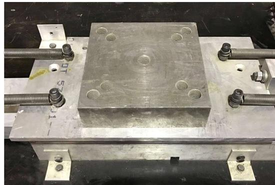
**Figure 2-4 Equivalent mass on the shake table**
