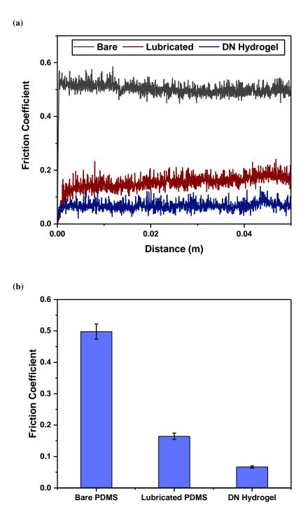
Figure 3.10 (a) Friction coefficient of various substrates and (b) their comparison.
