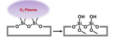
Figure 1.1 Oxygen plasma treatment for PDMS surface.
