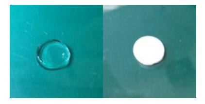
Figure 1.2 SN alginate gel (left) and DN alginate-pHEMA gel (right).
