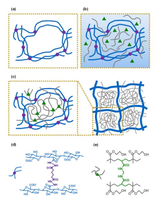
Figure 2.1 Schematics of the two networks of alginate-polyHEMA hydrogel; (a) alginate network, (b) diffusion of HEMA monomers, (c) resulting DN structure, (d) alginate chains covalently crosslinked by AAD (purple circles), (e) HEMA monomers covalently crosslinked by MBAA (green triangles).
