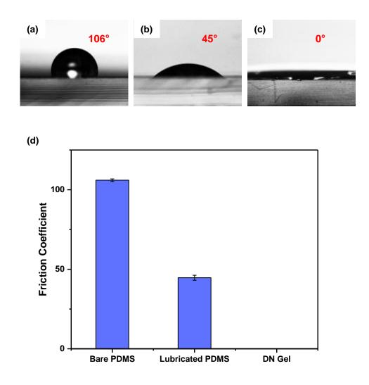
Figure 3.9 Water droplets on (a) bare PDMS, (b) lubricated PDMS and (c) DN hydrogel surface, and (d) the contact angles of water on these surfaces.
