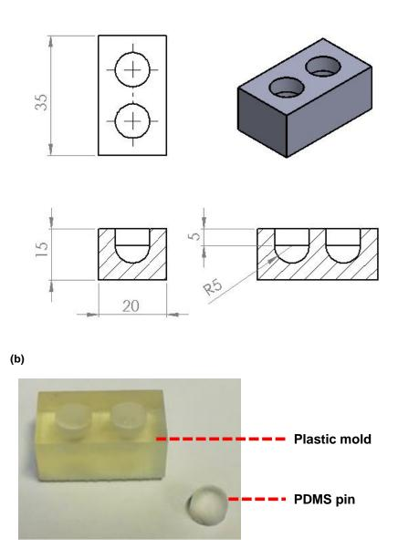
Figure 3.5 (a) The schematic and dimensions of the printed plastic mold for PDMS test pin (unit: mm) and (b) a printed plastic mold and cured PDMS test pin cast from the mold.
