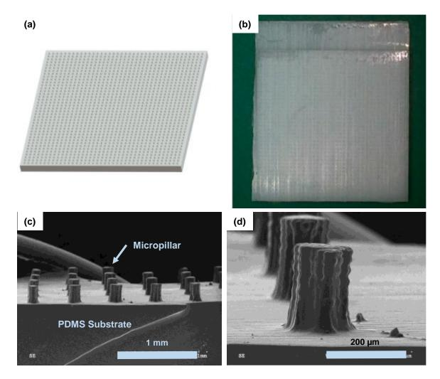
Figure 3.1 (a) Illustration of the CAD model of 20 mm × 20 mm substrate master; (b) The plastic master printed by Asiga Pico printer; (c) SEM image of micropillar substrate; and (d) close-up of a single micropillar.
