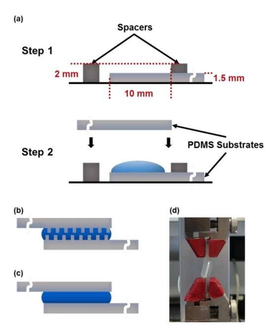
Figure 3.6 (a) Fabrication process for the lap-shear test strips, (b) the cross-section view of test ribbon with micropillars, (c) the cross-section view of test ribbon without micropillars, and (d)
