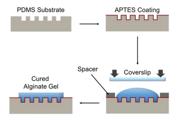
Figure 3.3 DN hydrogel coating procedures.
