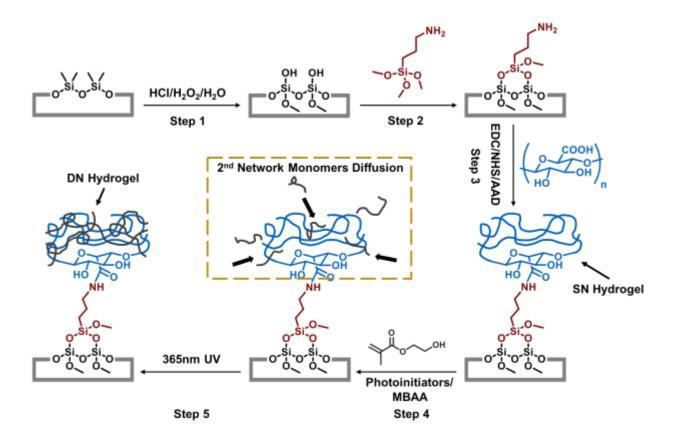
Figure 3.2 Chemical modification on PDMS substrate and DN hydrogel coating formation.
