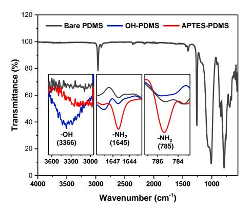
Figure 3.7 FT-IR spectroscopy of bare PDMS, OH-PDMS and APTES-PDMS.
