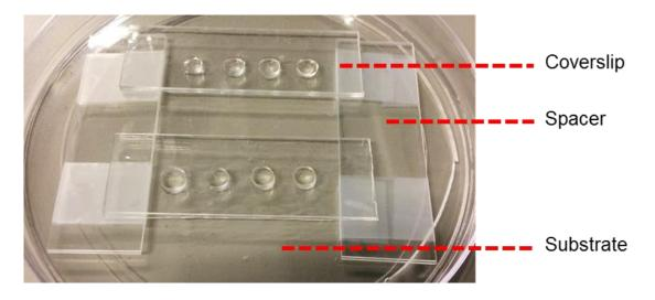
Figure 2.2 Fabrication setup for SN alginate hydrogel dishes.
