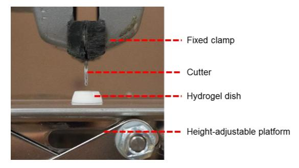
Figure 2.3 Setup for hydrogel slicing experiment.
