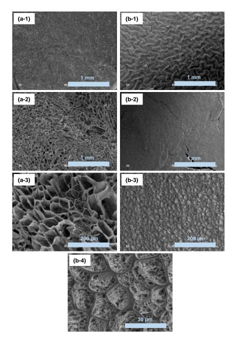
Figure 2.9 (a) SN alginate hydrogel and (b) DN alginate-pHEMA hydrogel; (1) 50× magnification on the surface, (2) 50× magnification on the cross-section, (3) 250× magnification on the cross-section, and (4) 1500× magnification on the cross-section.
