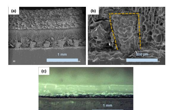
Figure 3.4 SEM and OM images of the cross-sections of DN gel coating on micropillar
