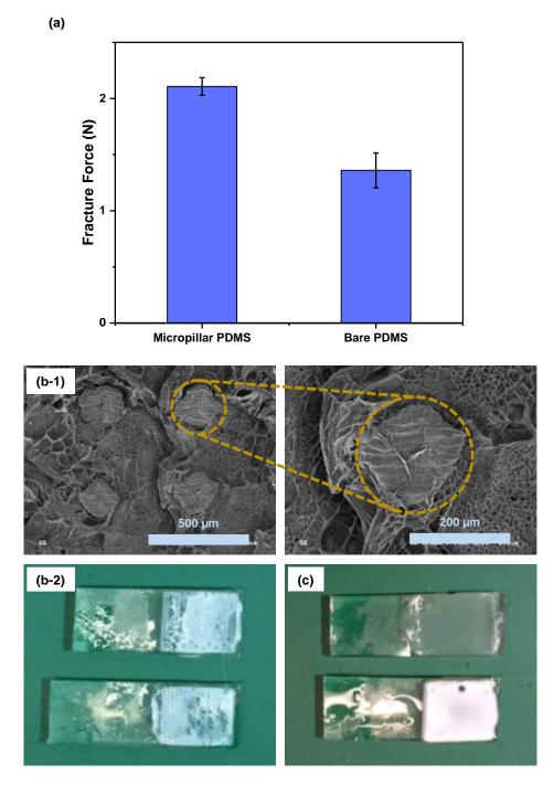
Figure 3.8 (a) Maximal force to separate the bonded strips, (b) separated micropillar strips and (c) separated bare PDMS strips.
