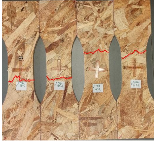
(a) Tested OSB Specimens (Diagonal (D45 0 ) direction)
