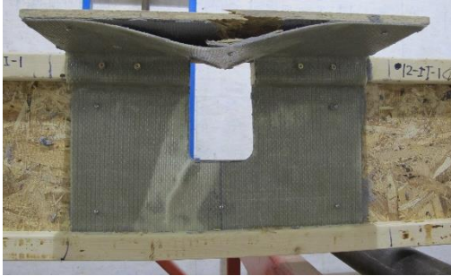
(a) Flange Notch Failure:Type-T1
