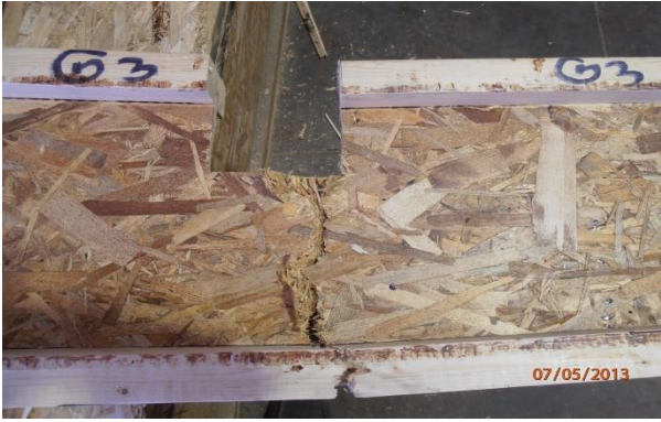
(a) Pure flexural failure: 12 feet I-joists
