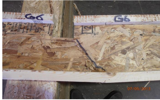
(b) Combined flexural and shear failure: 12 feet I-joists
