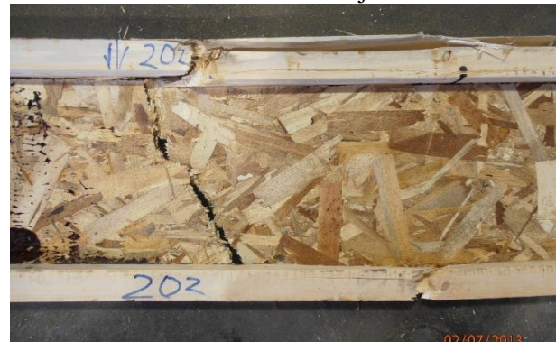
(d) Combined flexural and shear failure: Retrofitted 20 feet I-joists
