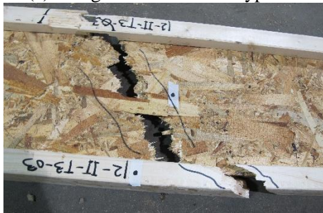
(e) Flange Notch Failure:Type-T3
