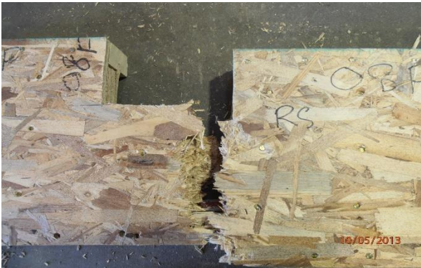
(a) Pure flexural failure: Retrofitted 12 feet I-joists
