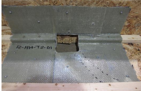
(a) Flange Notch Failure:Type-T1
