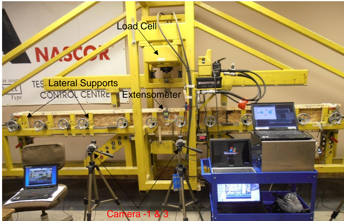
Figure 3.2: Testing Frame used to perform four points bending test of I-Joists (With a 12 ft Control I-Joist).
