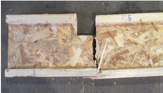
(c) Pure flexural failure: 20 feet I-joists
