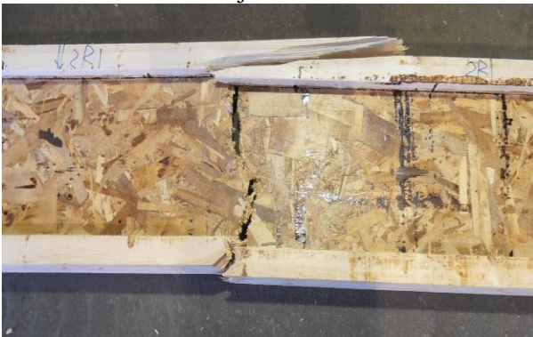
(c) Pure flexural failure: Retrofitted 20 feet I-joists
