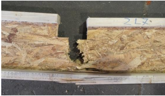
(a) Crack occurred at the middle of the notch width instead of the corner.
