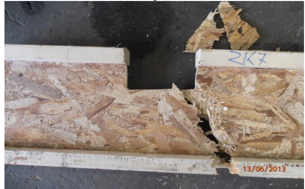
(d) Combined flexural and shear failure: 20 feet I-joists
