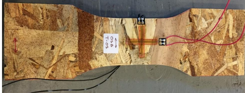
Figure 3.4 Sample of a OSB Tension test specimen with a Bi-axial Strain Gauge
