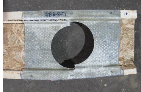
(b) Web Hole Failure:Type-T1
