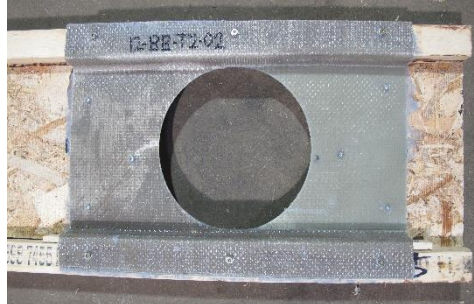
(b) Web Hole Failure:Type-T1
