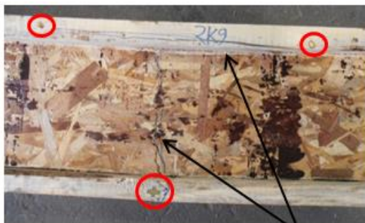
Figure 4.5: Failure mechanisms exhibited in tested I-joists with flange notch (Series: 12-F, 12-G, 12-H, 12-I, 20-K, 20-L, 20-M, and 20-N)
