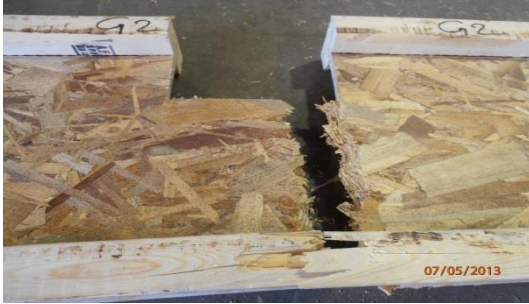
(a) Pure flexural failure: 12 feet I-joists
