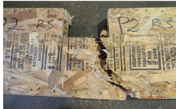
(b) Combined flexural and shear failure: Retrofitted 12 feet I-joists
