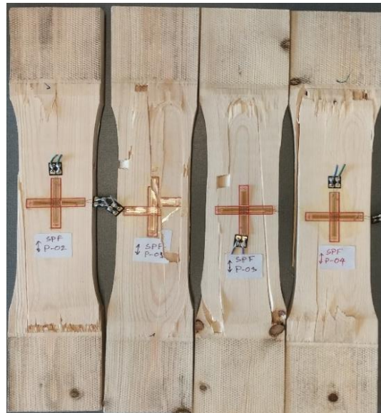
Figure 3.8 Details of Timber coupon specimen for tension test.
