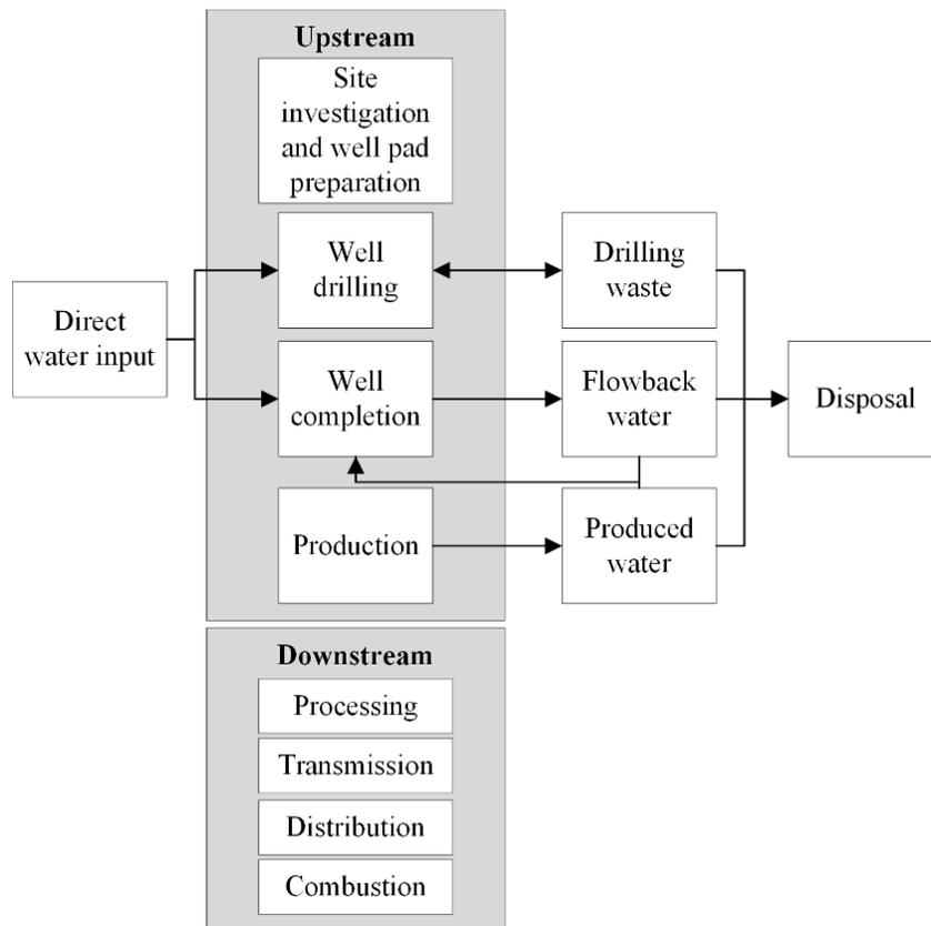
Figure 2.3 Direct water input in the upstream unconventional well life cycle
