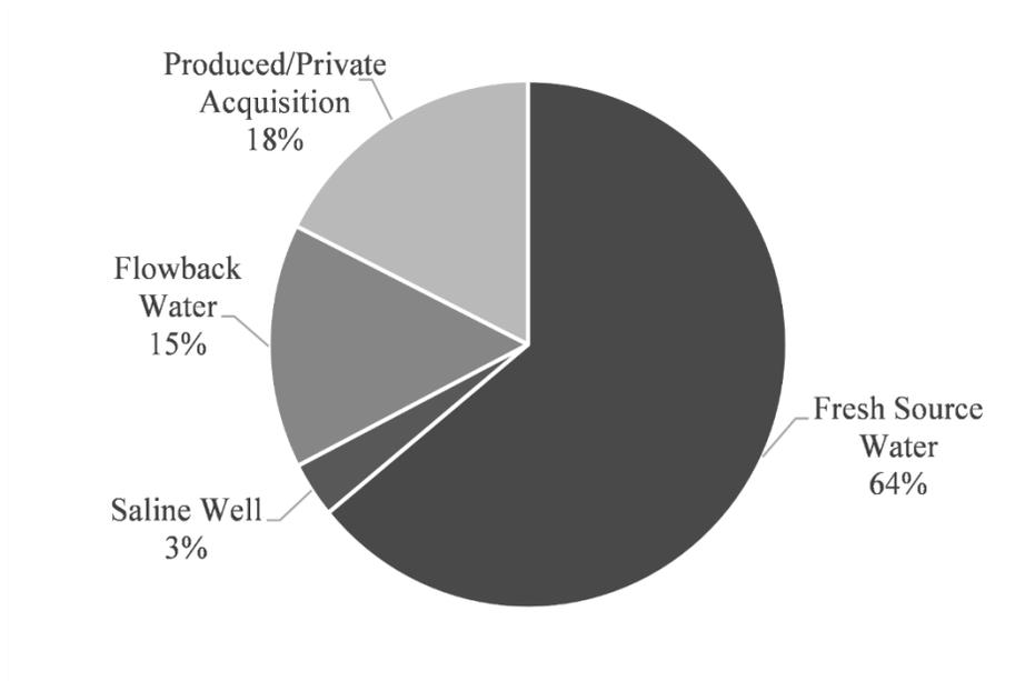
Figure A.3 Water sources of BC fracturing fluid<sup>20</sup>
