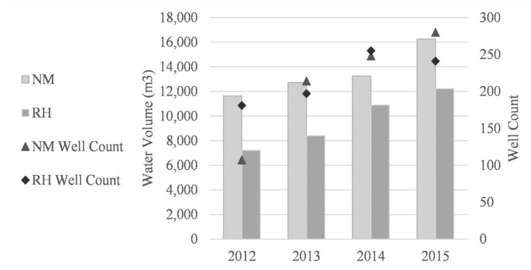
Figure A.1 Average hydraulic fracturing water demand (m<sup>3</sup>/well) and well counts
