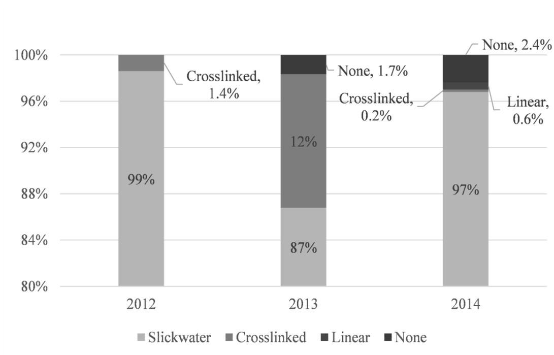
Figure A.5 Percentage of fluid treatment type by fracture stage
