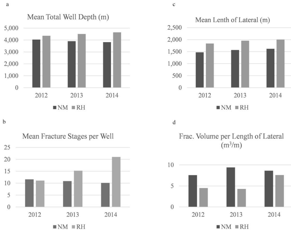
Figure A.2 Well characteristics by year for NM and RH wells (2012-2014)
