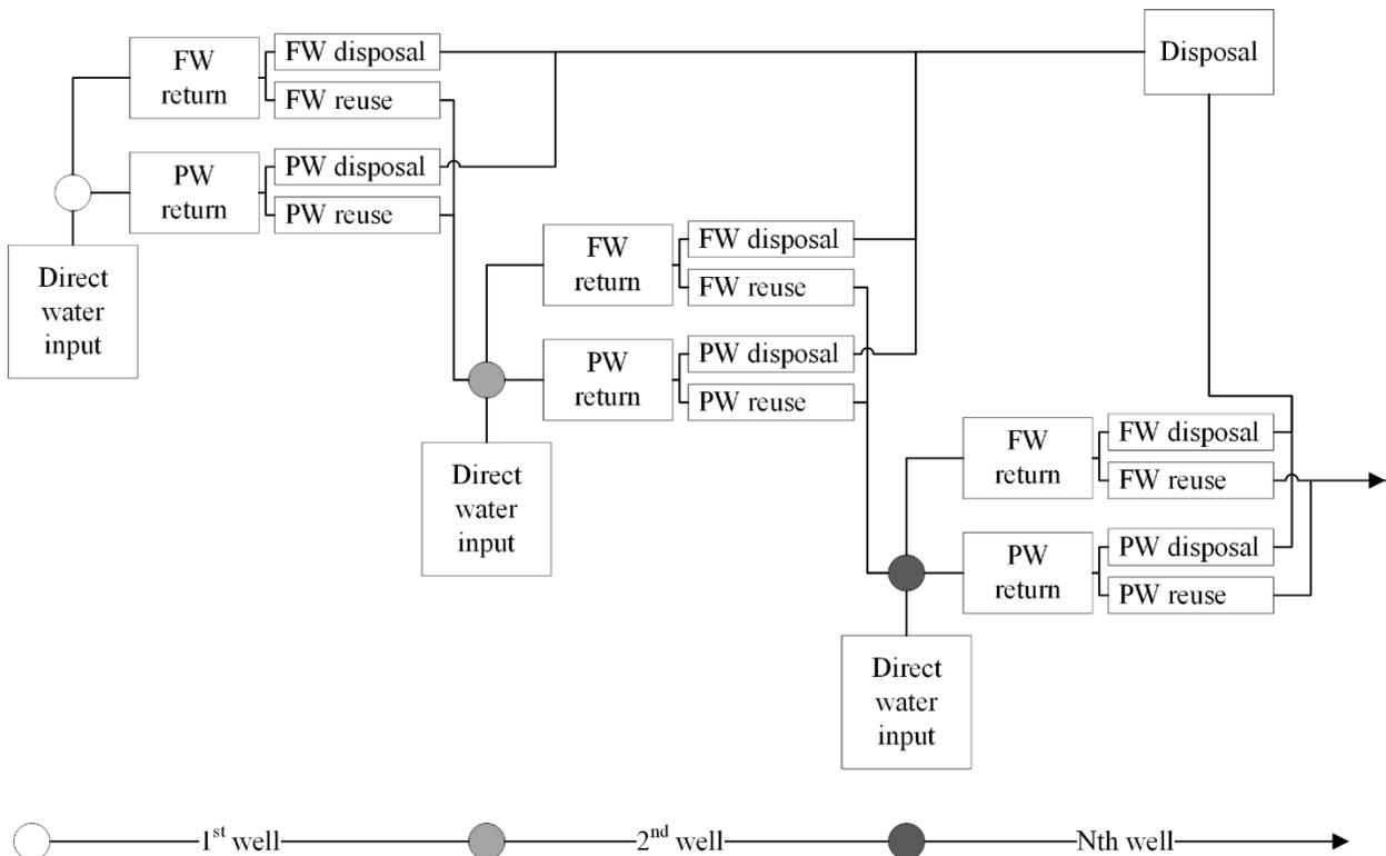
Figure 2.4 Direct water use, flowback, and produced water reuse cycle in UUOGA
