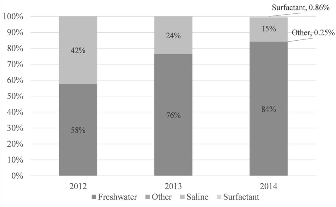
Figure A.4 Percentage of fracture stages completed by base fluid
