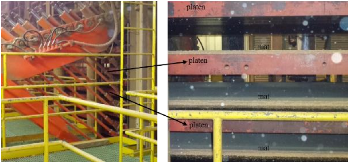
Figure 1.14: Daylight press with multiple openings for hot pressing mats. Source: Sam-Brew 2016.
