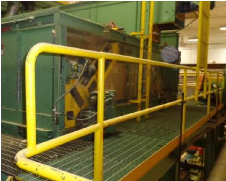
Figure 1.9: Forming bin with resinated face furnish. Source: Sam-Brew 2016.
