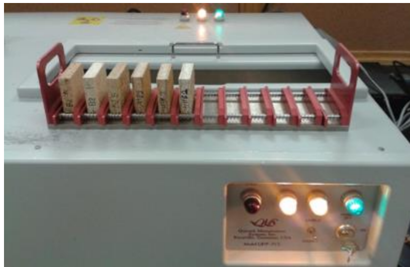
Figure 2.17: X-ray machine for vertical density gradient measurements. Source: Sam-Brew 2016.
