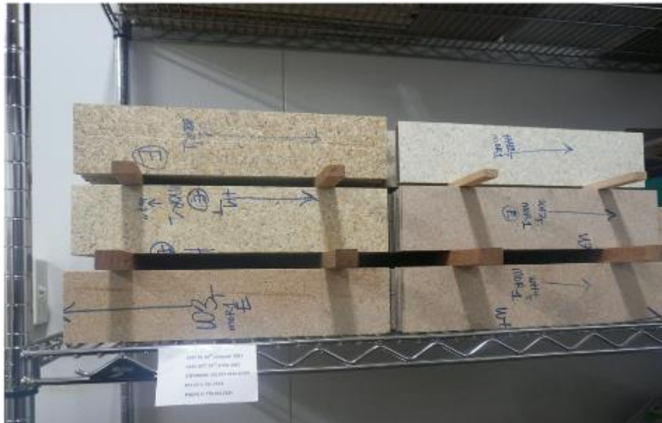
Figure 2.16: Test samples stacked in a constant humidity chamber. Source: Sam-Brew 2016.
