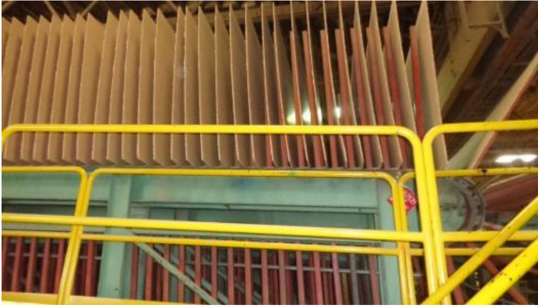
Figure 1.16: Cooling wicket for manufactured particleboard. Source: Sam-Brew 2016.
