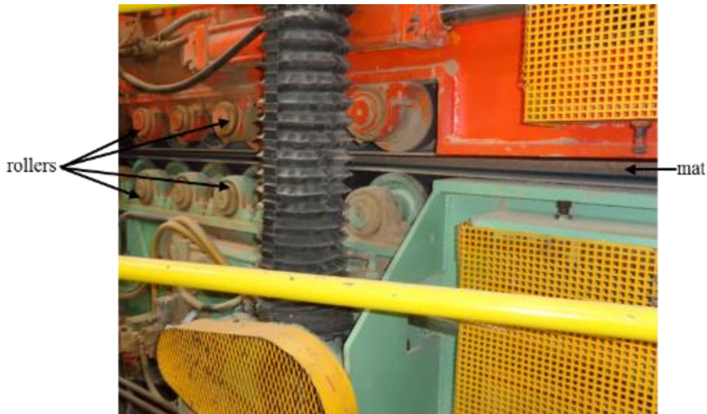
Figure 1.13: Prep-pressing of formed mat using a system of rollers. Source: Sam-Brew 2016.
