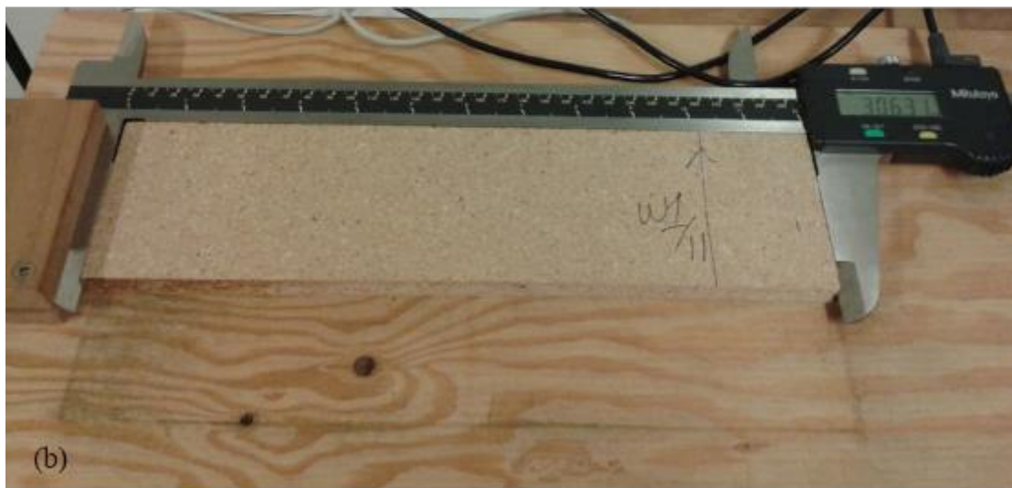
Figure 2.20: Linear expansion measurements for wood particleboard measured a) parallel and b) perpendicular to the forming direction of the board. Arrow indicates the forming direction of the original board. Source: Sam-Brew 2016.
