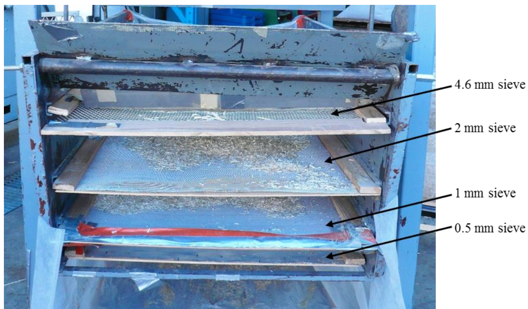
Figure 2.2: Mechanical shaker with 4 sieves for residue fractioning. Source: Sam-Brew 2016.
