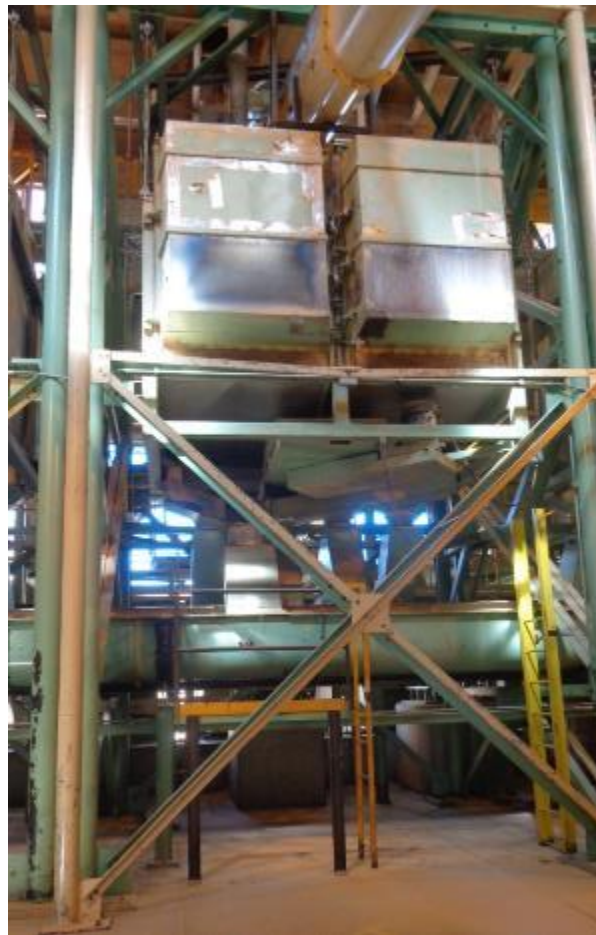
Figure 1.4: Overhead classifying bins for screening residue into face and core material. Source: Sam-Brew 2016.
