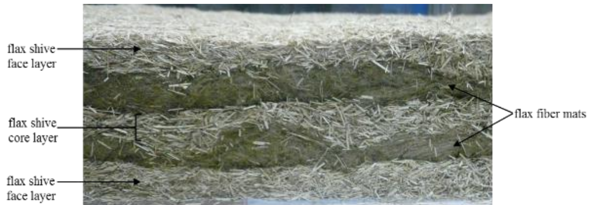
Figure 6.2: Three-layered particleboard mat comprising of flax shive residues and flax fiber. Source: Sam-Brew 2015.
