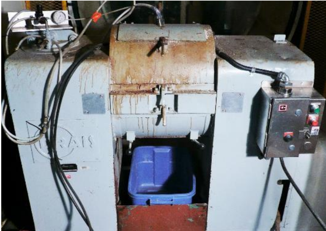
Figure 2.12: Drais paddle-type particleboard blender. Source: Sam-Brew 2016.
