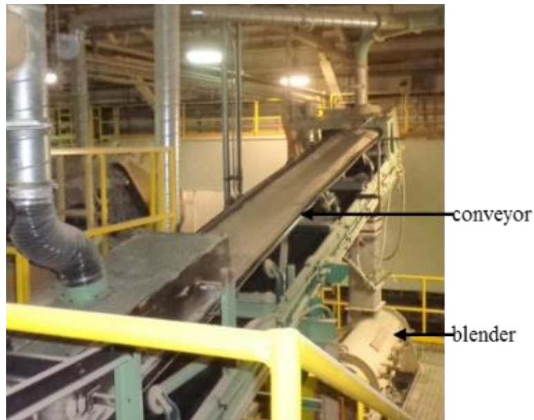
Figure 1.6: Furnish being transported into blender. Source: Sam-Brew 2016.
