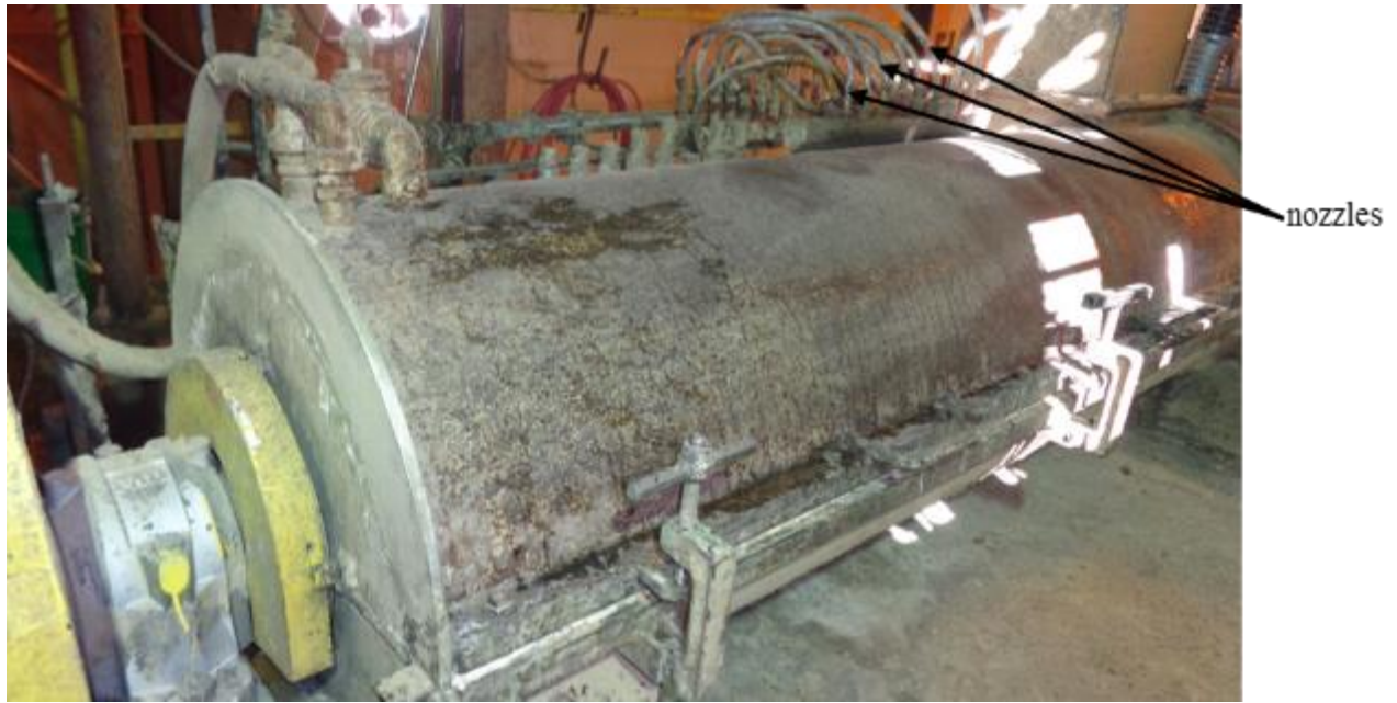
Figure 1.7: Batch blender with several hoses/nozzles for spraying resin and additives. Source: Sam-Brew 2016.
