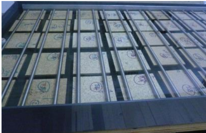
Figure 2.21: Submerged particleboards in thickness swell and water absorption measurements. Source: Sam-Brew 2016.
