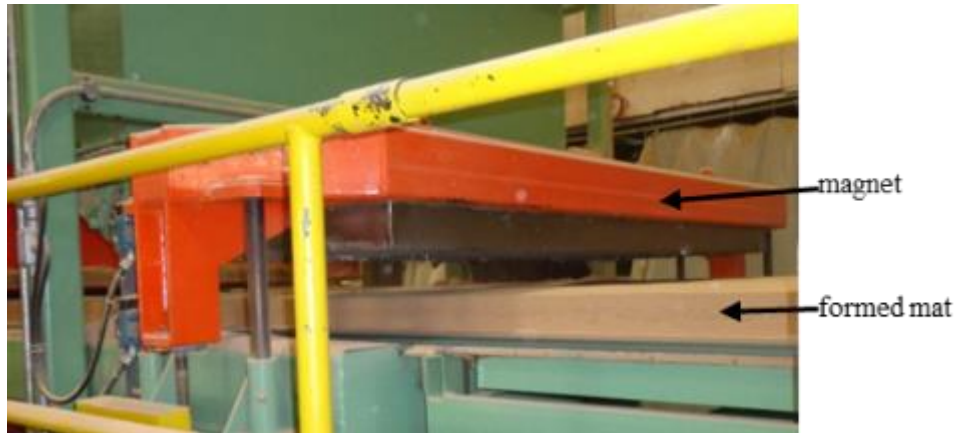
Figure 1.12: Magnet located above formed mat to remove ferro-magnetic objects. Source: Sam-Brew 2016.
