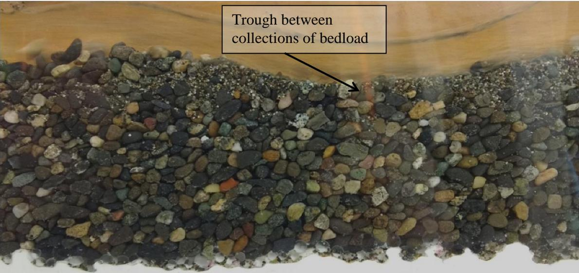
**Figure 5.7** Image from the SLR camera of a trough forming during the SFU<sub>nat</sub> Experiment S.17 ( $D_f=0.6$  mm, fine feed/total feed = 42 %). Flow from left to right.
