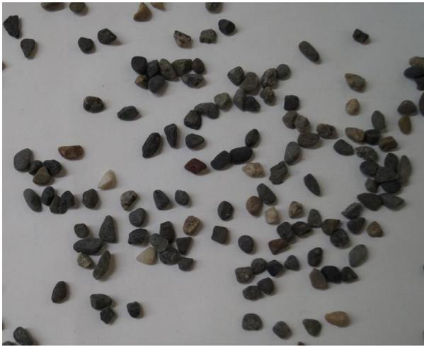
**Figure 5.1** Photograph of the natural 4 mm diameter sediment.
