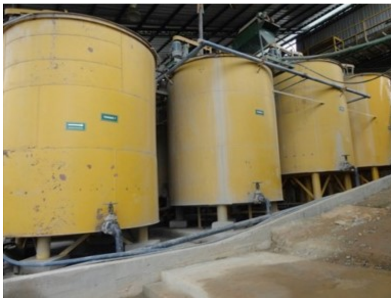
Figure 5.11. Cyanidation with agitated tanks at a processing center in Portovelo-Zaruma. Photo by A. Gonçalves, 2015.
