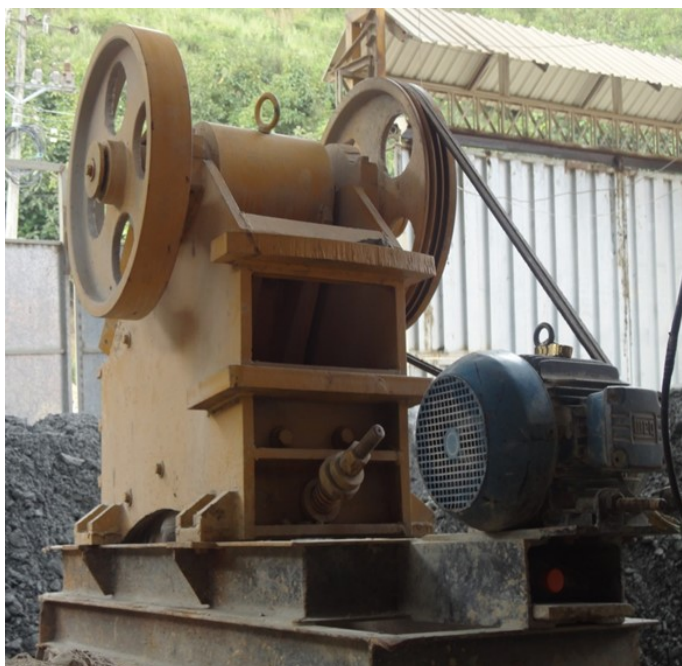
Figure 5.2. Jaw Crusher used by processing centers in Portovelo-Zaruma. Photo by A. Gonçalves, 2015.
