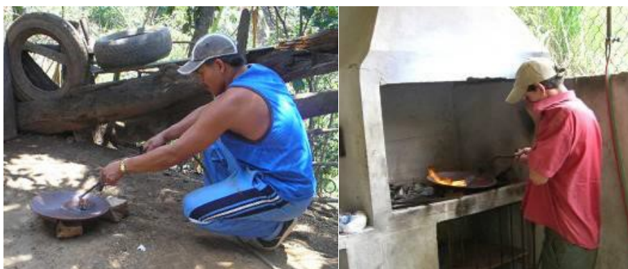
Figure 5.9. Miners burning amalgams in the open air, releasing atmospheric mercury emissions. (Used with permission by Velásquez-López).
