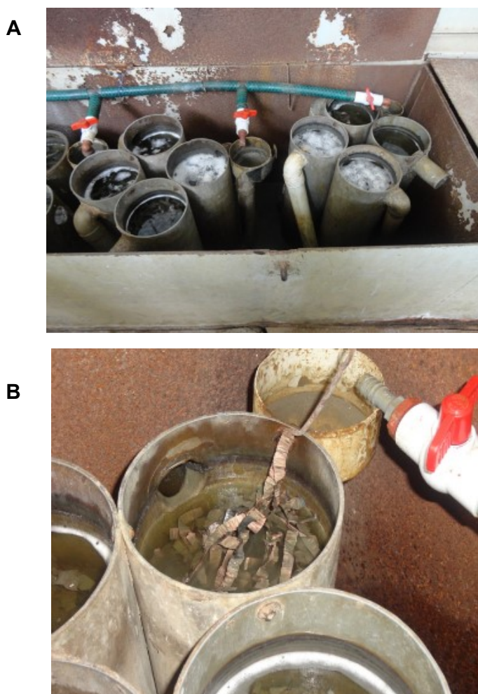
Figure 5.15. A and B. Zinc shavings full of gold during the Merrill-Crowe process at a processing center in Portovelo-Zaruma. Photo by A. Gonçalves, 2015.
