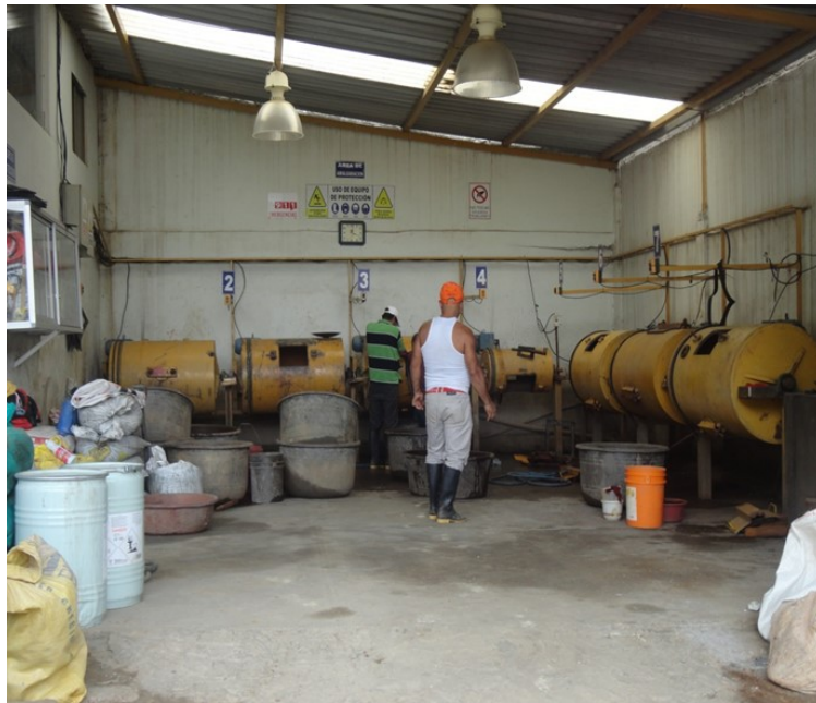
Figure 5.6. Chanchas used in processing centers in Portovelo-Zaruma. Photo by A. Gonçalves, 2015.
