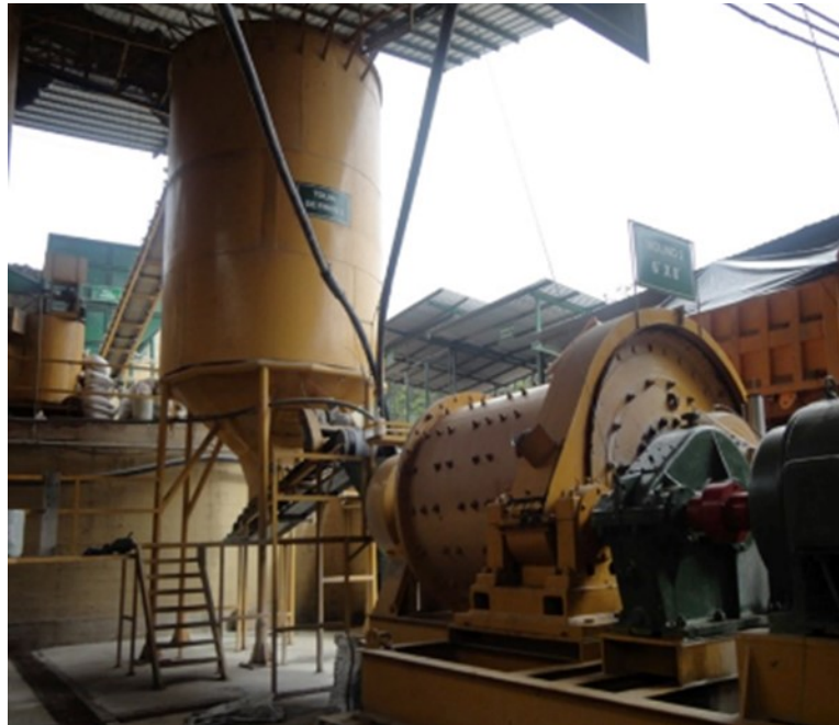
Figure 5.4. Ball mill used in the processing centers in Portovelo-Zaruma. Photo by A. Gonçalves, 2015.
