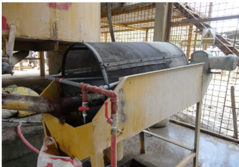
Figure 5.12. Rotating screen drum used in the CIP process in Portovelo-Zaruma. Photo by A. Gonçalves, 2015.
