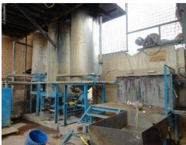
Figure 5.14. Electrowinning circuit at a processing center in Portovelo-Zaruma. Photo by A. Gonçalves, 2015.
