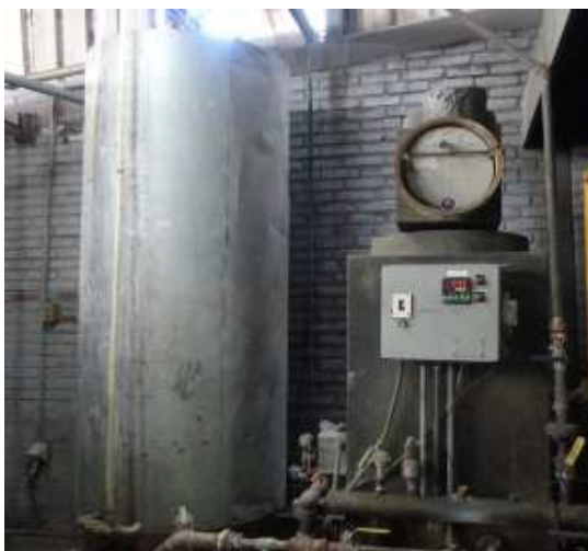
Figure 5.13. Desorption circuit at a processing center in Portovelo-Zaruma. Photo by A. Gonçalves, 2015.
