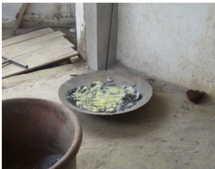
Figure 5.17. Borax used for smelting the gold. Photo by A. Gonçalves, 2015.
