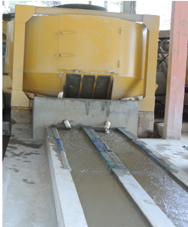
Figure 5.5. Chilean Mill with sluice boxes covered with wool carpets, used in processing centers in Portovelo-Zaruma. Photo by A. Gonçalves, 2015.
