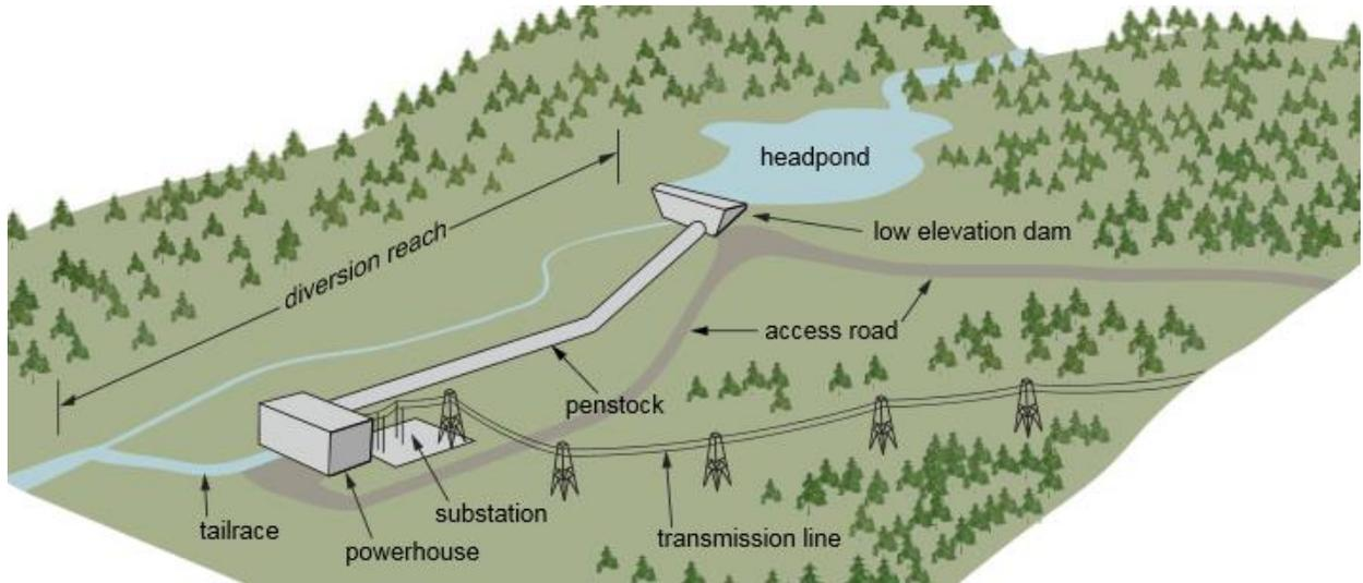
Figure 2-1. A generalized schematic of a run-of-river (RoR) hydropower project (from Gower et al. 2012). A small weir is installed in the river creating a small headpond which raises water levels to allow water to enter the penstock.
